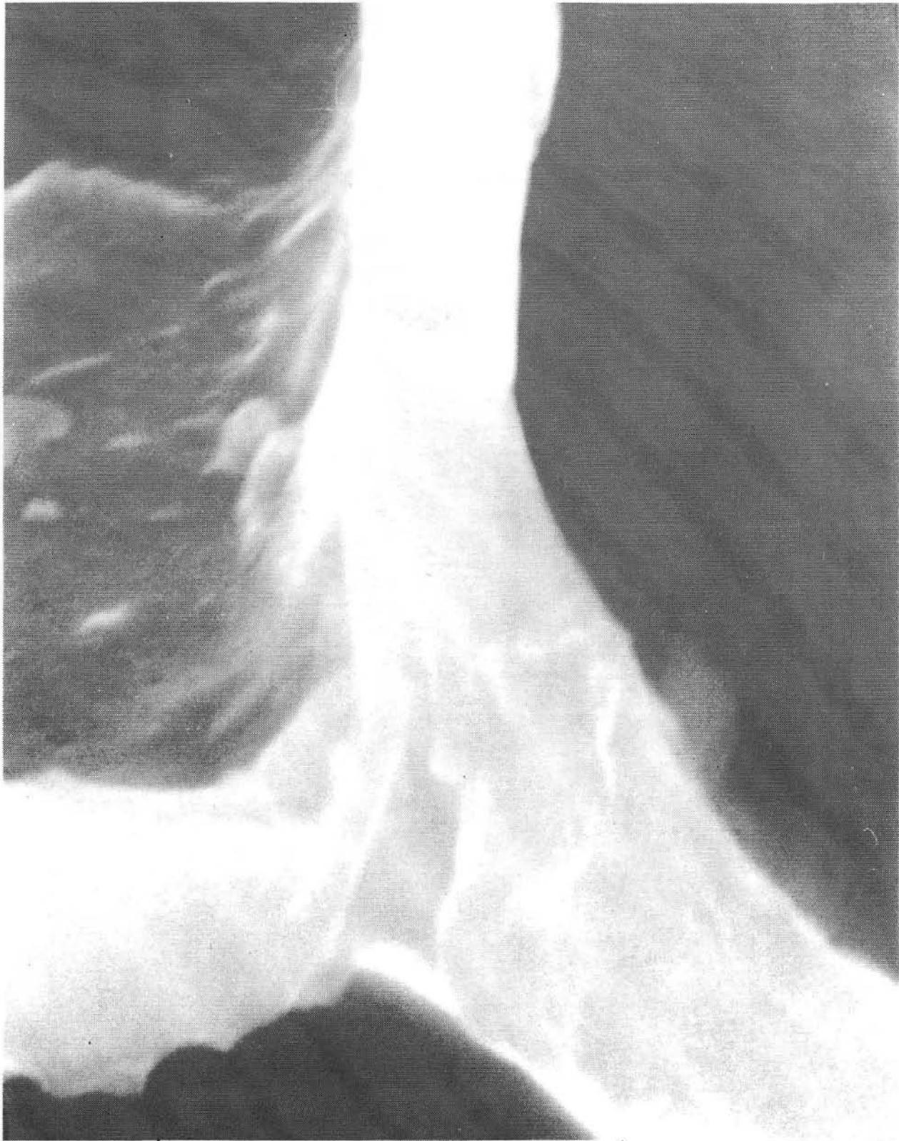
Figure 14. Typical junction of carbonized TKD cell walls.
