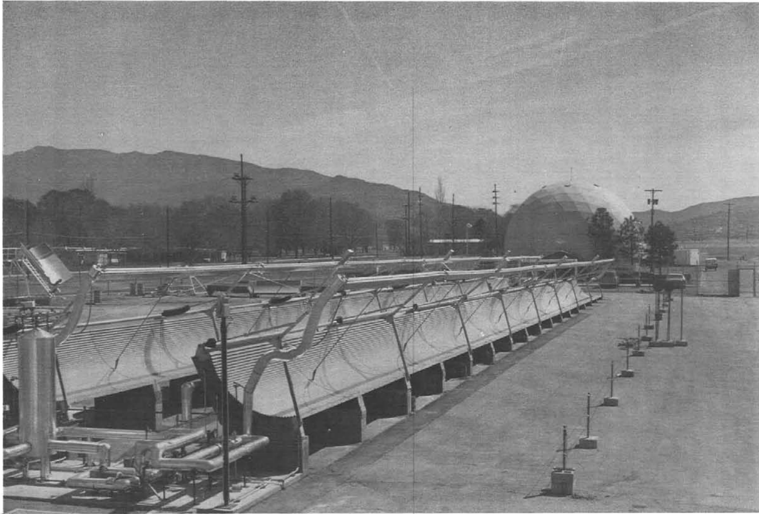
Fig. 1-1. The FMSC collector subsystem installed at Sandia Laboratories' solar total energy test facility
