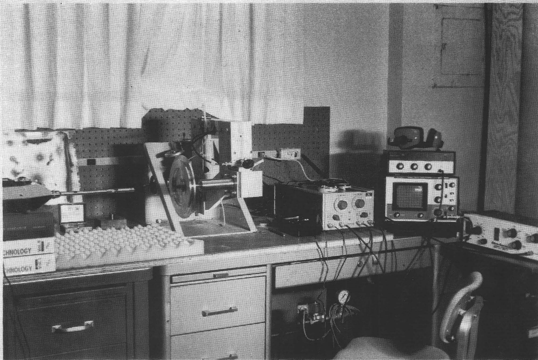
Figure 5-36. Test Setup for Ultrasonic Transducer Sound Level and Frequency Measurements
