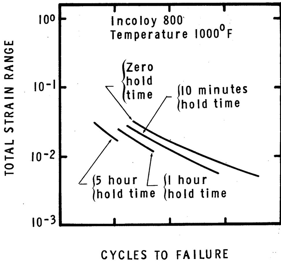
Figure 10. Tensile hold time effects in fatigue, after Majumdar. (19)
