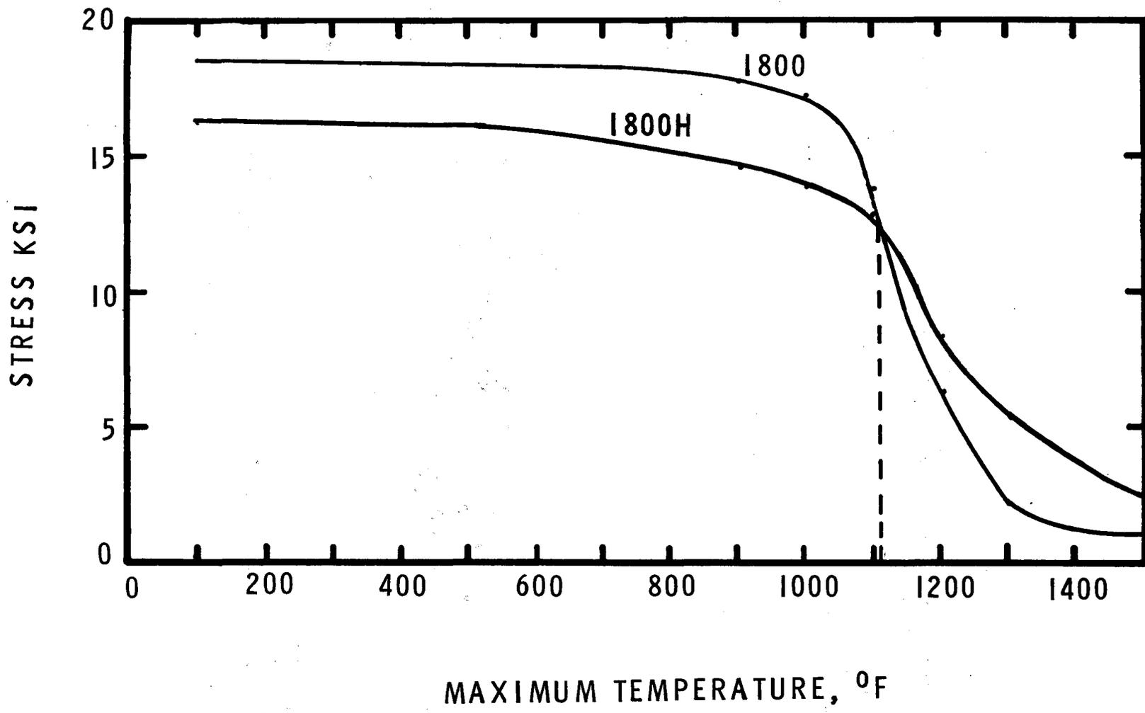
Figure 7. Stress allowable as function of temperature for alloy 800 according to Section VIII of the ASME Boiler and Pressure Vessel Code.
