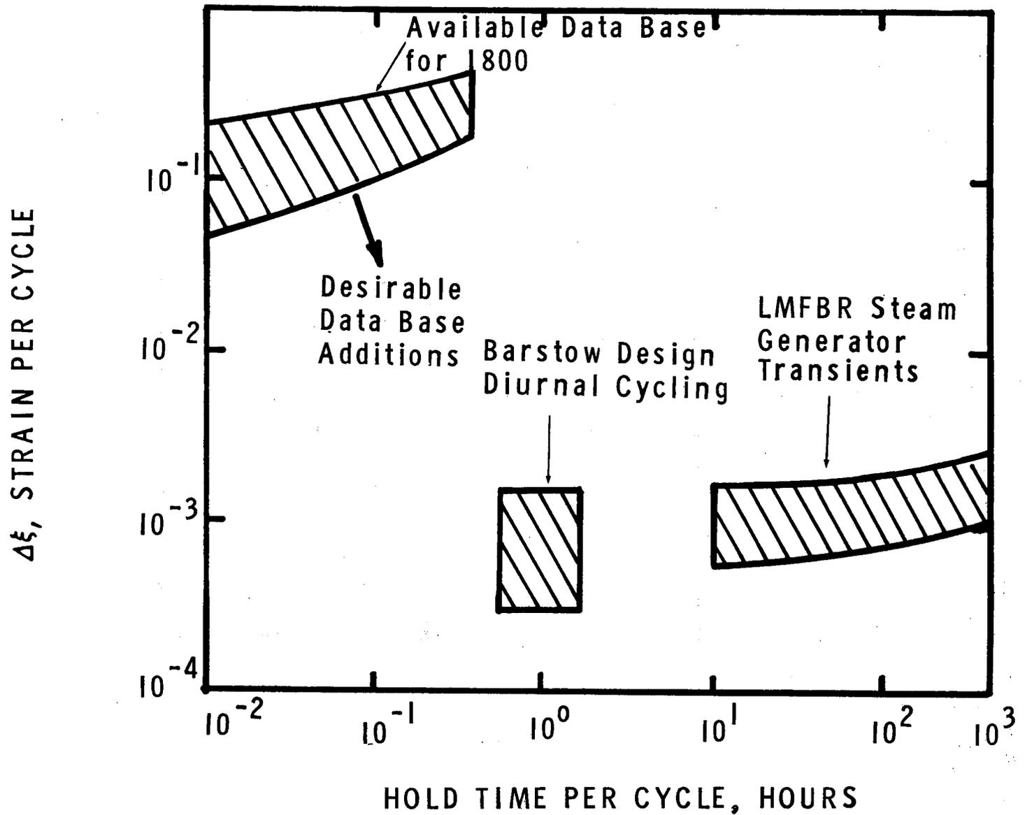
Figure 9. Overview of diurnal fatigue problem in Solar Central Receiver Pilot Plant.
