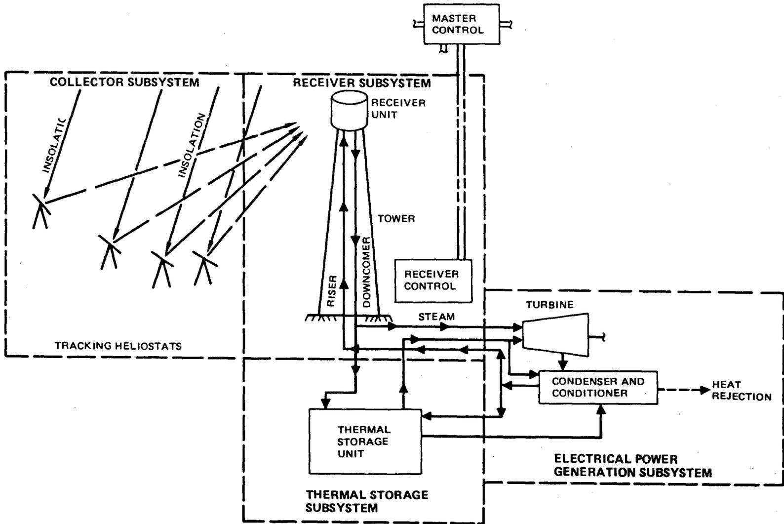
Figure 2. Subsystem description of the pilot plant. (2)
