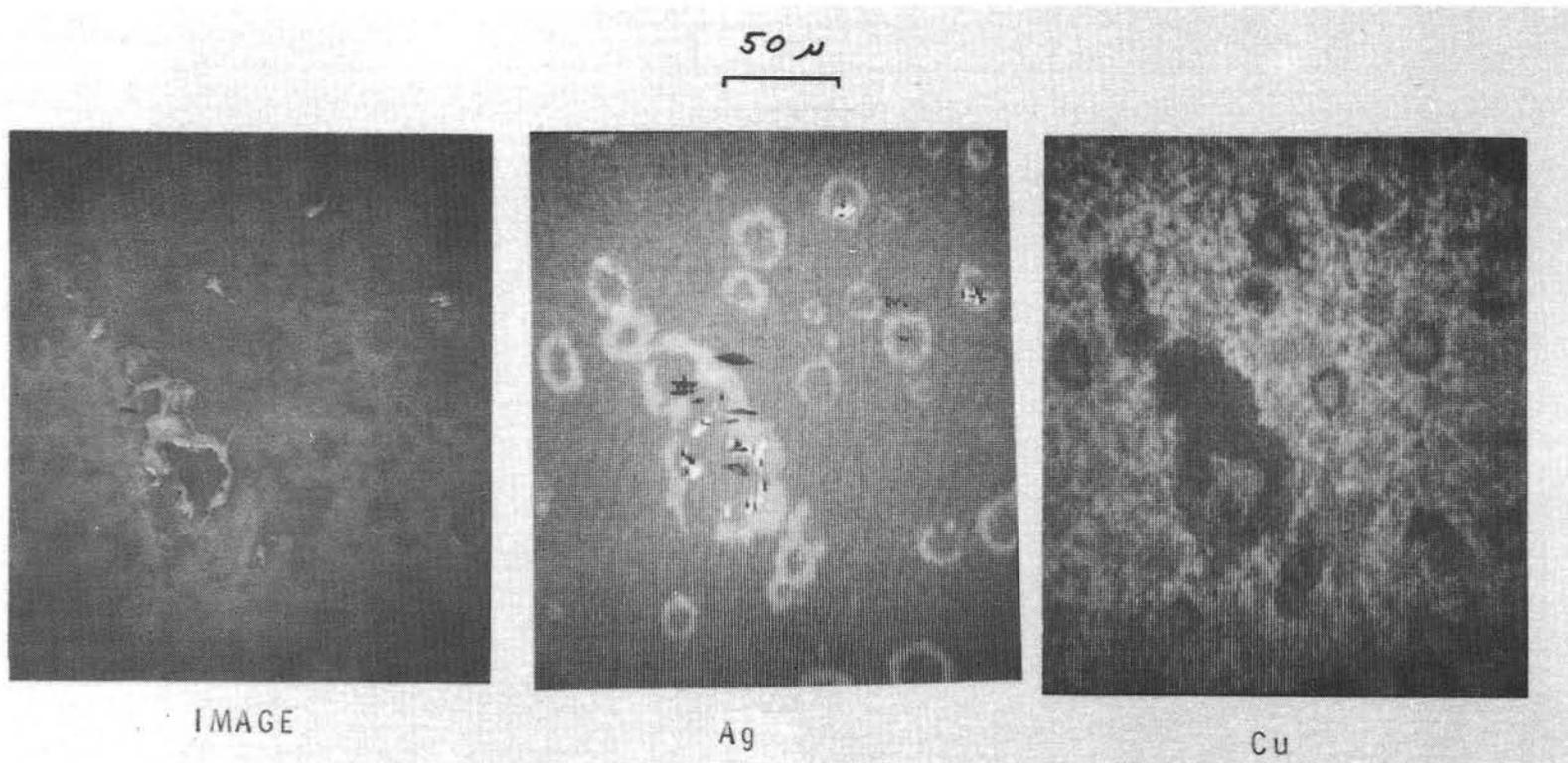
Figure 5. Scanning electron microscope and scanning auger microprobe analyses of localized degradation on mirror reflective surface.
