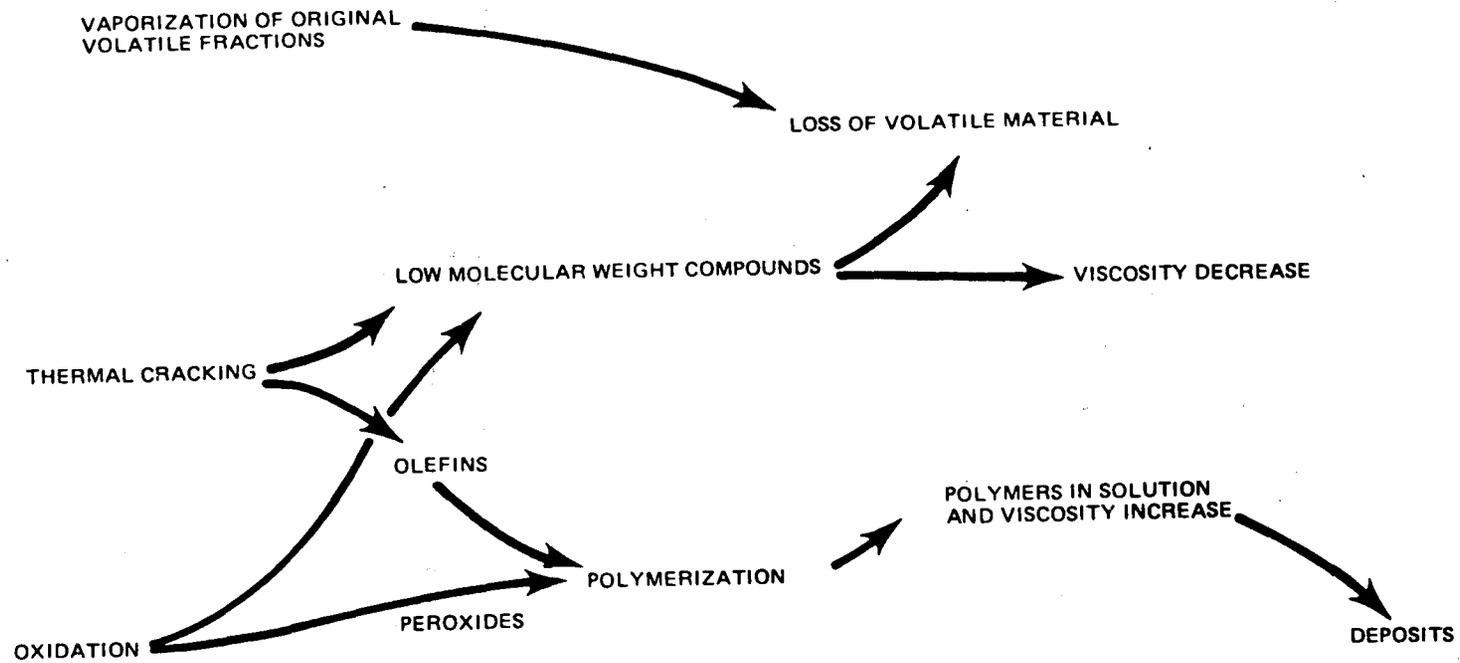
Figure 13. Fluid maintenance considerations for storage of hot oil. (2)
