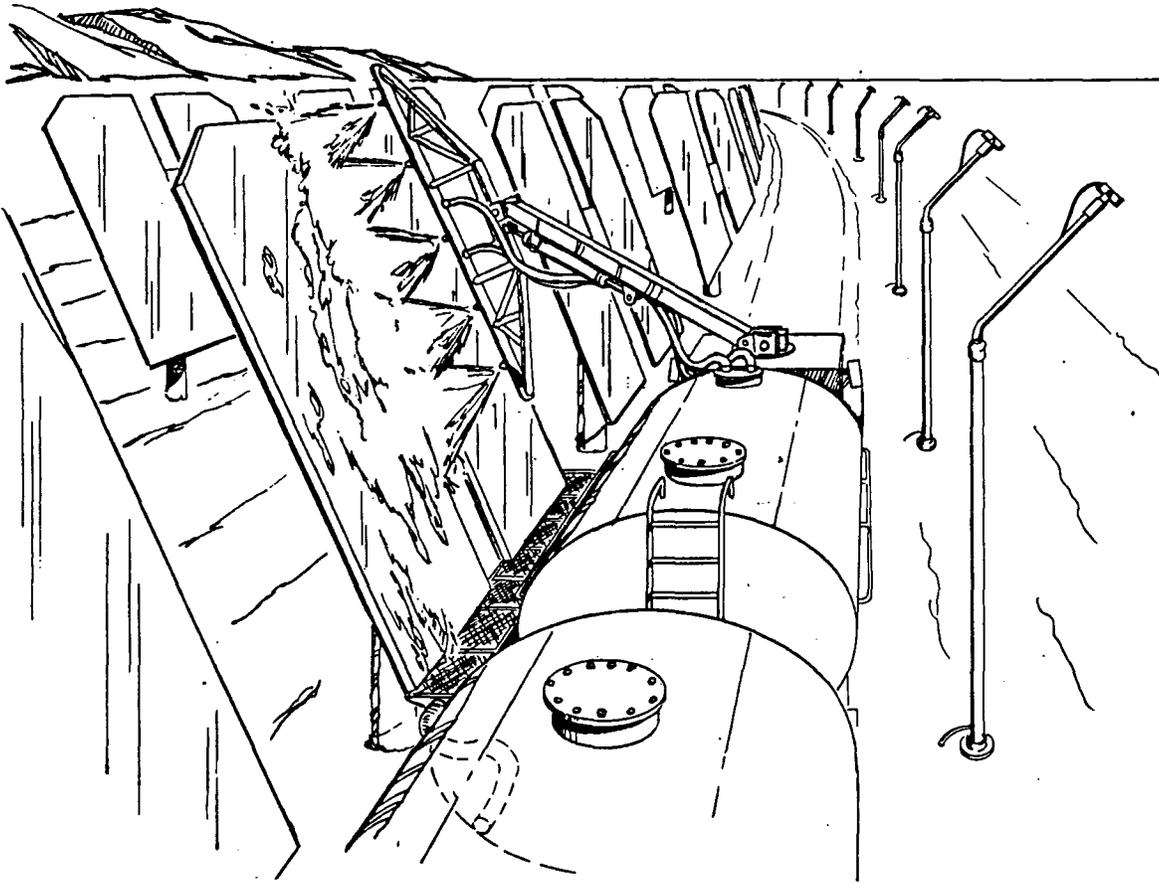
Figure 4. Artists conception of heliostat washing procedure. (2) The sun-sensors shown are not part of the present scheme.
