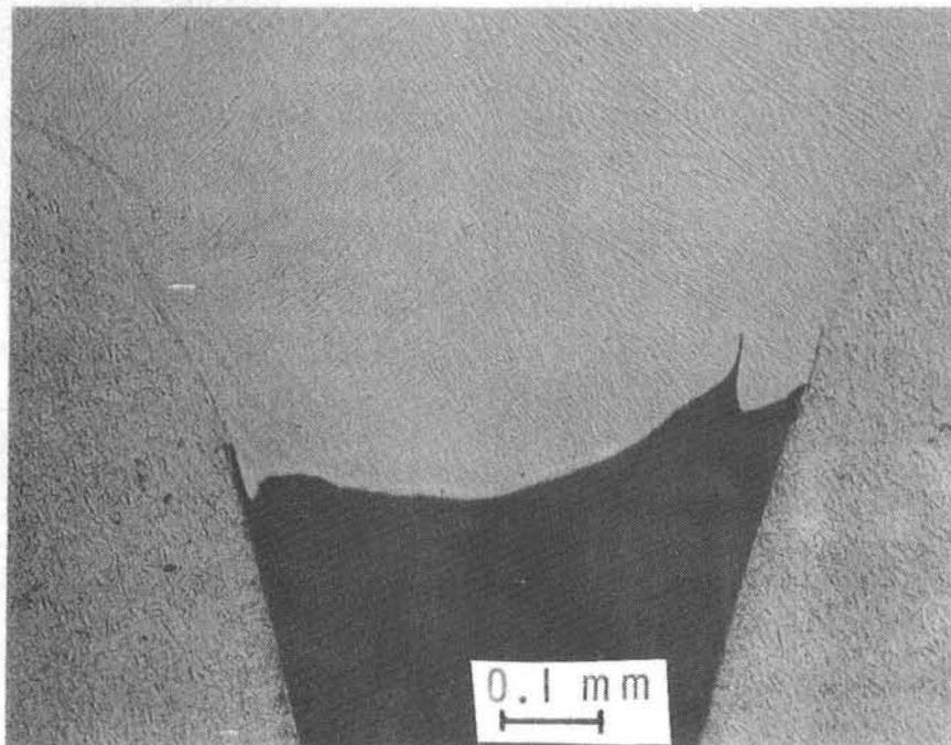
Figure 11. Optical micrograph of welded tube joints.
