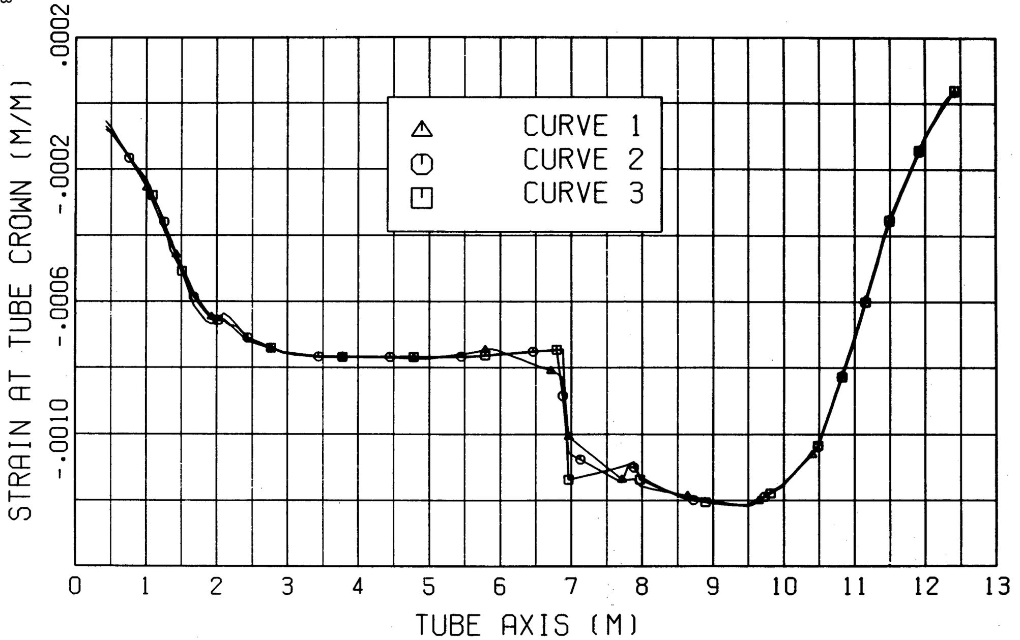
Figure 6. Calculated strains in superheater tubes.
