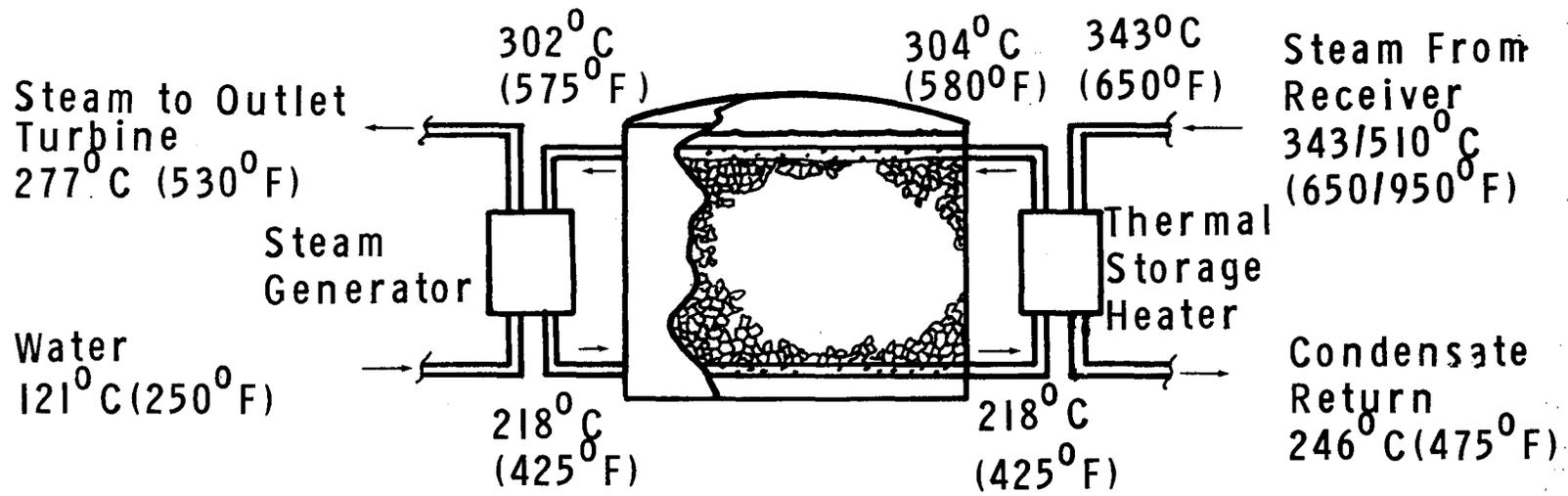
Figure 12. Storage system and secondary steam generator - schematic.
