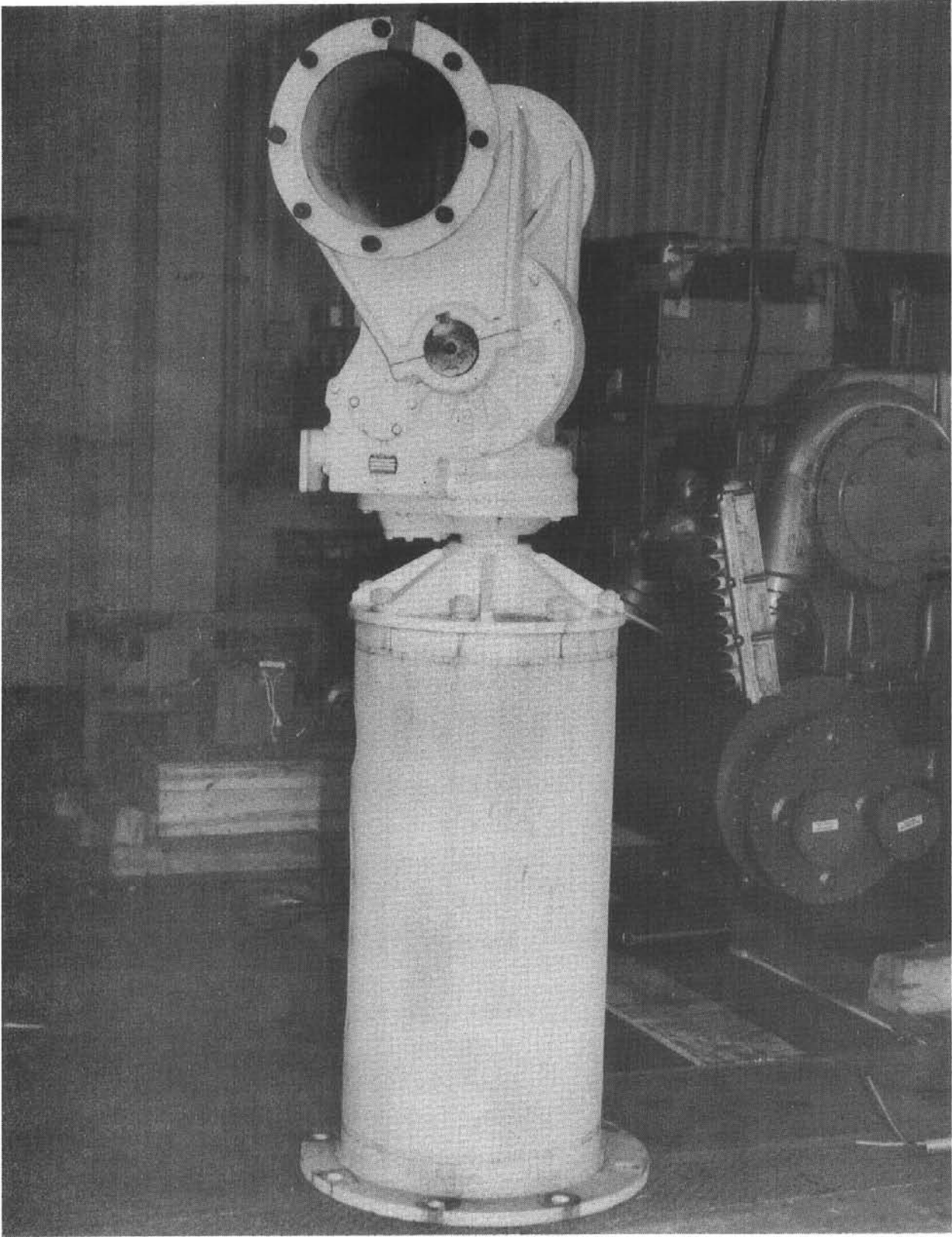
Figure C-8.11. MMC Heliostat after Test with Weights Removed
