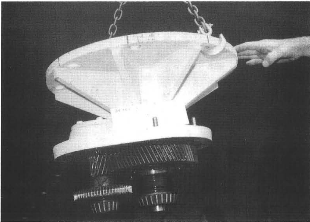
Figure C-8.4. MMC Azimuth Drive Train after Test
