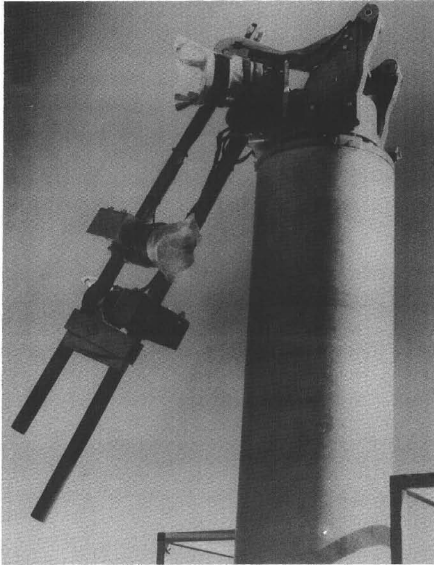
Figure A-10. MDAC Drive Unit Installed on Pedestal
