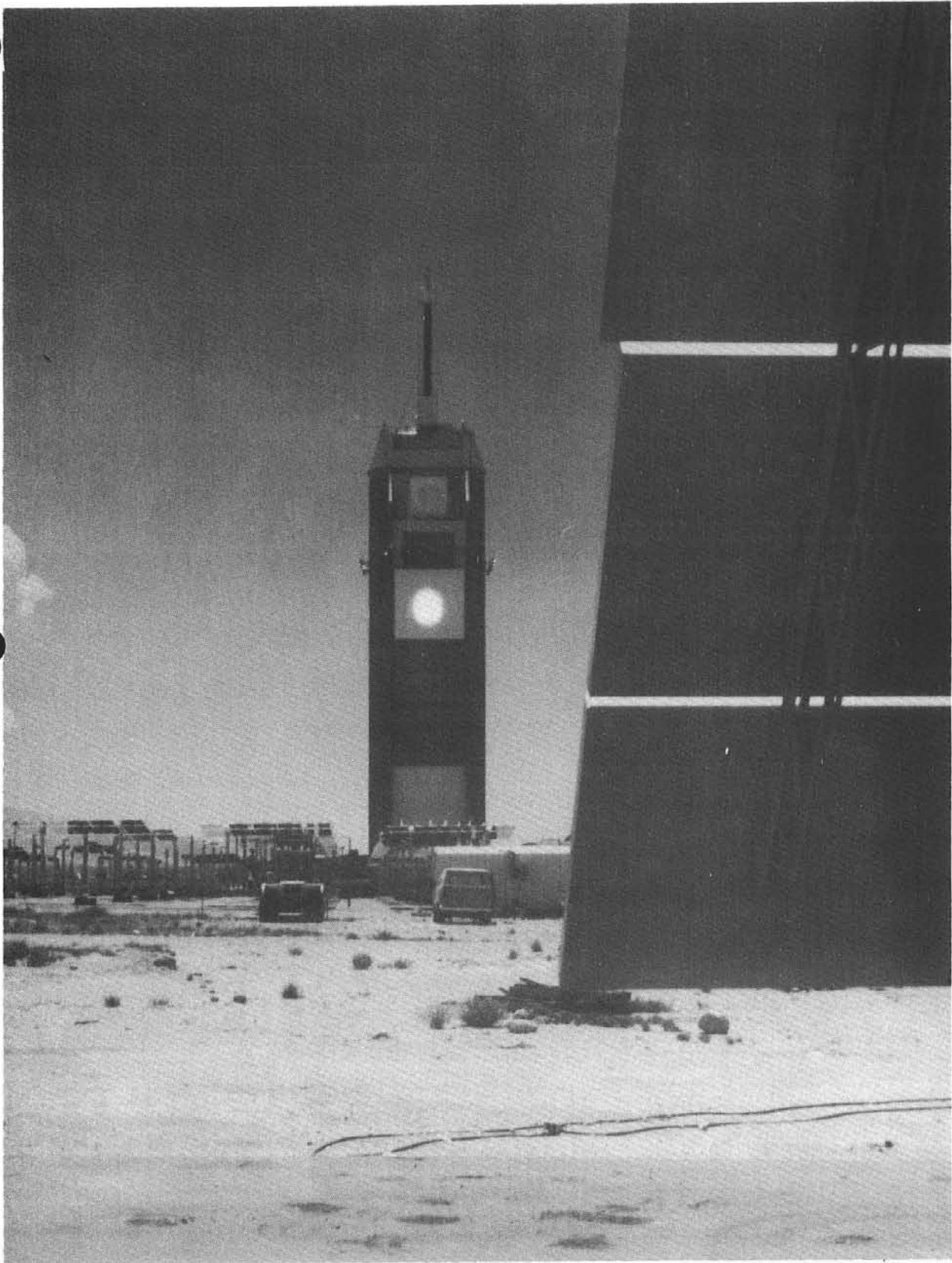
Figure A-7.23. Typical Beam from One of the MMC Heliostats near Solar Noon
