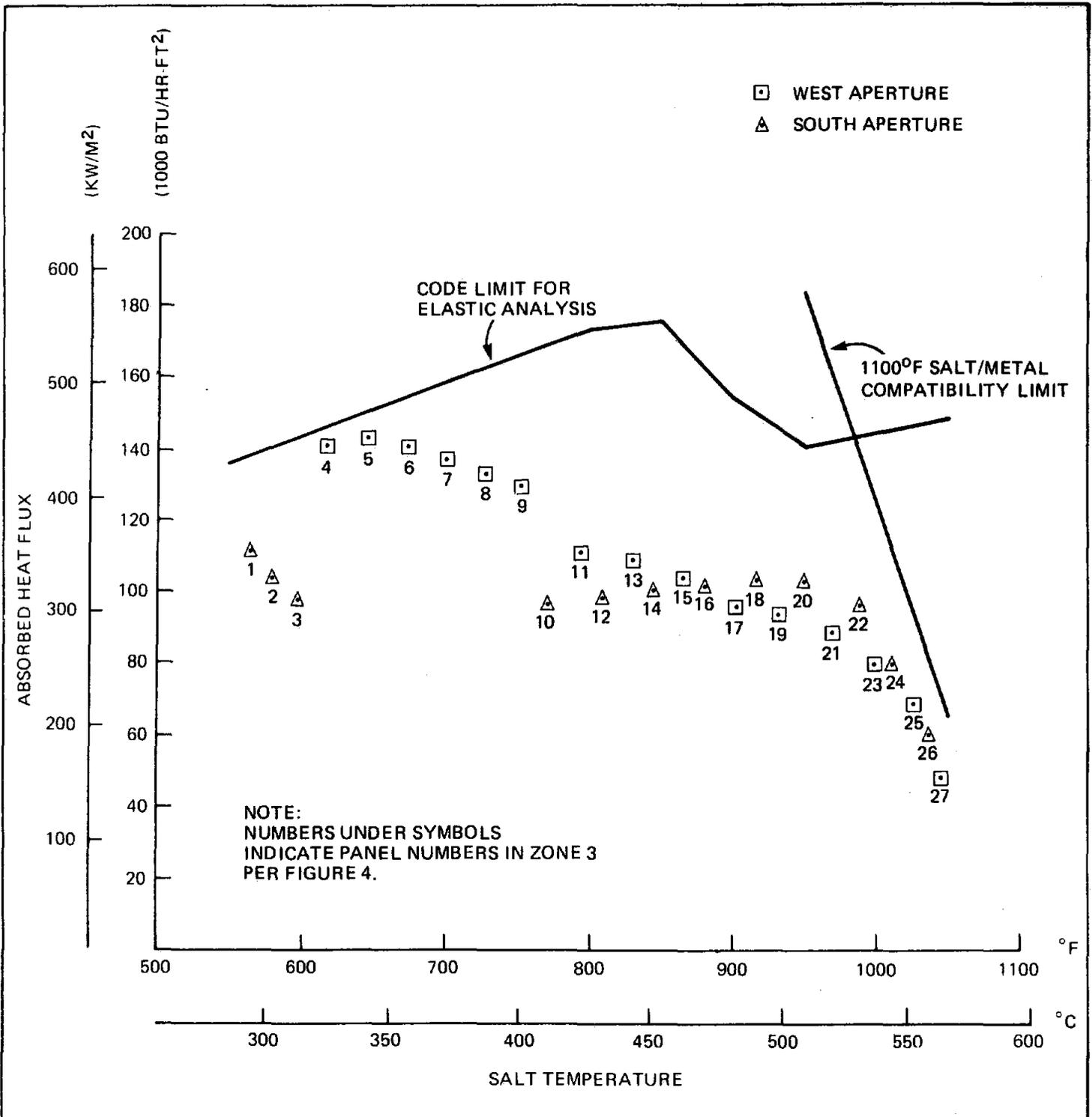
FIGURE 10 ZONE 3 PEAK FLUX AND LIMIT
