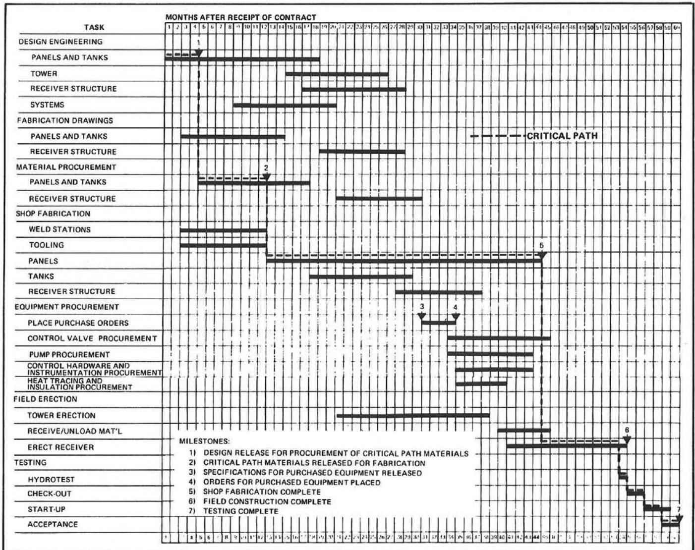
**FIGURE 13 DESIGN, FABRICATION AND FIELD ERECTION SCHEDULE**
