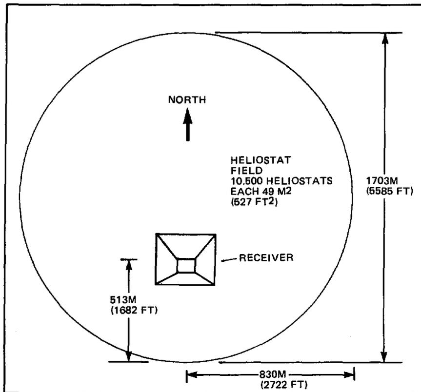
FIGURE 2 POSITION OF RECEIVER RELATIVE TO FIELD
