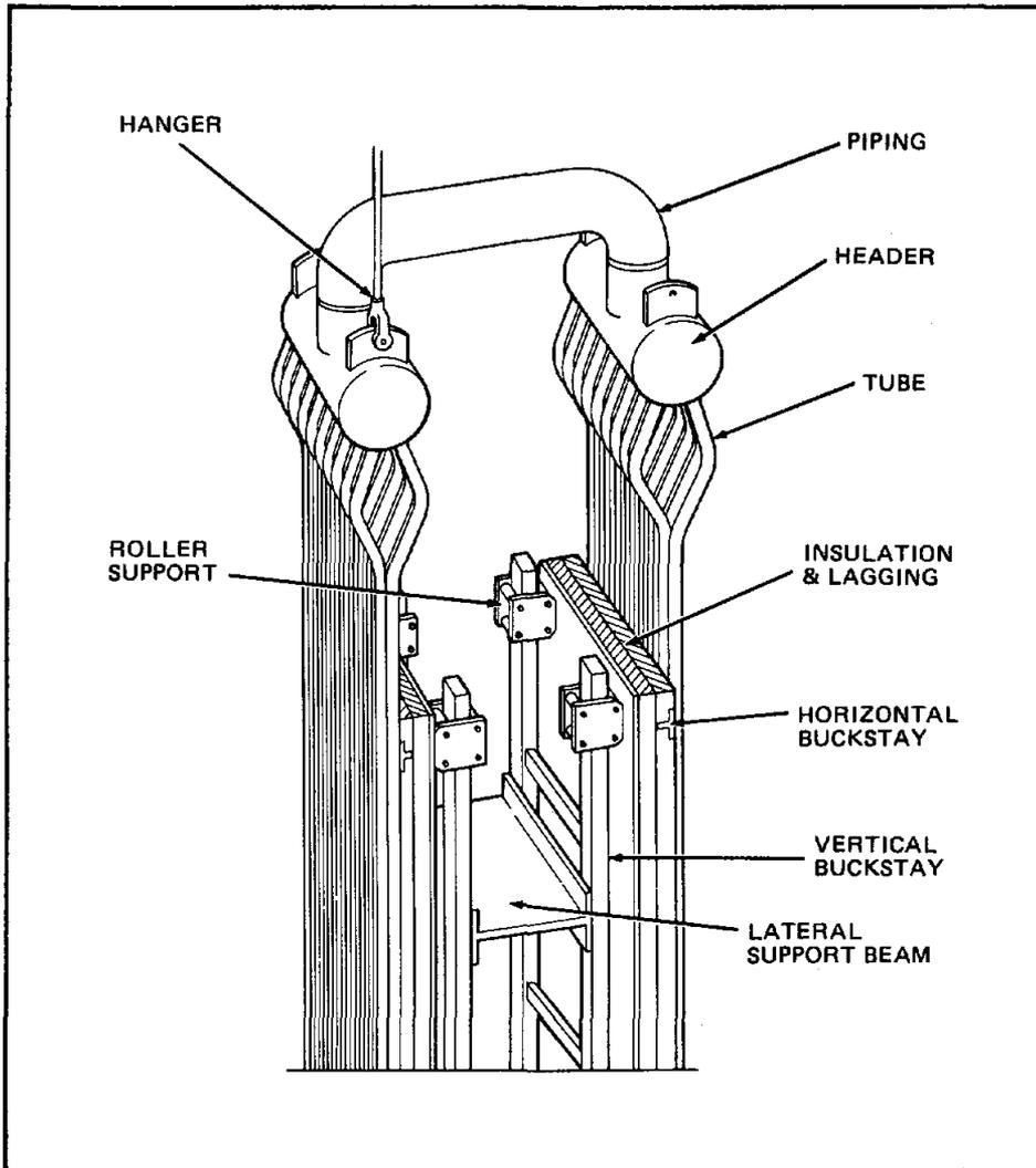
FIGURE 7 DOUBLE WING WALL
