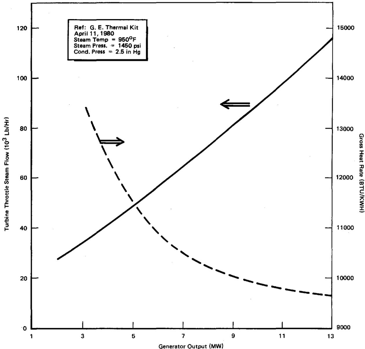
Figure 3.2. Baseline Turbine Cycle Performance Characteristics
