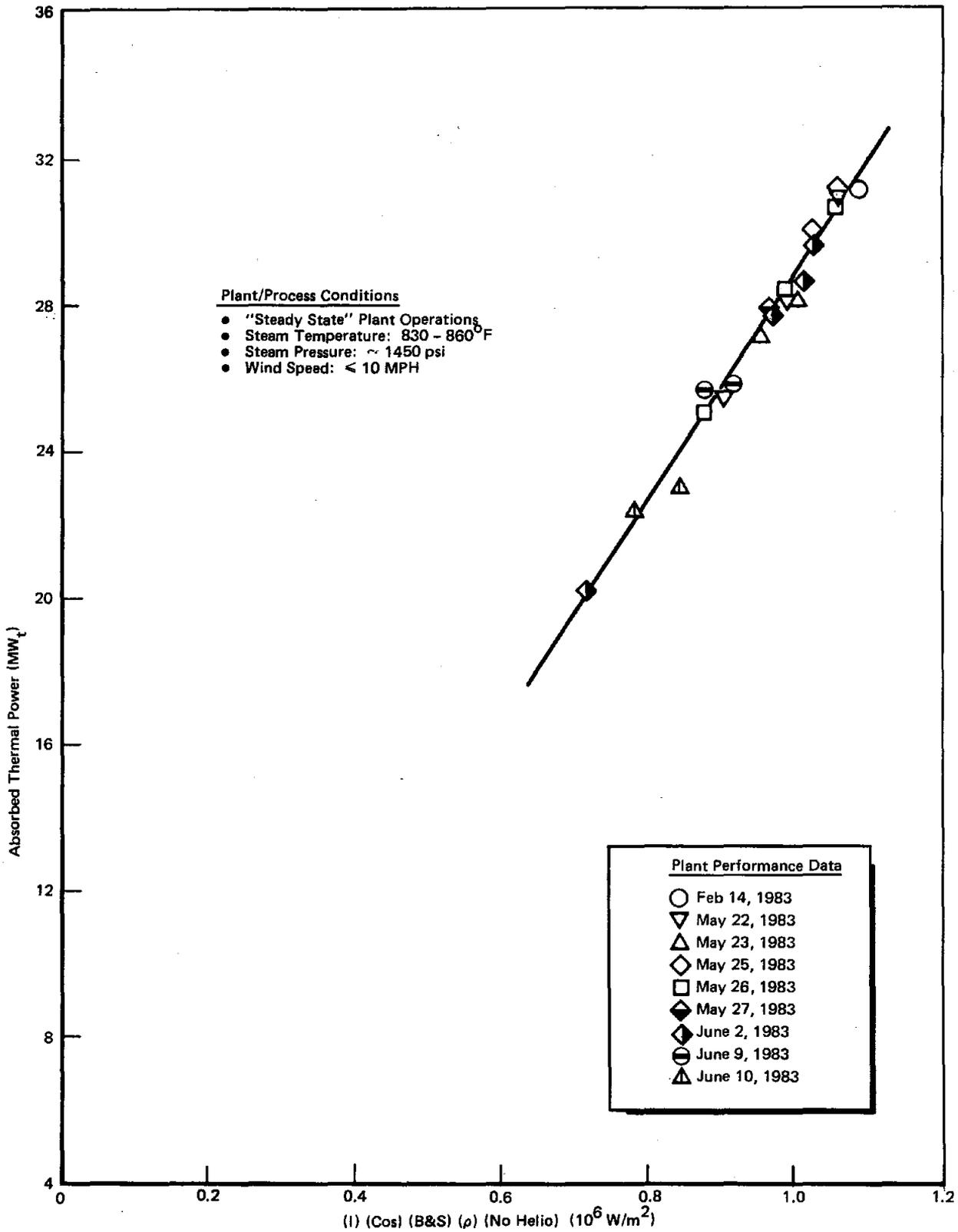
Figure 5.9. Receiver Absorbed Power as a Function of Collector Field Power (Steam Temperature 830 - 860°F)
