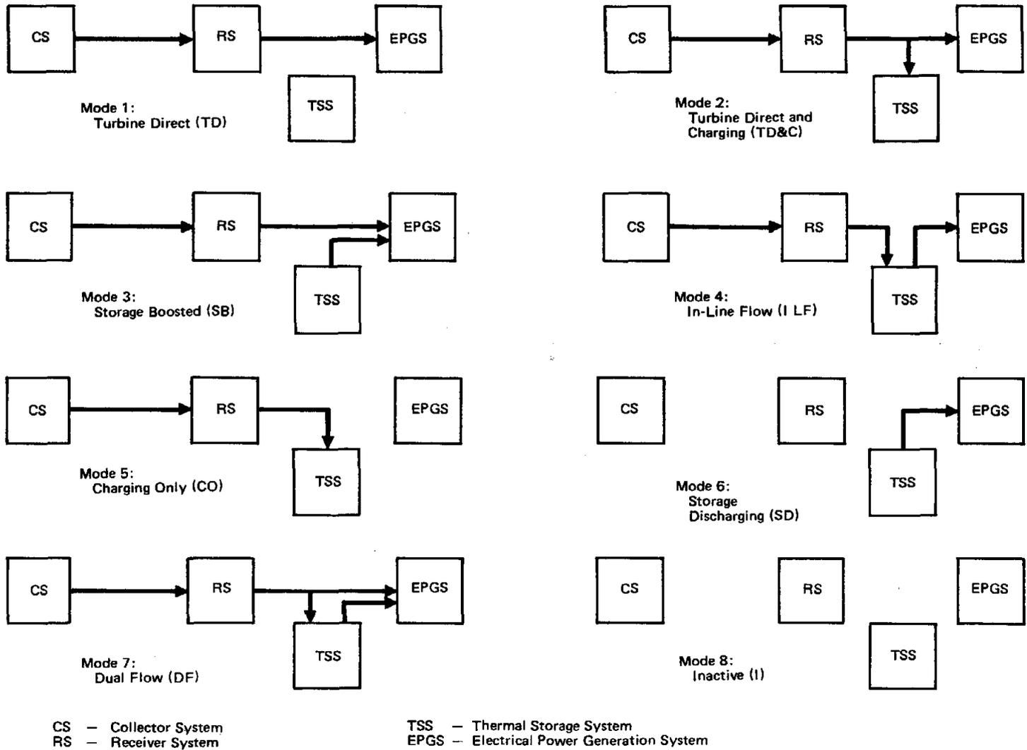
Figure 1.2. Solar One Plant Operating Modes
