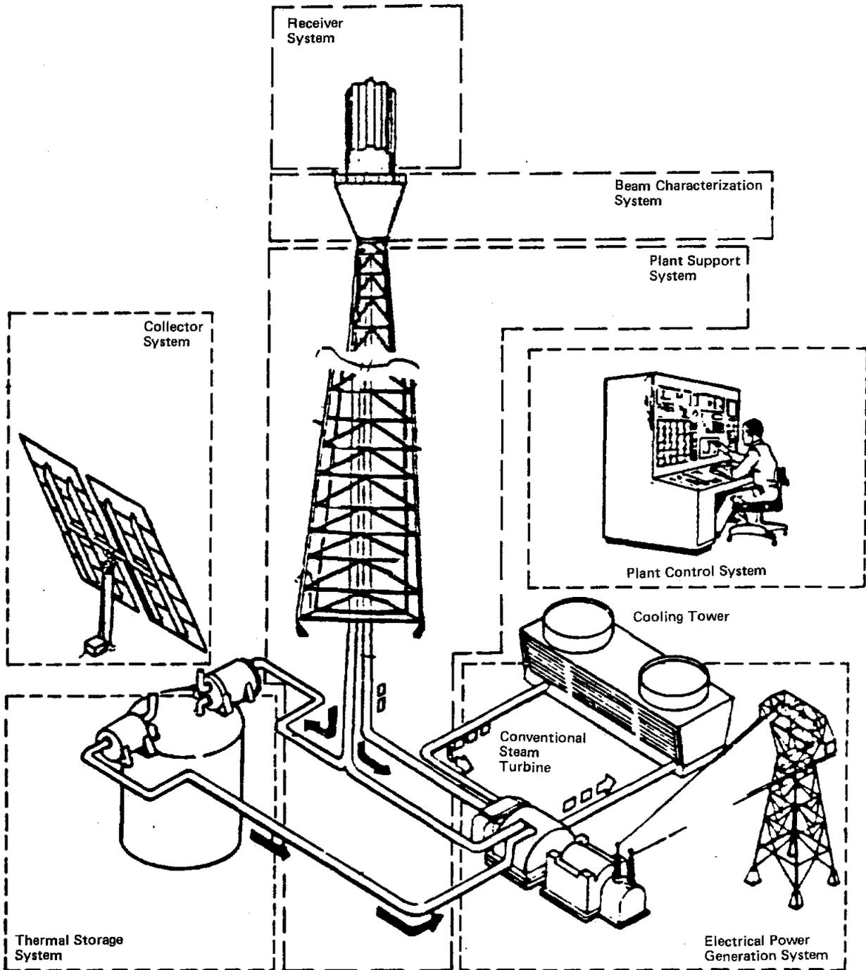
Figure 1.1. Solar One System Schematic
