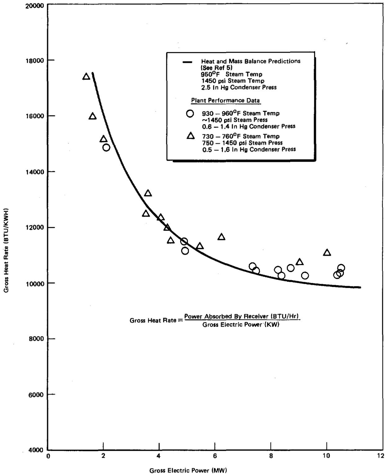
Figure 5.4. Gross Heat Rate for Water/Steam Cycle Portion of Plant
