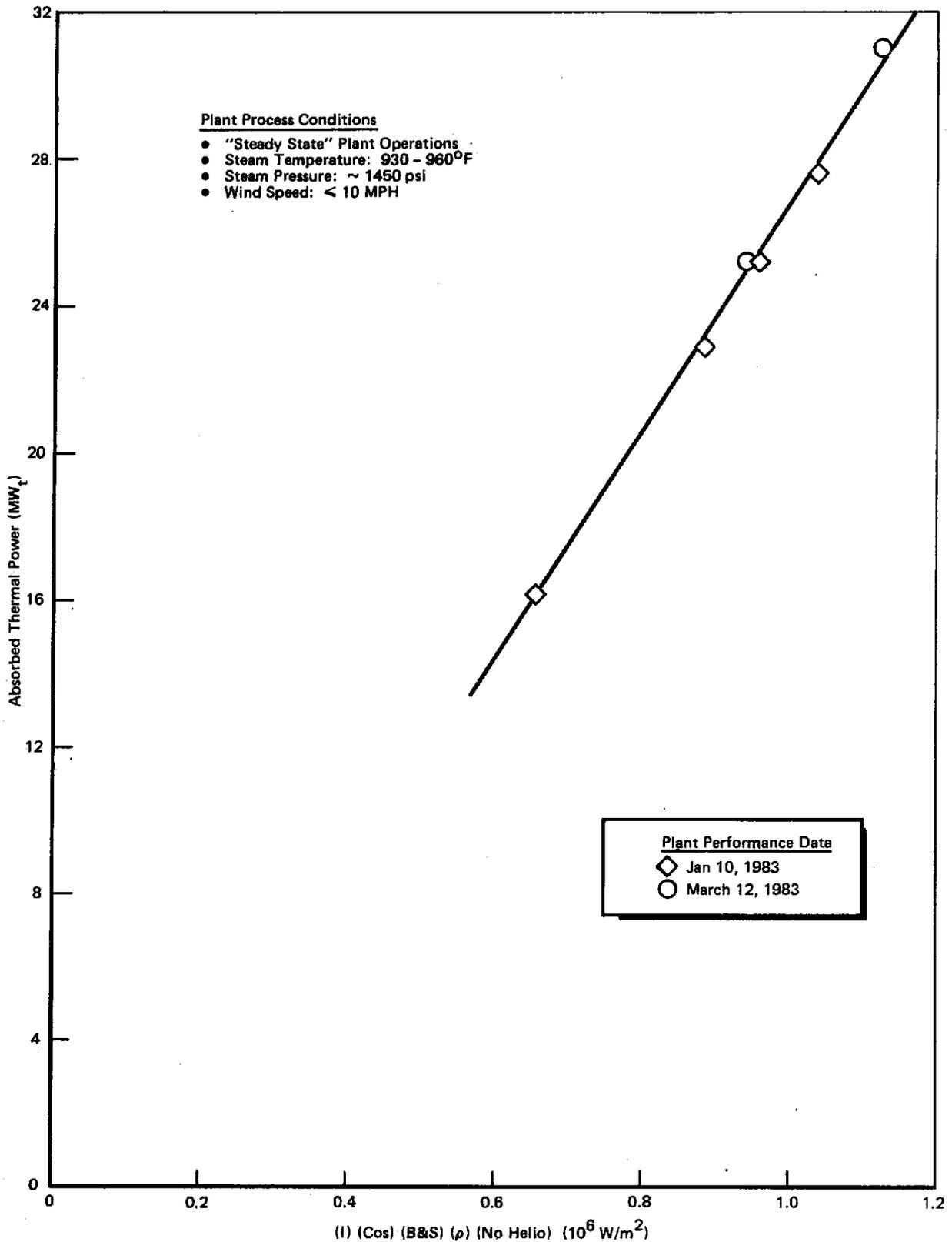
Figure 5.8. Receiver Absorbed Power as a Function of Collector Field Redirected Power (Steam Temp 930 - 960°F)
