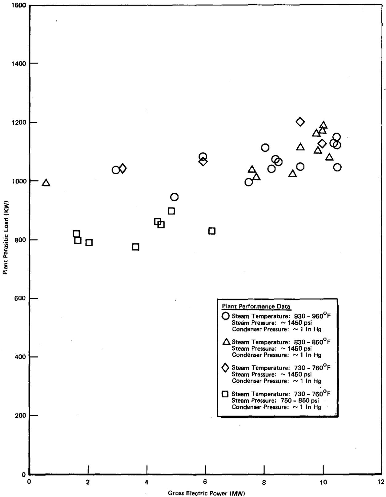
Figure 5.7. Measured Plant Parasitic Loads
