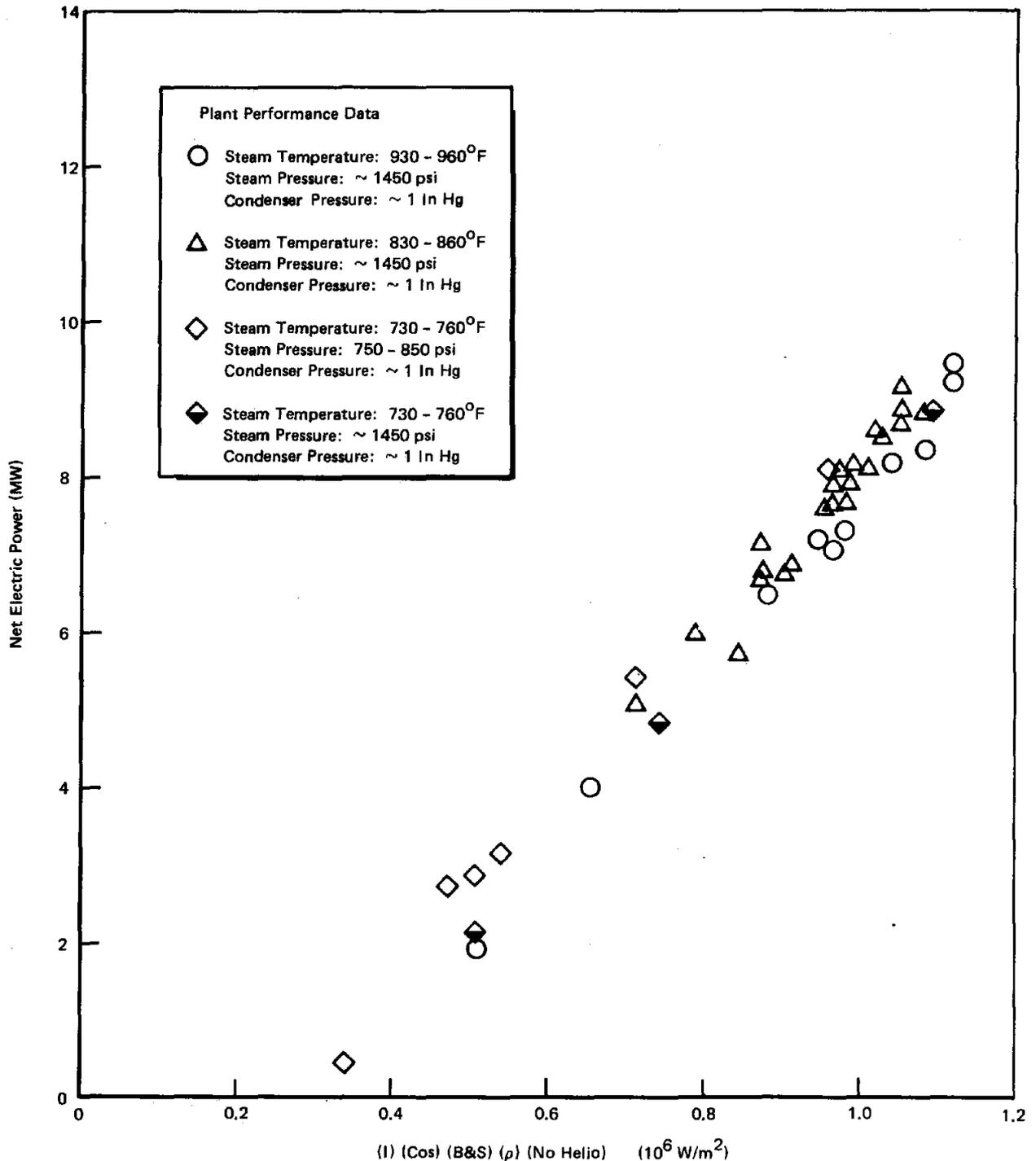
Figure 5.12. Net Electric Power As a Function of Collector Field Redirected Power Parameter
