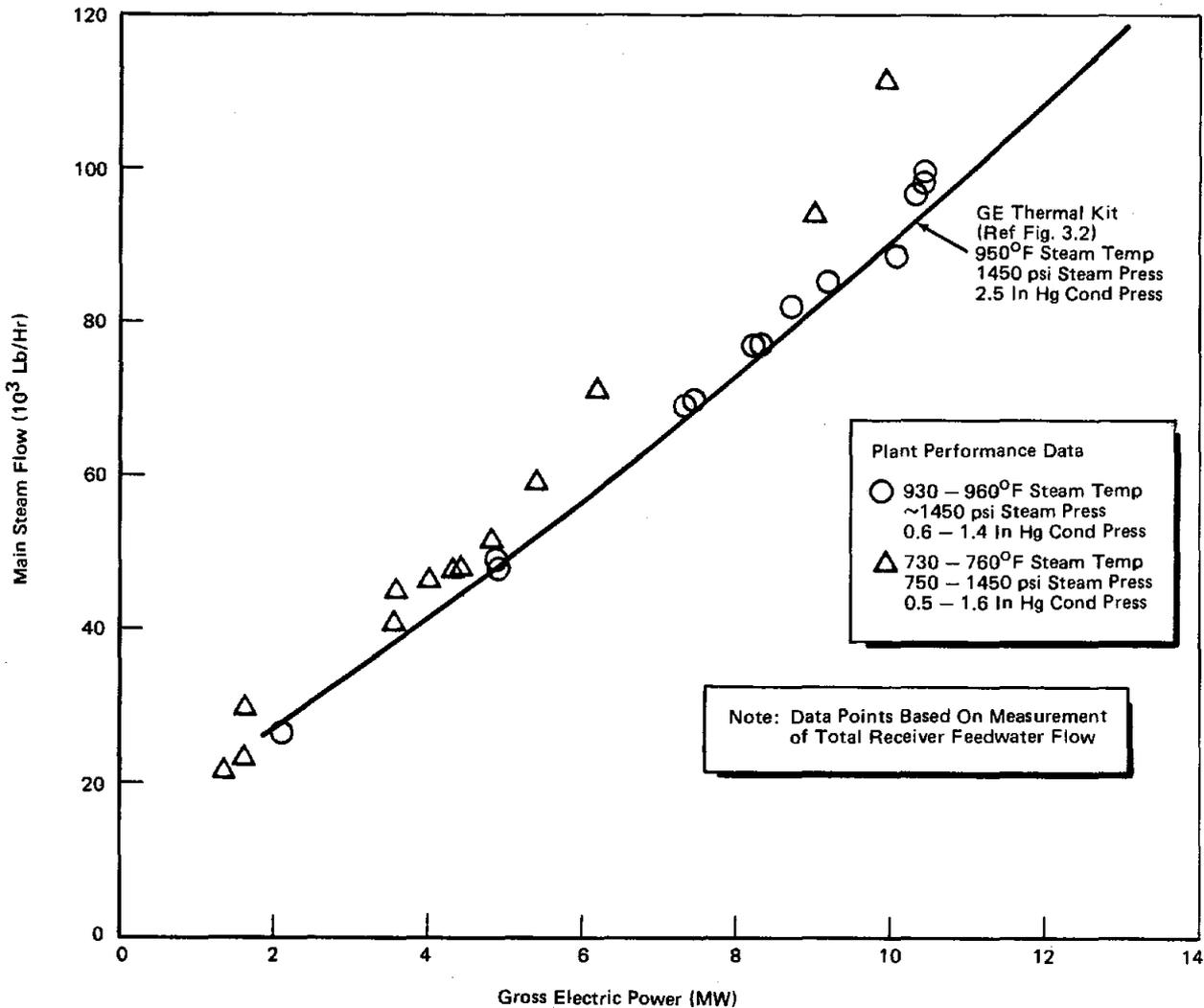
Figure 5.1. Main Steam Flow Required for Gross Electric Generation
