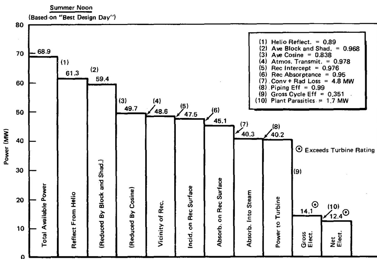
Figure 3.1. Solar One Mode 1 Design "Waterfall Efficiency" Chart
