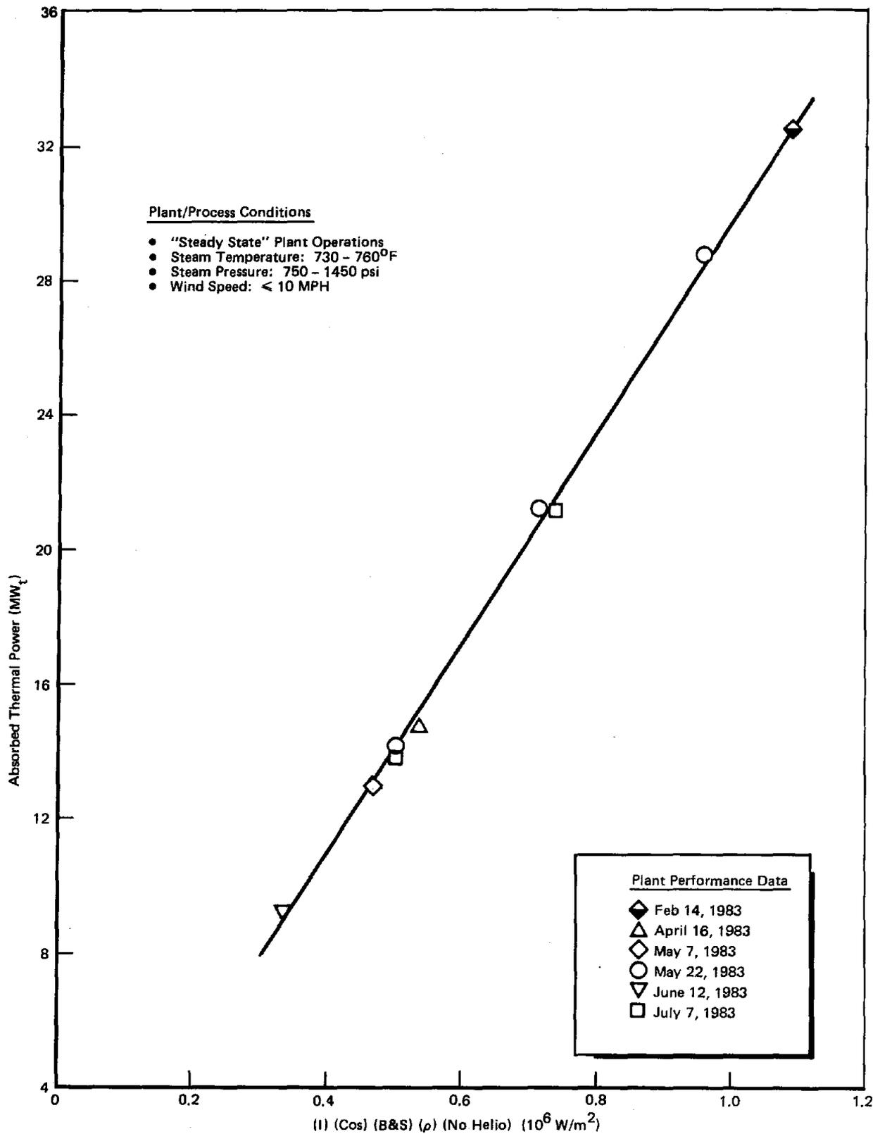
Figure 5.10. Receiver Absorbed Power as a Function of Collector Field Redirected Power (Steam Temp 730 - 760°F)
