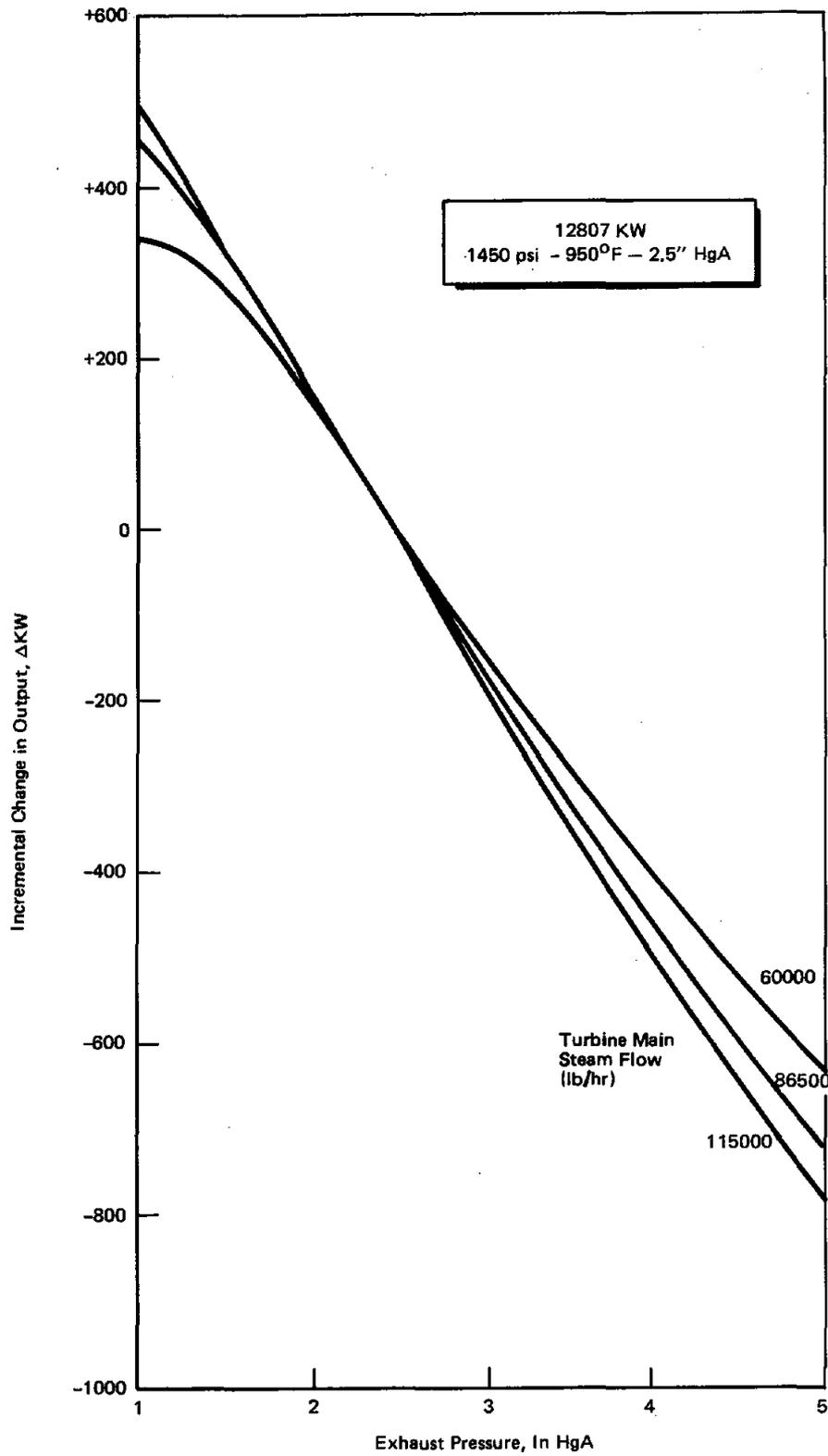
Figure 3.4. Impact of Turbine Exhaust Pressure on Electrical Output
