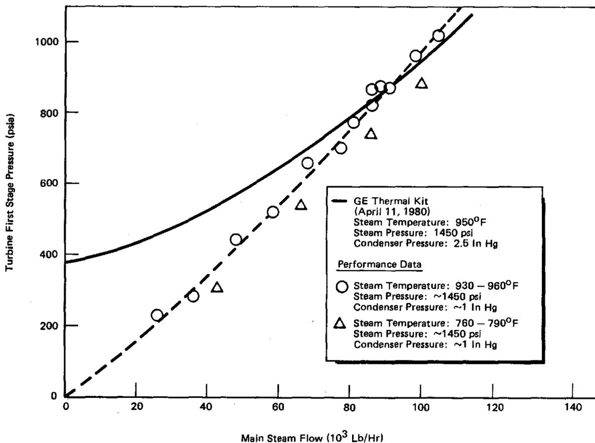
Figure 5.3. Comparison of Turbine First Stage Pressure to Main Steam Flow
