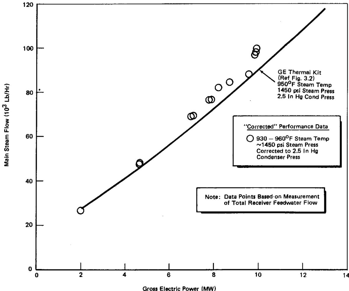
Figure 5.2. Performance Comparison Employing "Corrected" Condenser Pressure
