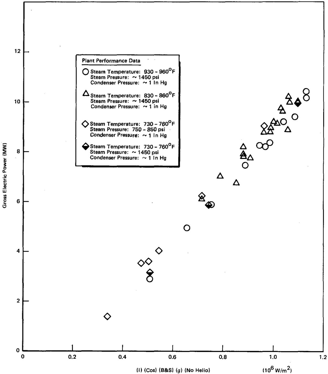
Figure 5.11. Gross Electric Power as a Function of Collector Field Redirected Power Parameter
