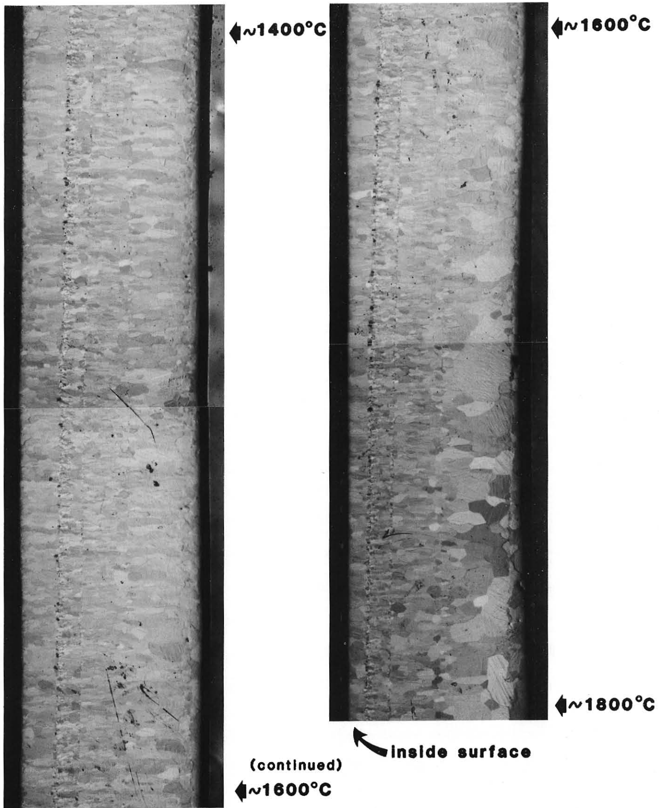
Fig. 127 CVD RE TUBE METALLOGRAPHIC SECTIONS.
