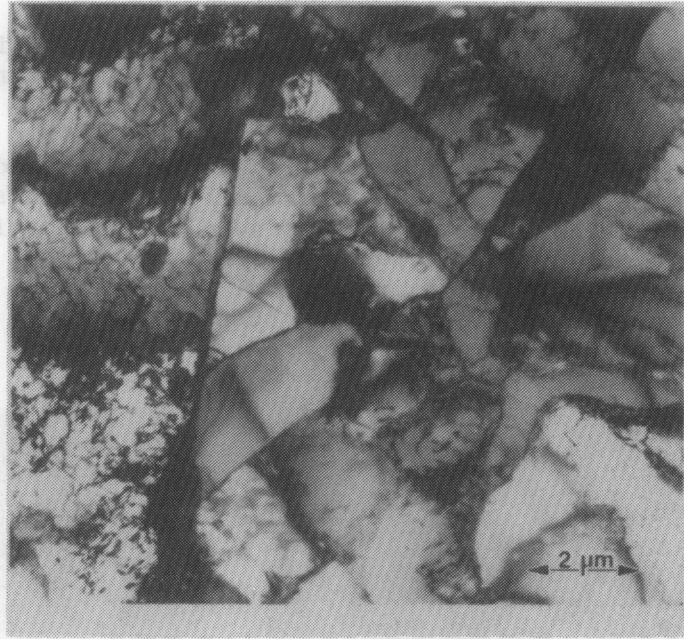
Figure 11. Transmission electron micrograph of Alloy 800 thermomechanical HTC cycled, 60 s/cycle, 75 hr. test duration.
