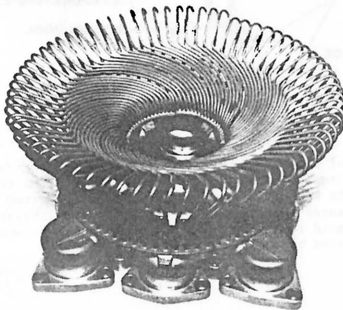
United Stirling ESOR-IIB heater head used on the Advanco Dish-Stirling Module. The oversized heater head tubes are spread out to improve the flux distribution and reduce thermal stress, but engine and receiver performance are compromised.
