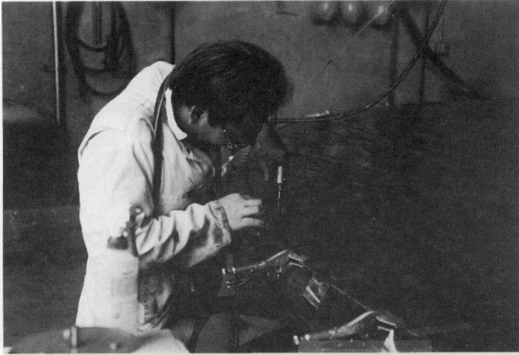
Figure 12.0-12. Tensioning Strips to Membrane Weld (View 1)
