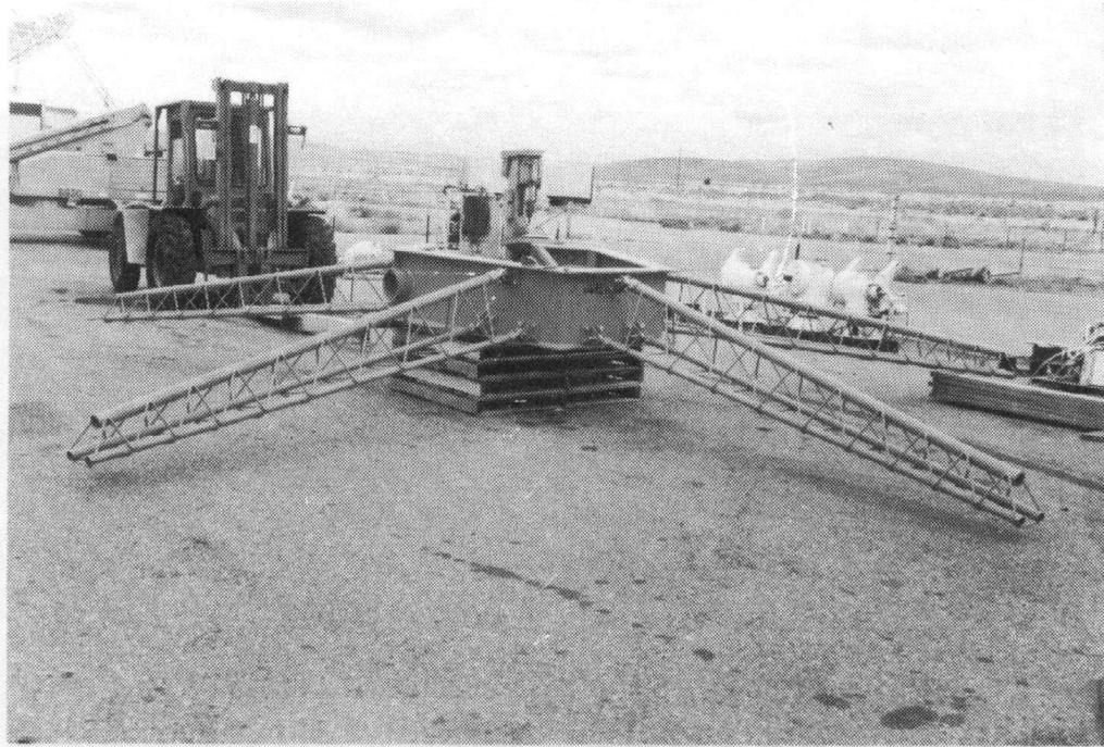
Figure 12.0-18. Truss/Hub Subassembly
