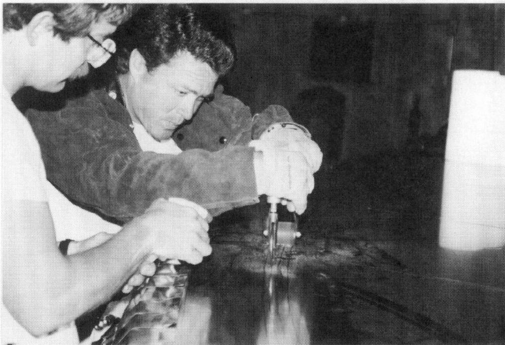
Figure 12.0-17. Membrane to Ring Welding
