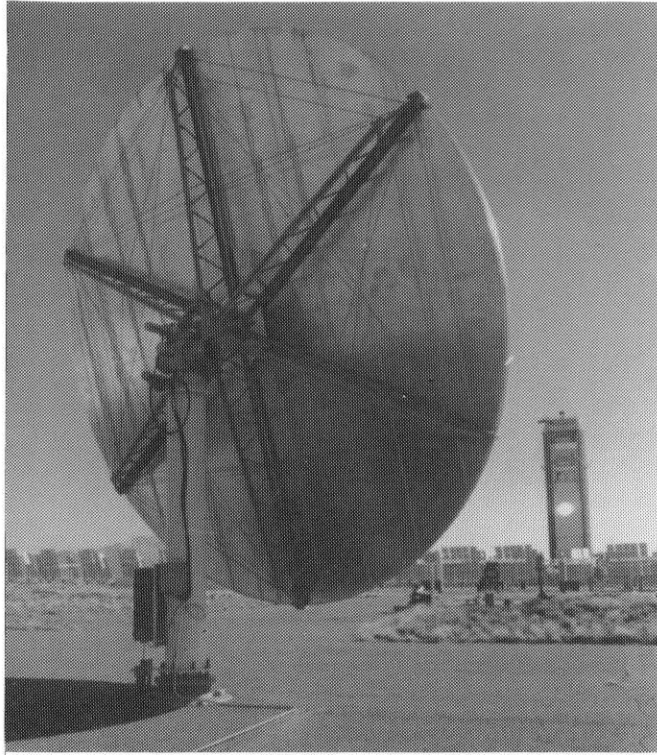
Figure 10.17 Rear View of the SKI Mark II Prototype Heliostat.
