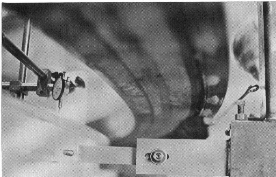
Figure 10.12 Heliostat Ring Channel Segment and Ring Support Pylon. The ring is being adjusted to set planarity and radius with dial indicators mounted on the central sweep arm.
