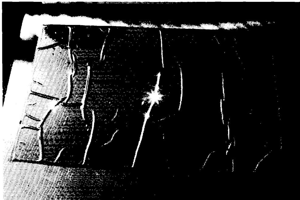
Figure 5 - Failure of ECP-305/polyester/Y-9415 laminate during immersion testing
