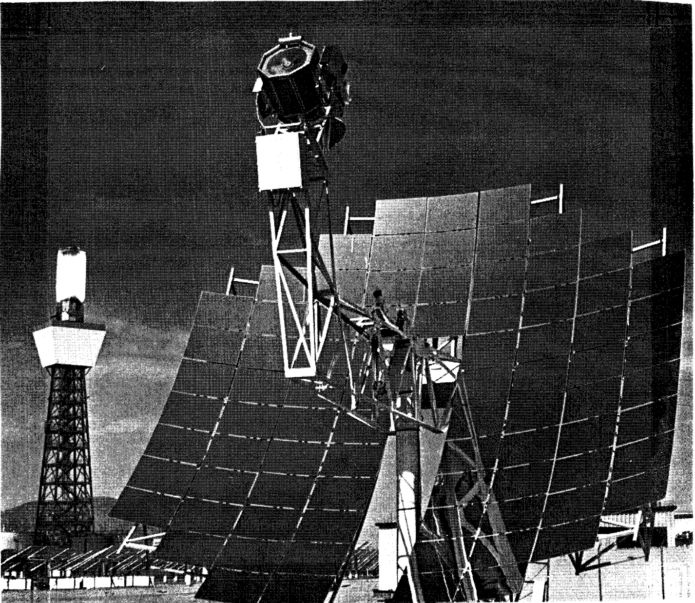
Figure I-1. Stirling Dish Operating at the SCE Test Site With Solar One in the Background.
