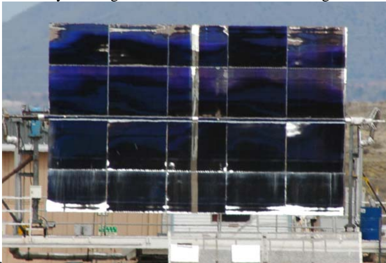
Figure 3: Picture of the mirror alignment of the LS-2 concentrator with the Schott HCE on the rotating platform, after the mirrors were aligned.
