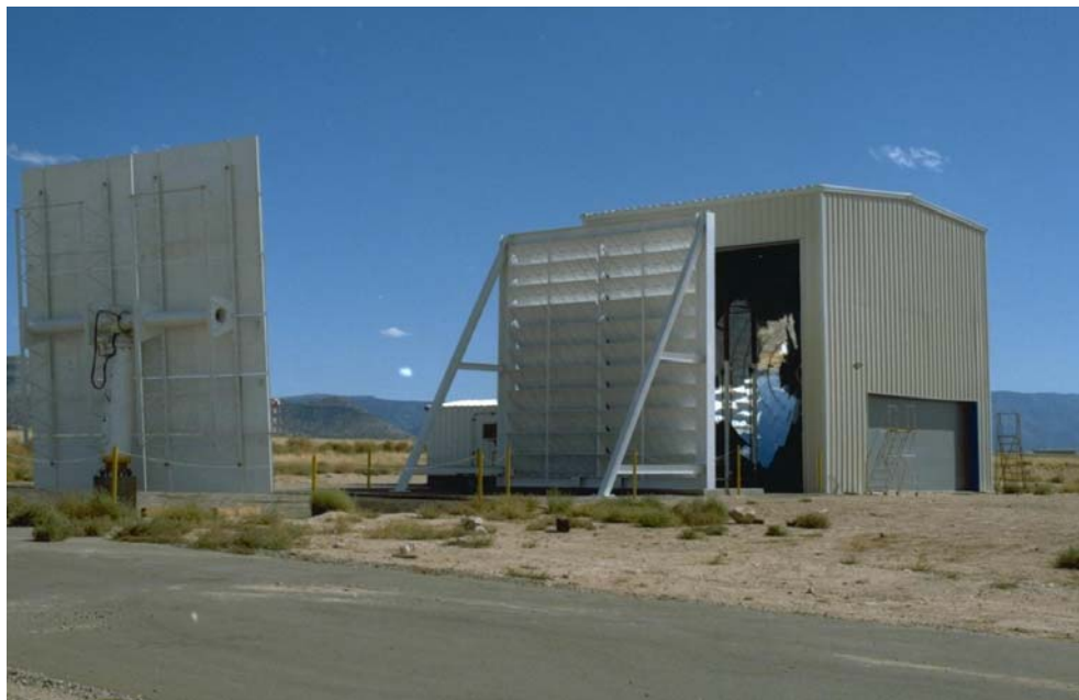
Figure 6. Photograph of the NSTTF solar furnace facility. A large Venetian-blind like attenuator located between the flat heliostat and parabolic dish concentrator allows the solar power to the experiment to be varied.
