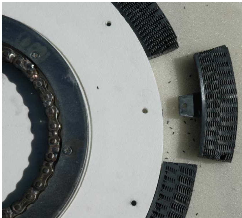
Figure F-2. Photograph of a reactant ring showing the attachment of the reactant fins to carrier ring.
