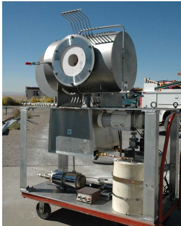
Figure F-3. Photograph of the CR5 test assembly. On the top part of the skid the CR5 vacuum vessel, injector s, and aperature insulation assembly can be seen. On the lower half are the tube in tube condensers, water traps, control valves, vacuum pumps, and steam generator.
