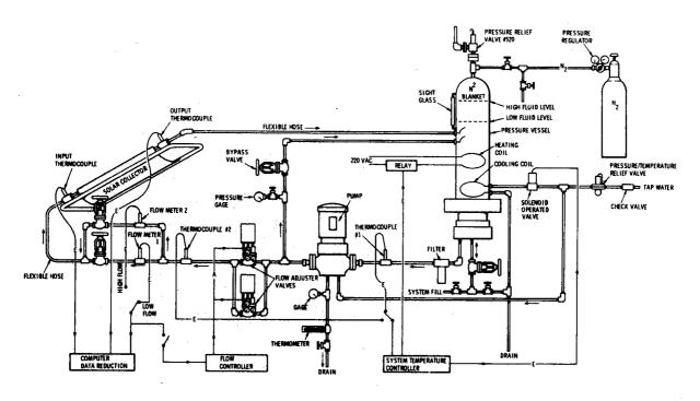
Figure 3. Instrumentation fluid loop, Solar Collector
