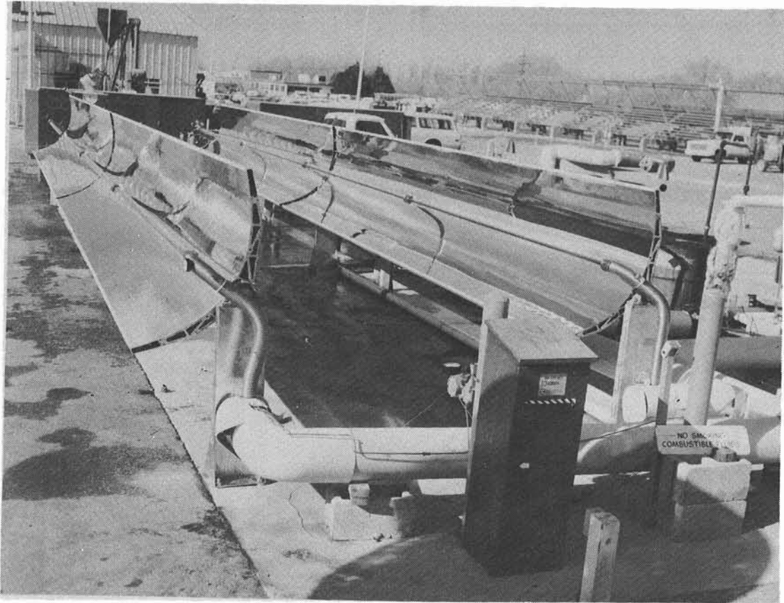
Figure 9. Solar Kinetics Solar Collector
