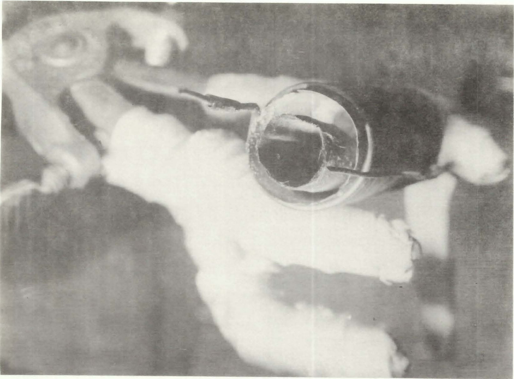
Figure II-11. View of Distorted Retainer Screen in Unit I Reactor
