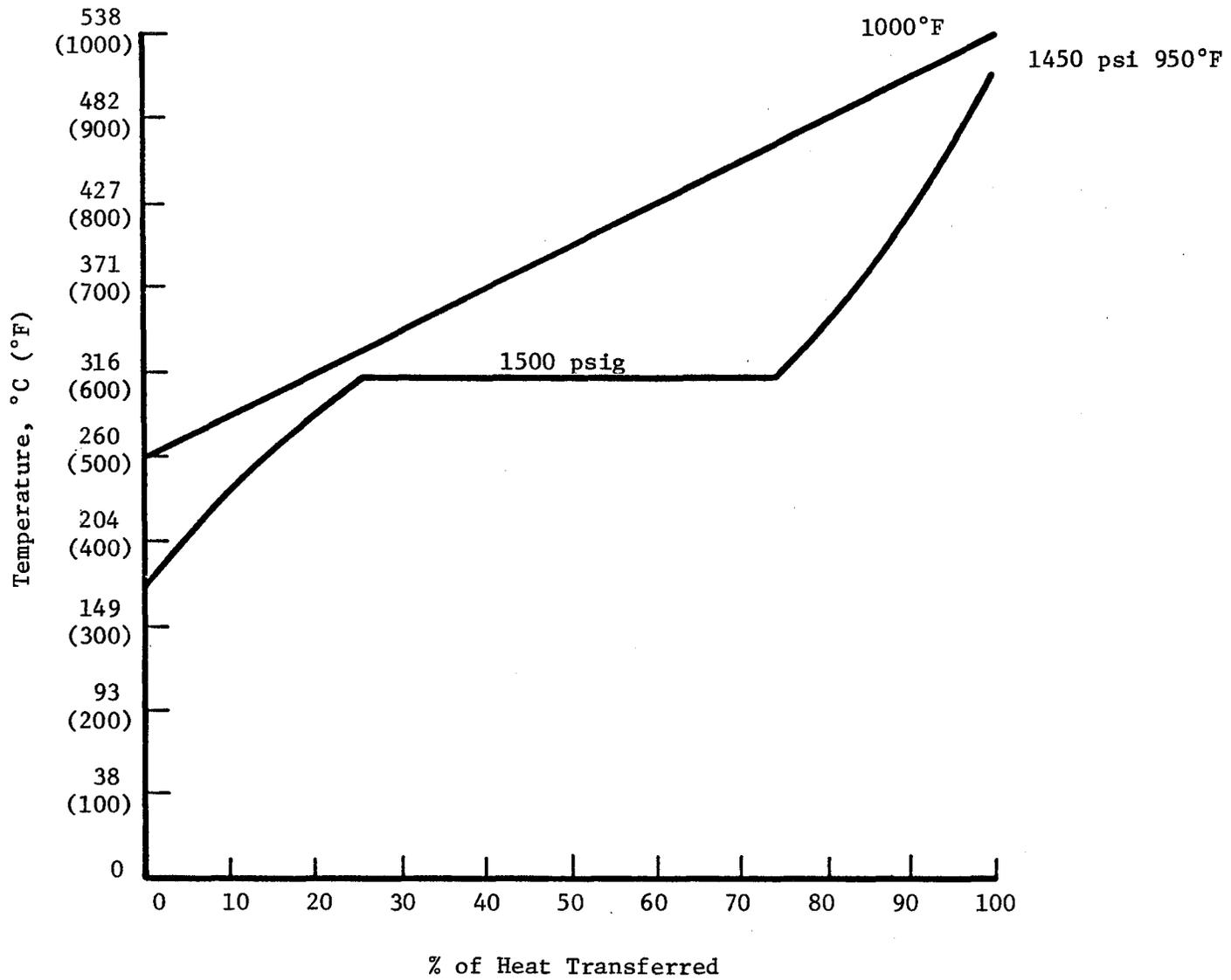
Figure 7-2. Special Temperature Diagram for Solar Plant Using High-Temperature Thermal Storage and Reheat Steam Cycle With Reduced Final Feed Temperature and Two-Stage Reheat in Charge and Discharge Modes
