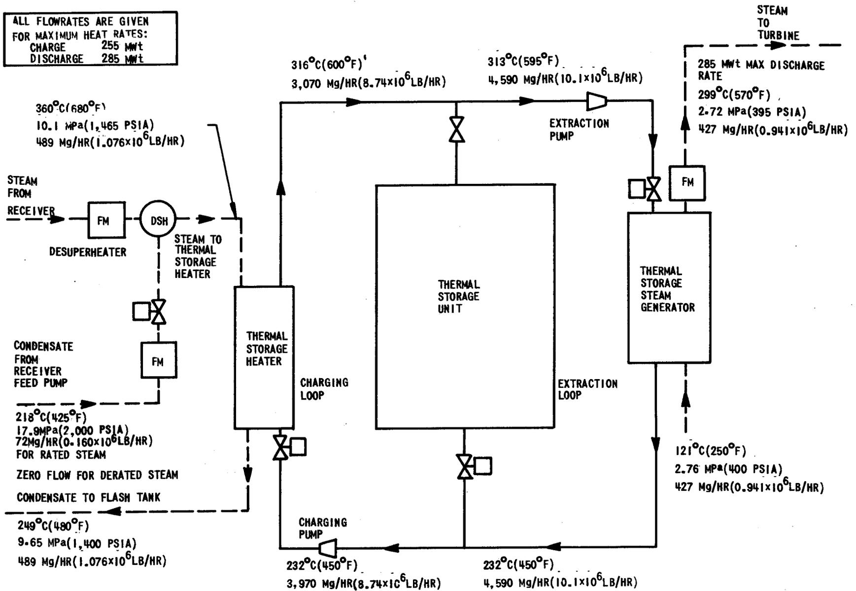
Figure 4-2. Oil/Rock Temperature-Energy Diagram
