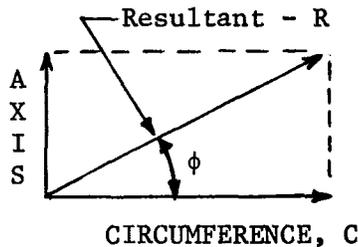
$$\cos \phi = \frac{C}{R} \quad (\text{Note: This } \phi \text{ is the same as OD helix angle.})$$
