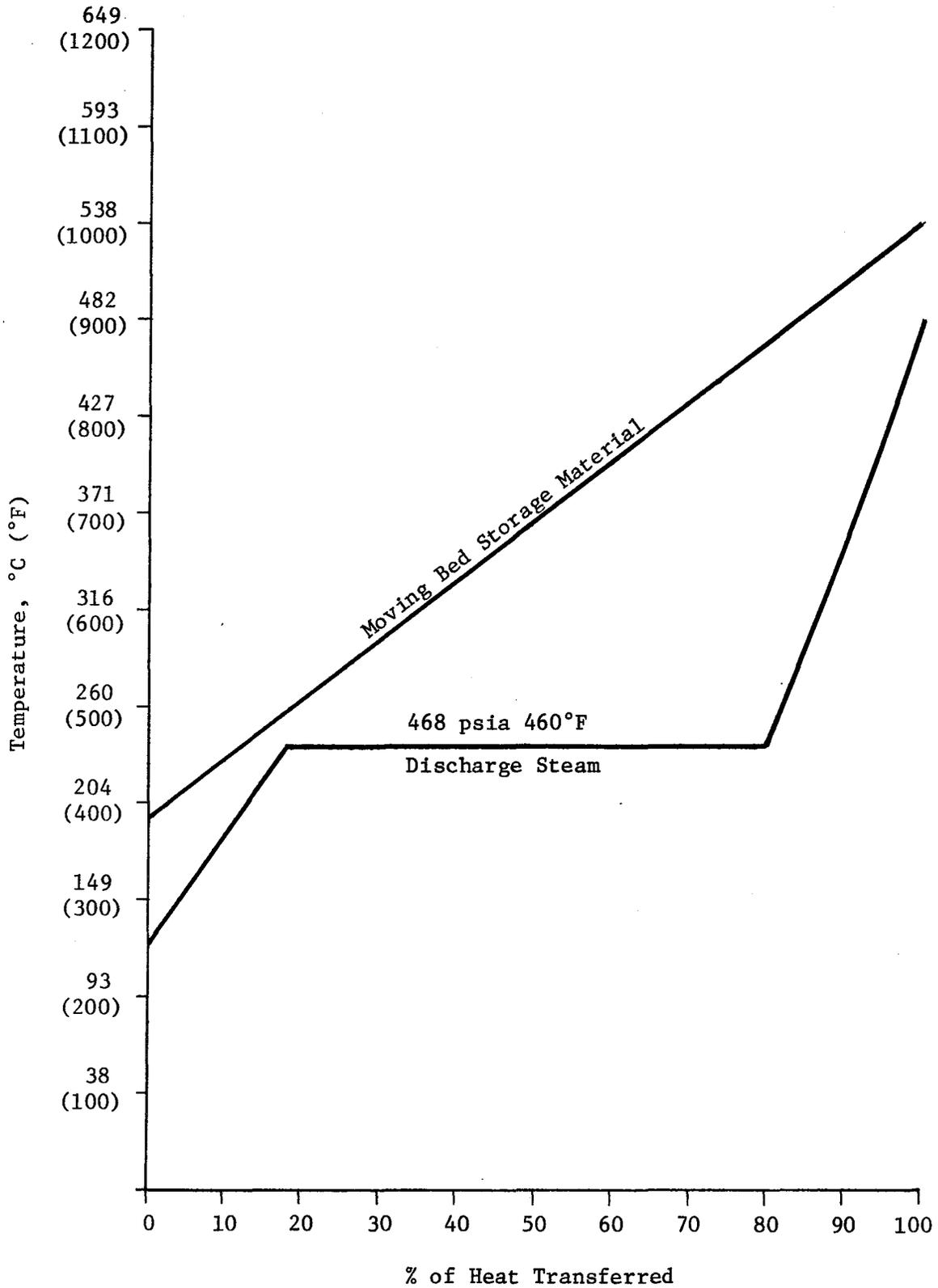
Figure 7-4. Charge/Discharge Temperature Diagram
