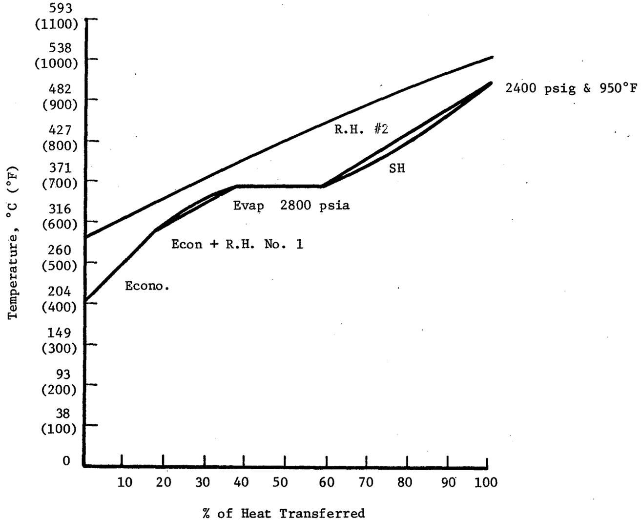
Figure 7-3. Temperature Diagram for Single-Stage Moving Bed Thermal Energy Storage, 468 psia, 900F Steam Cycle
