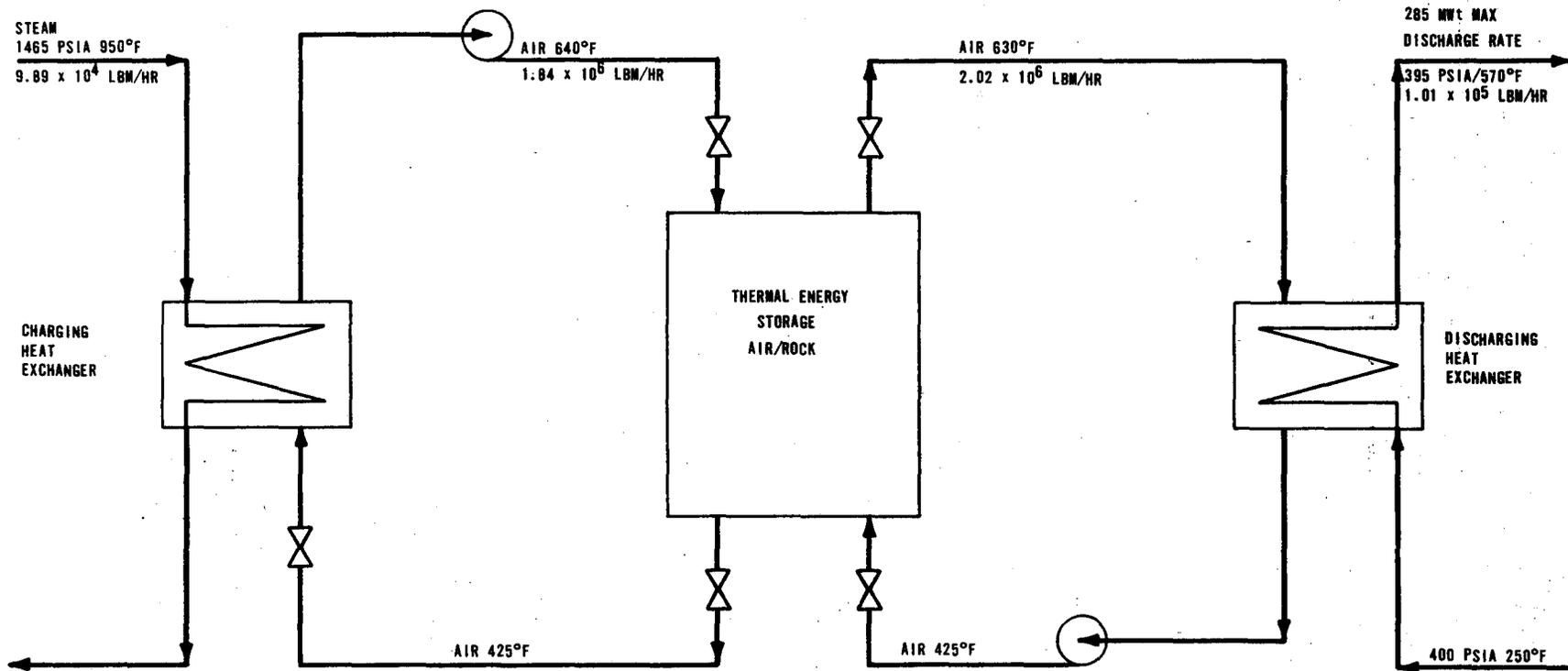
Figure 4-9. Air/Rock Tank-Heat Exchanger-Fan Arrangement —
