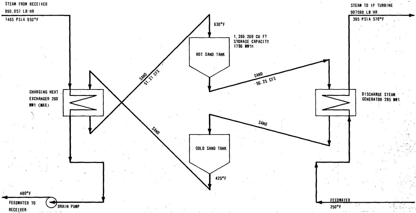
Figure 4-4. Moving Bed Temperature-Energy Diagram
