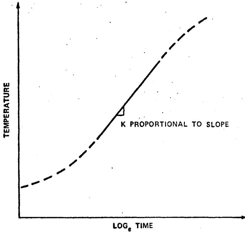
Figure E-2. Method for Determining Thermal Diffusivity Using Hot Wire Technique
