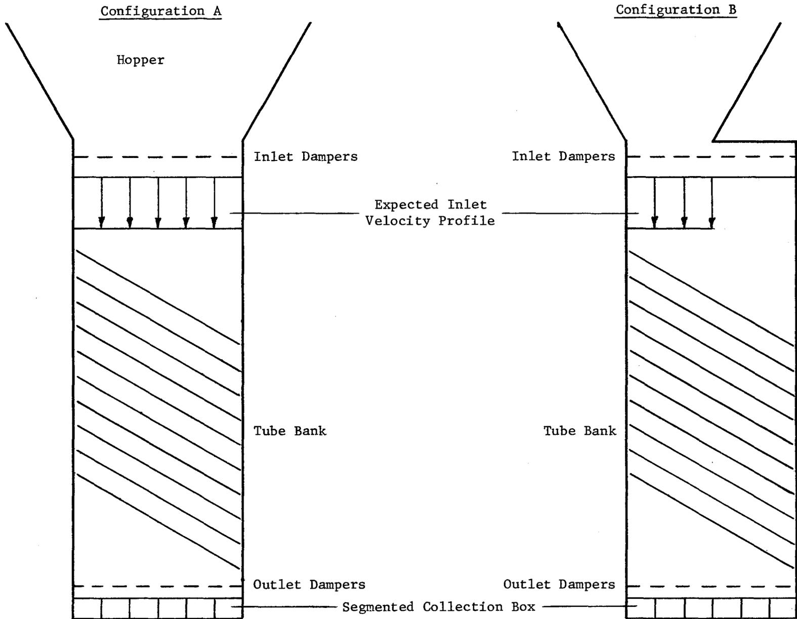
Figure 8-2. Heat Transfer Test Apparatus,
