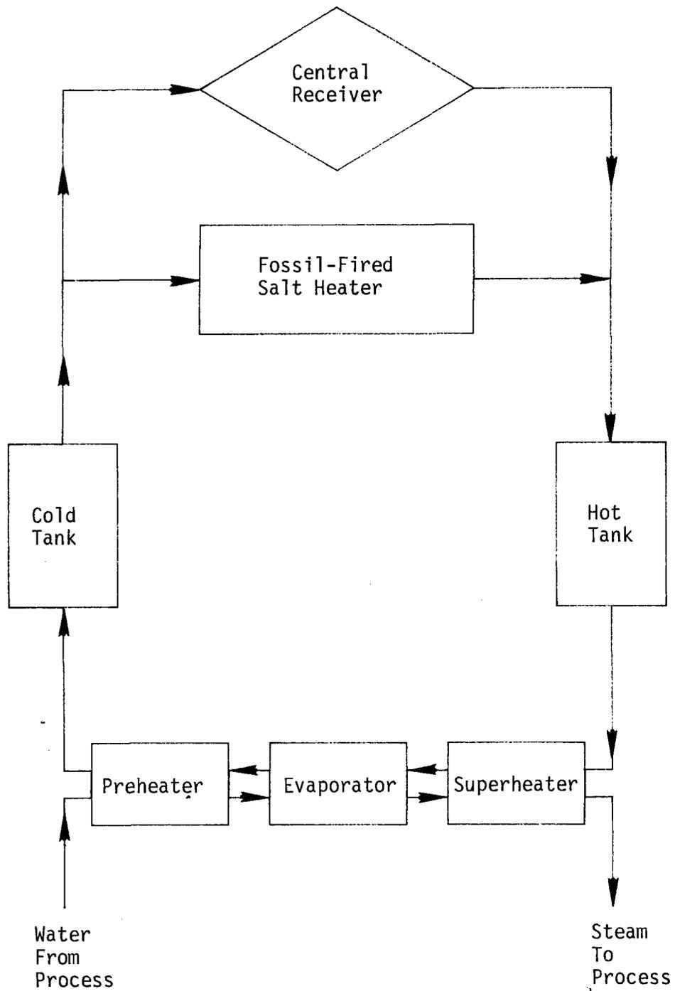
Figure 15. Molten Salt Receiver Based Hybrid System
