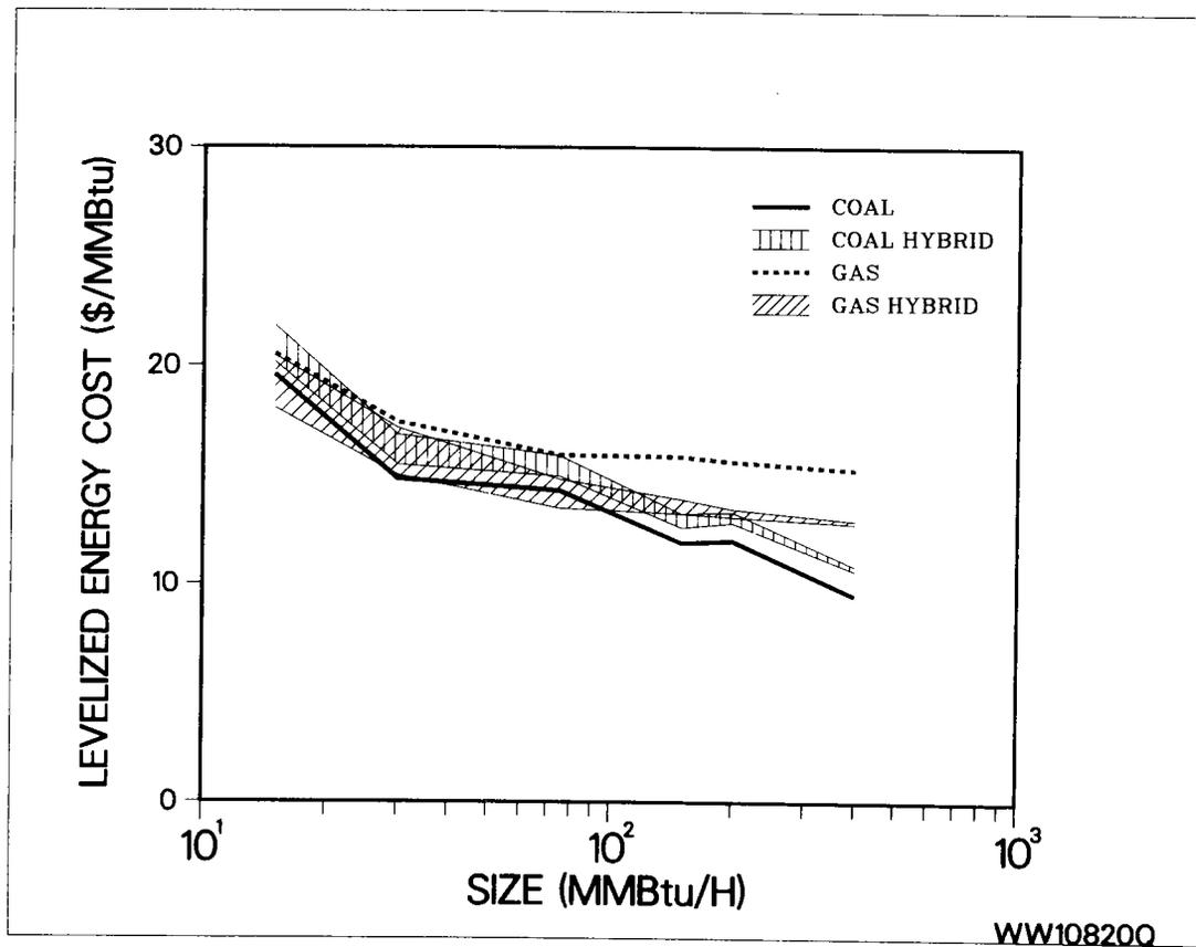
Figure 21c. LEC Curves Resulting from Adding 25% to O&M Costs of the Fossil Portion of the Plants
