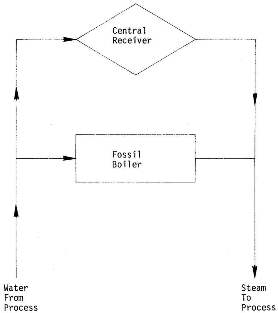
Figure 13. Water/Steam Receiver System
