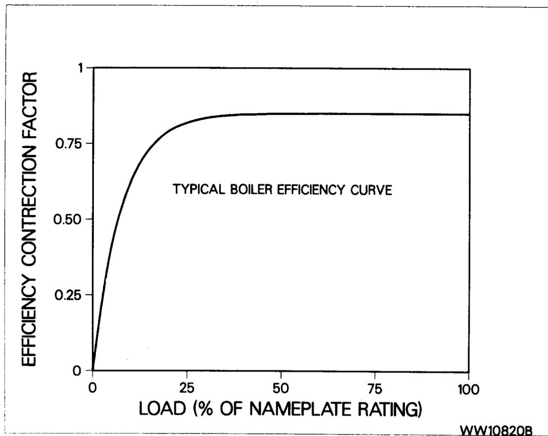
Figure 12. Boiler Efficiency Correction Curve
