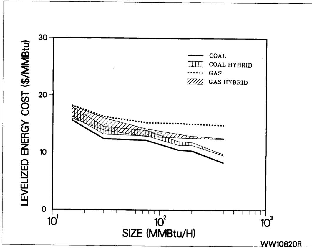
Figure 21d. LEC Curves Resulting from Reducing O&M Costs of the Fossil Portion of the Plants by 25%
