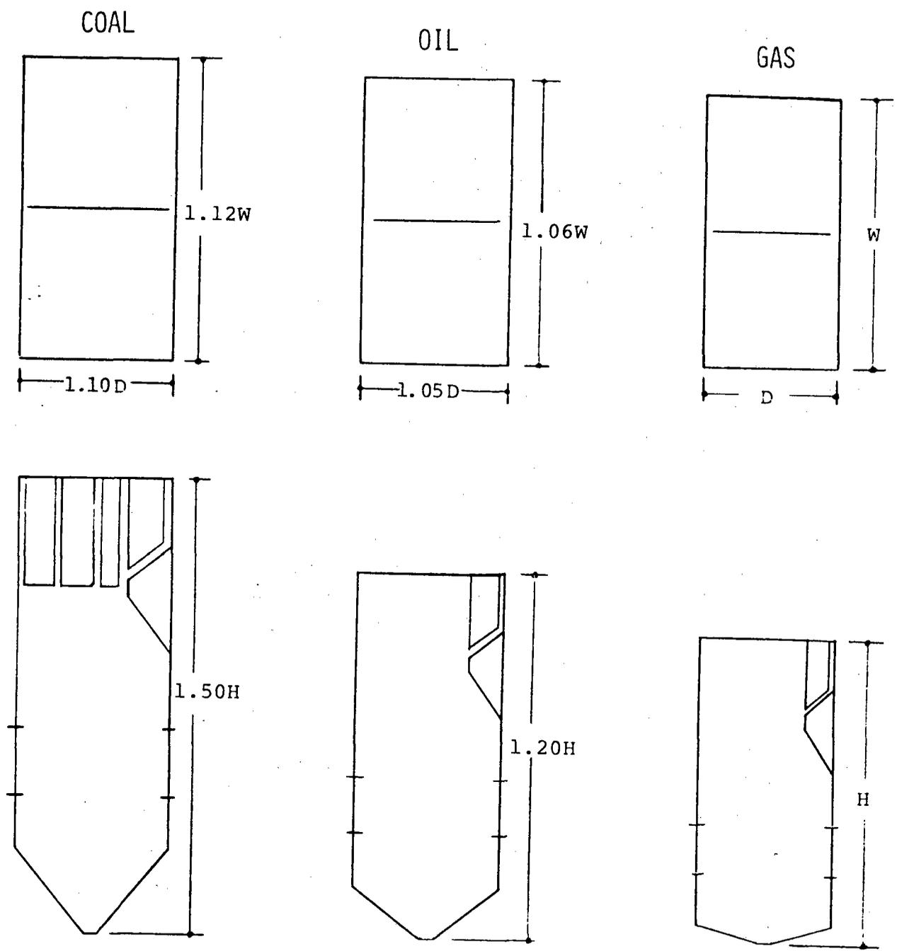
Figure 2. Relative Furnace Size for Boilers Designed for Coal, Oil and Natural Gas Fuel (From M. L. McKimney [17])
