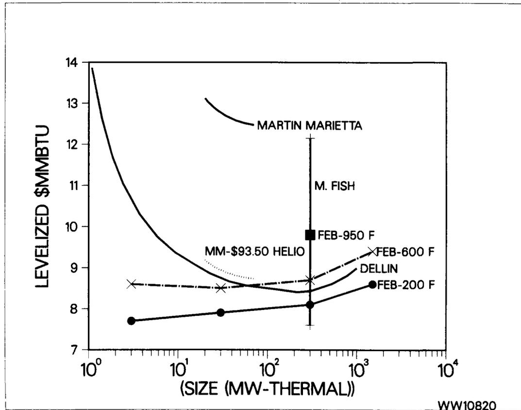
Figure 6. Cost of Energy at the Base of the Receiver Tower from a Number of Previous Studies: Martin Marietta Data from Ref. 38d; Dellin Data from Ref. 10; February Study Data from Ref. 9
