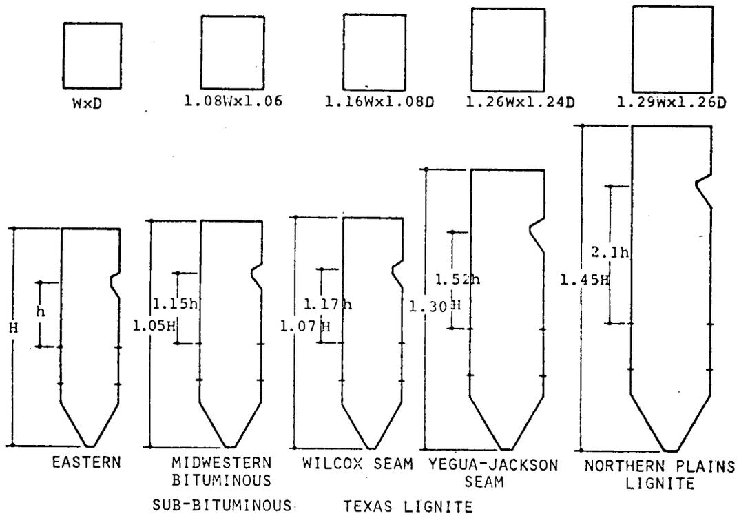
Figure 3. Effect of Coal Rank on Furnace Sizing
