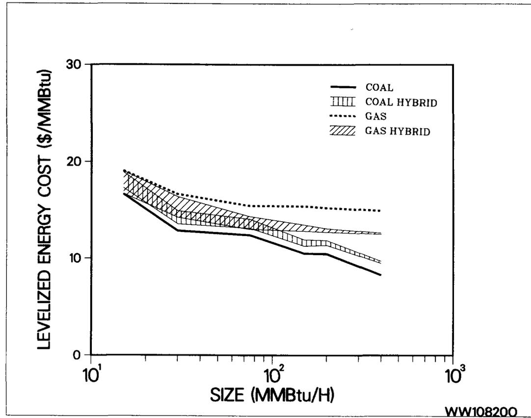
Figure 21b. Cost Curves Resulting from Subtracting 25% from Capital Costs of the Fossil Portion of the Plants
