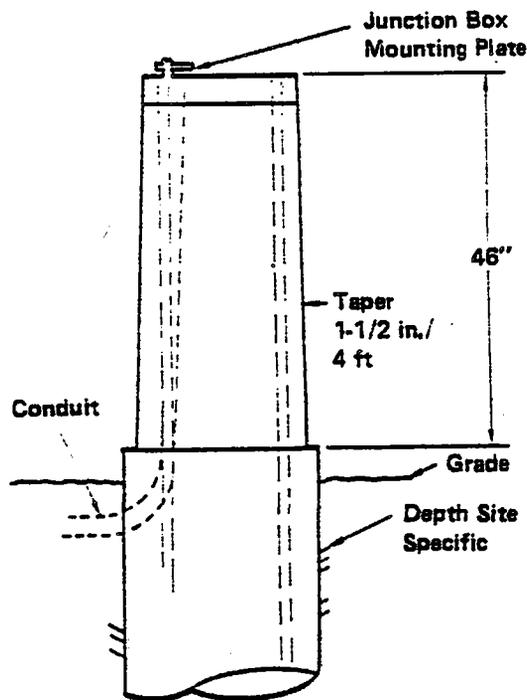
**Figure IV.C.4. Foundation Configuration**
