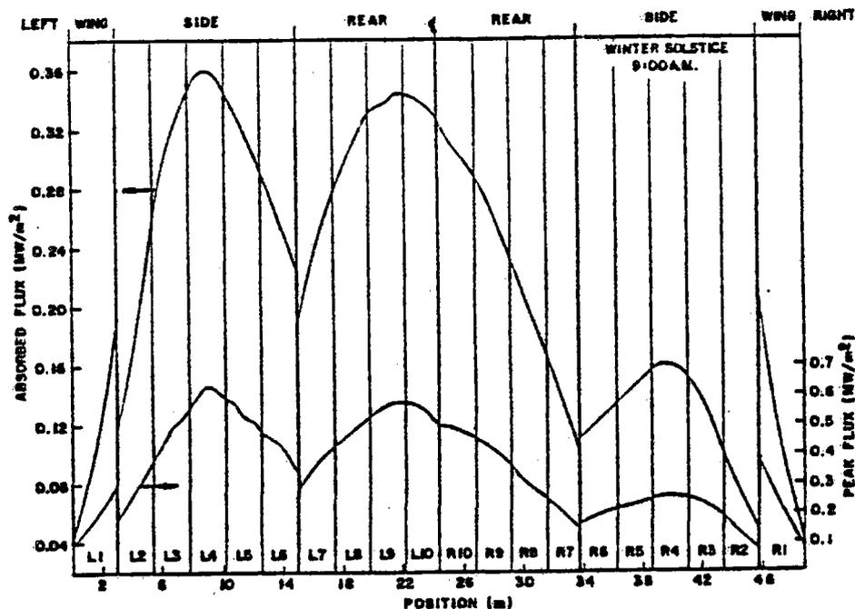
Figure IV.D.4. Winter Solstice Absorbed Flux Profile
