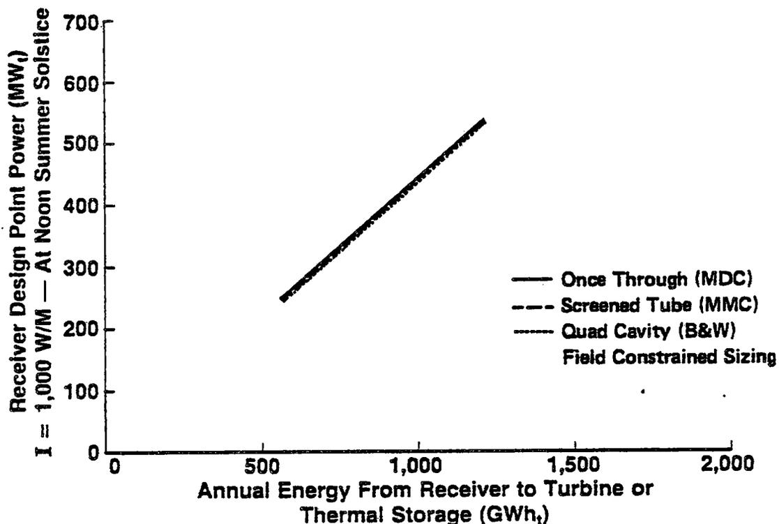
Figure III.B.4. Typical Delsol Results Comparison of Water/Steam Configurations
