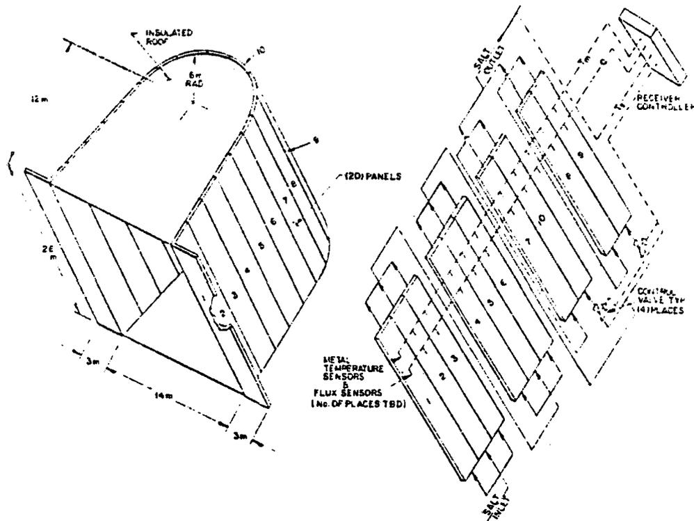
Figure IV.D.8. Receiver Panel Sensor Arrangement
