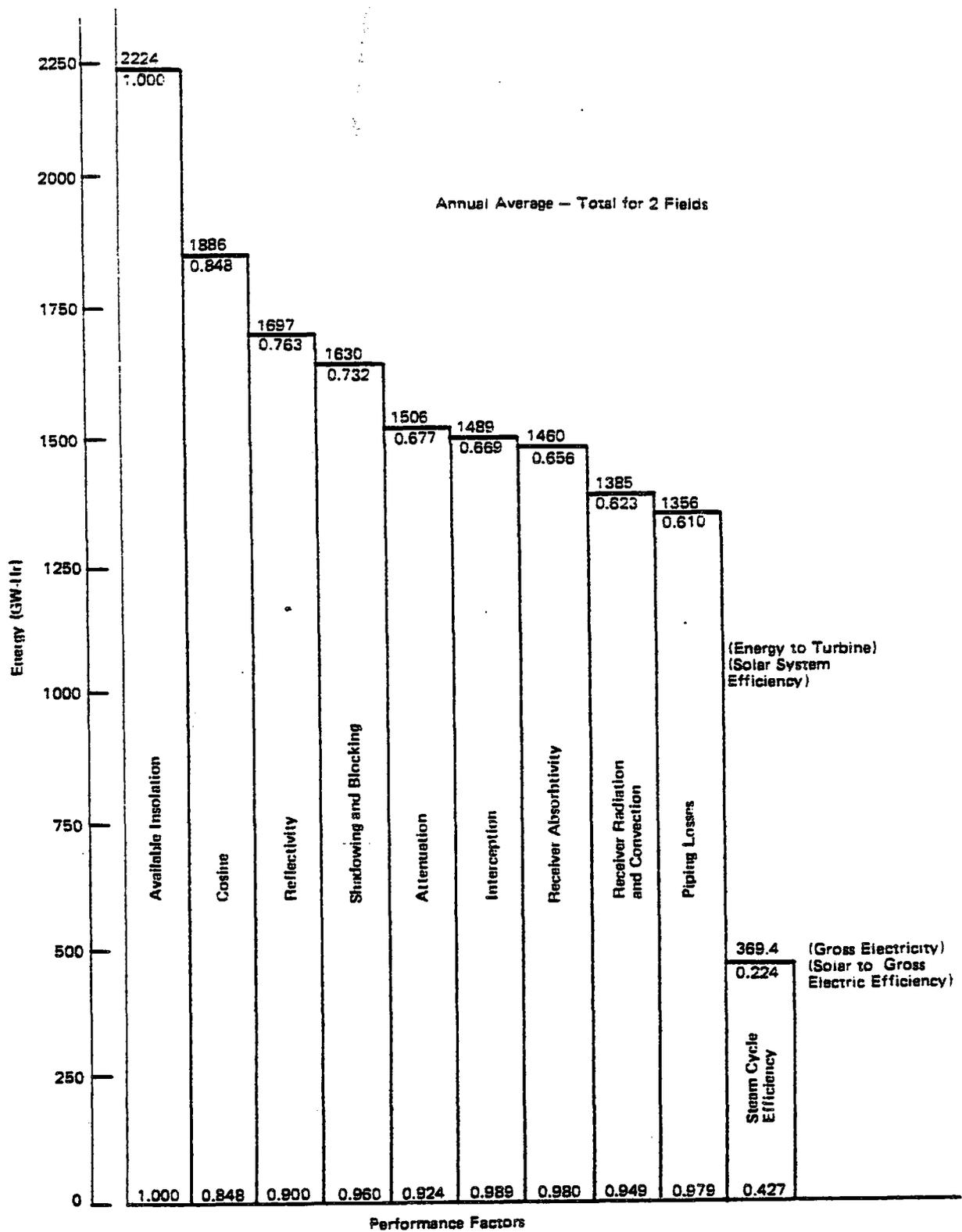
Figure III.C.15. Baseline Molten Salt System Performance
