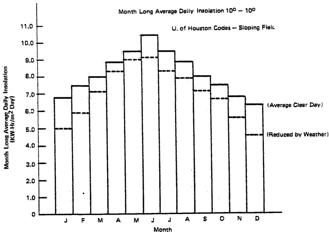
Figure V.A.6. Insolation Model for Final Performance Analysis
