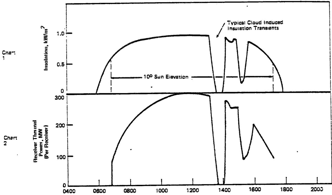
Figure IV.B.1(a). Typical Daily Operation Timeline
