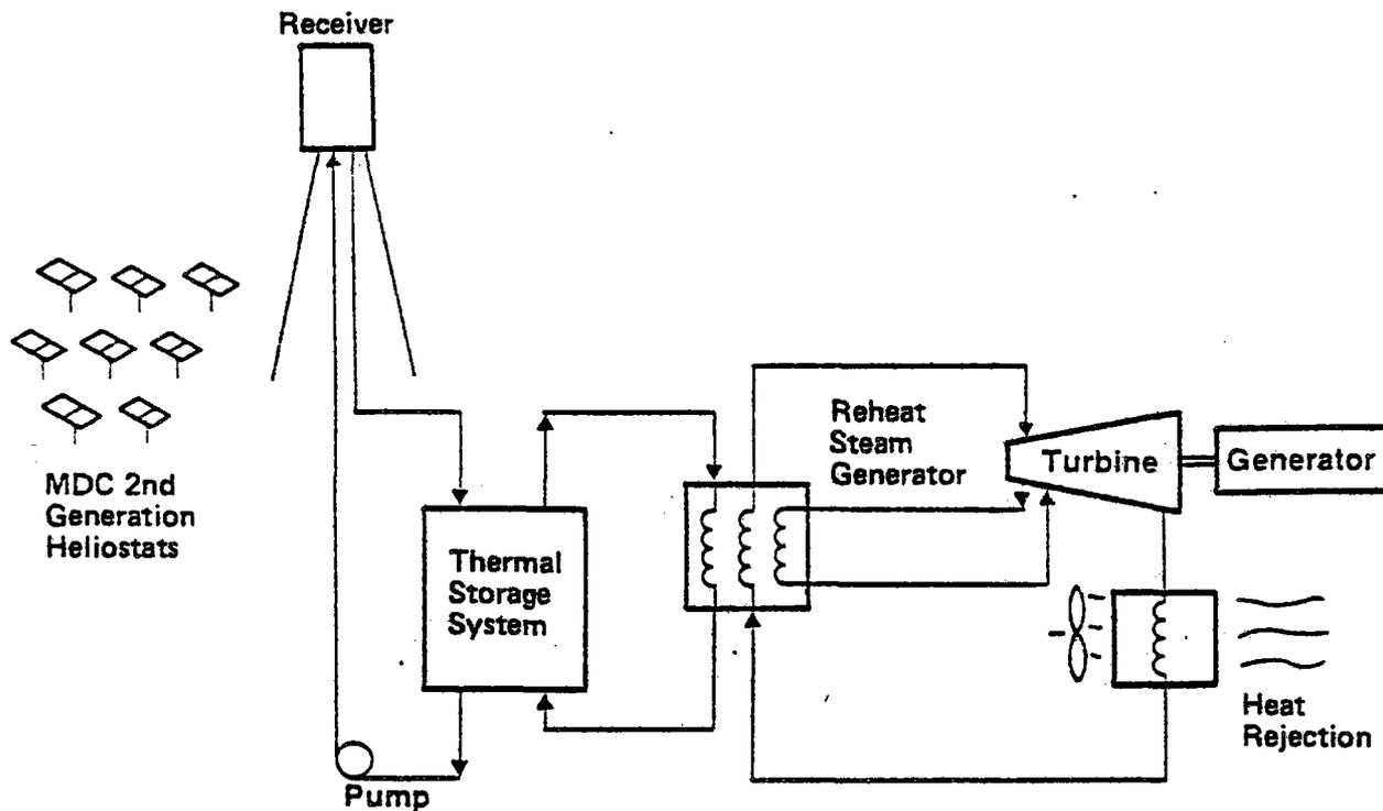
Figure III.D.1. Solar Central Receiver System – Liquid Sodium
