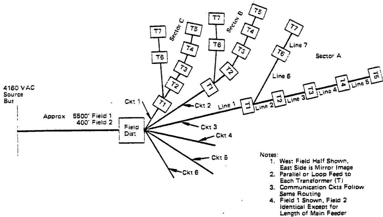
Figure IV.C.8. Electric Power Distribution Schematic
