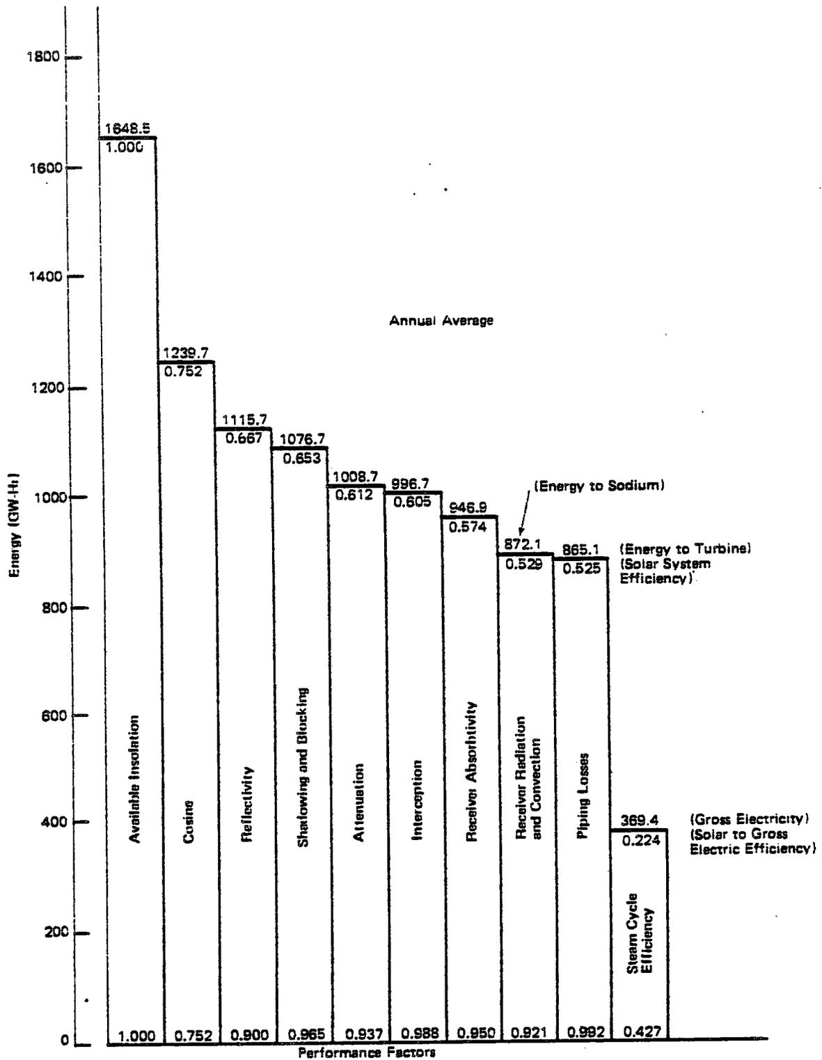
Figure III.D.9. Baseline Sodium System Performance
