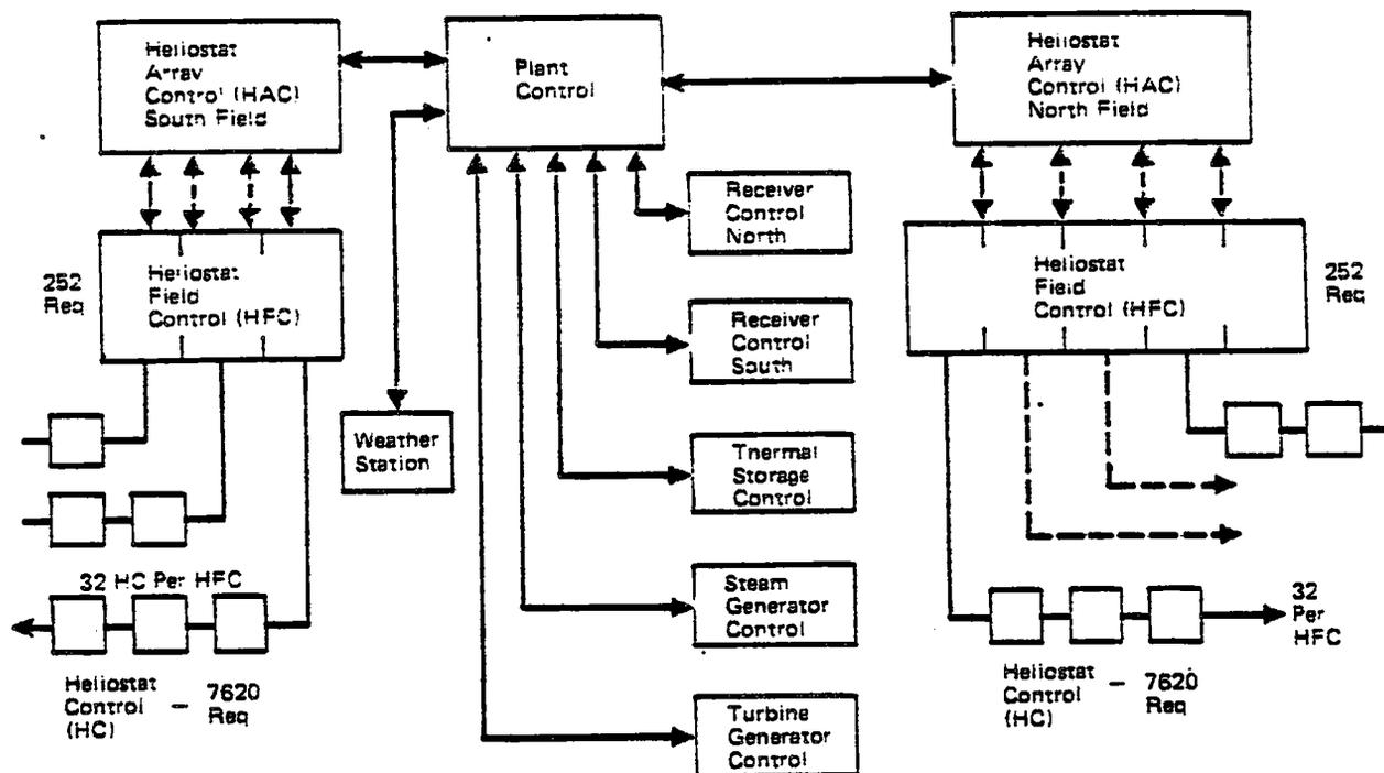
Figure III.C.13. Plant Control System – Molten Salt Configuration
