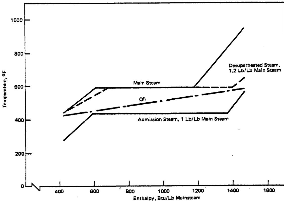
Figure III.B.7(a). Pinch Point Diagram of Single Stage Storage Unit
