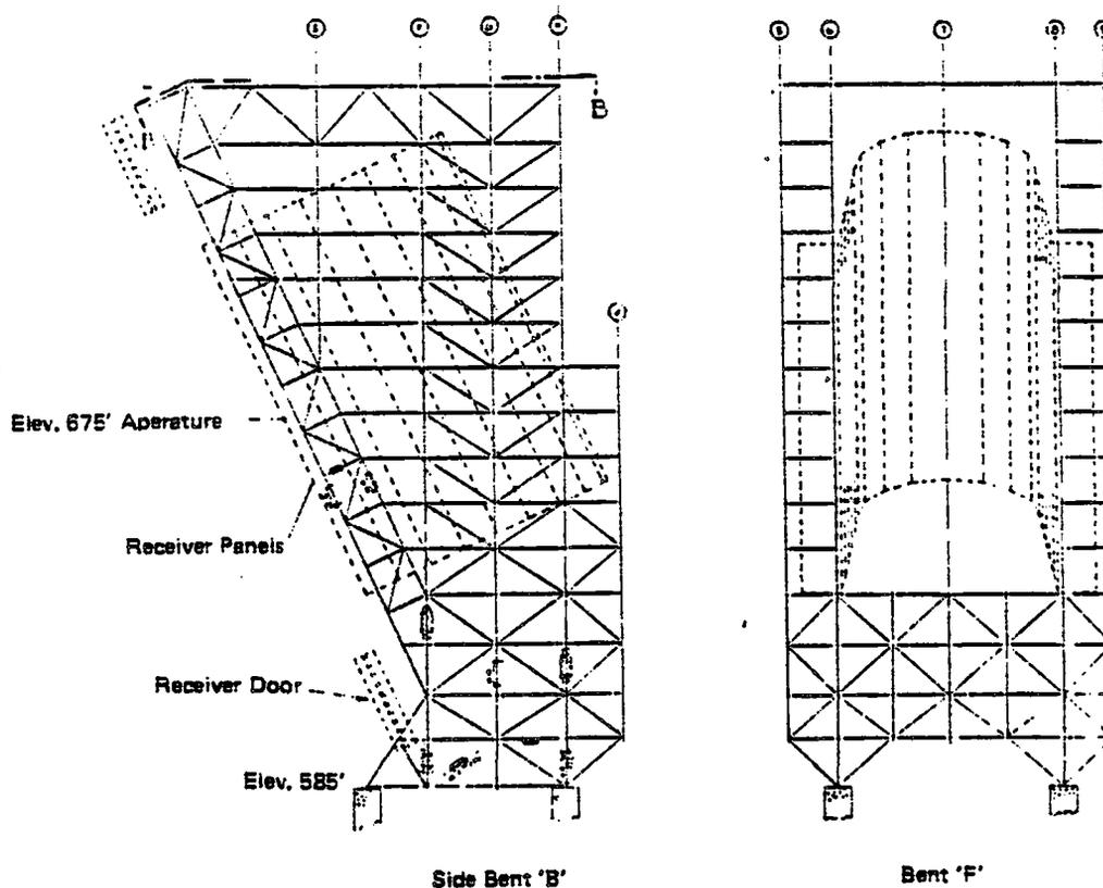
Figure IV.D.1. Receiver Support Structure
