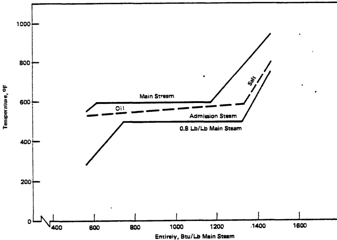
Figure III.B.7(b). Pinch Point Diagram for Two Stage Storage
