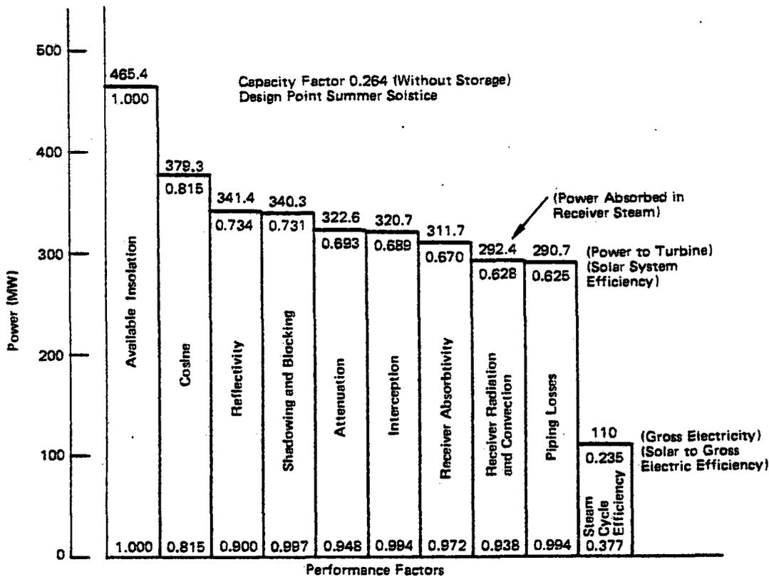
Figure III.B.14. Baseline Water/Steam System Performance
