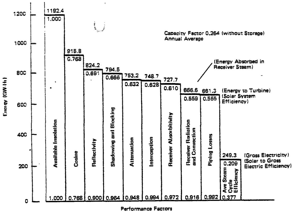
Figure III.B.15. Baseline Water/Steam System Performance
