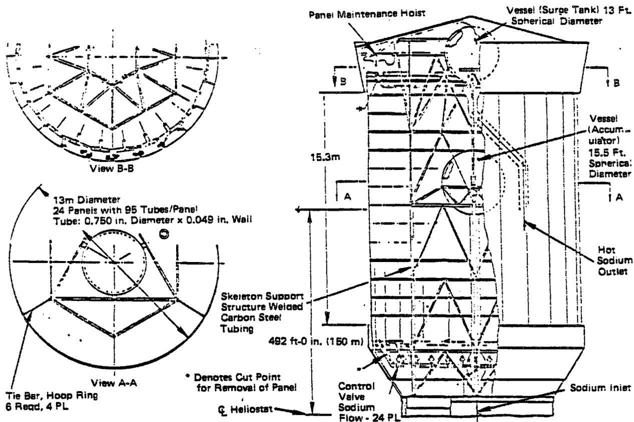
Figure III.D.6. Sodium Receiver General Arrangement
