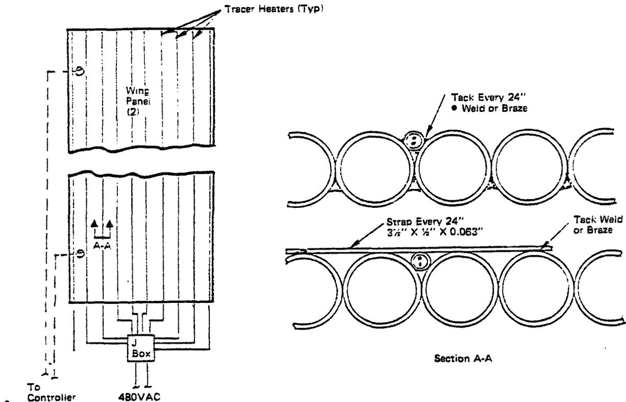
Figure IV.D.10. Panel Heater Configuration – Wing Panels Only
