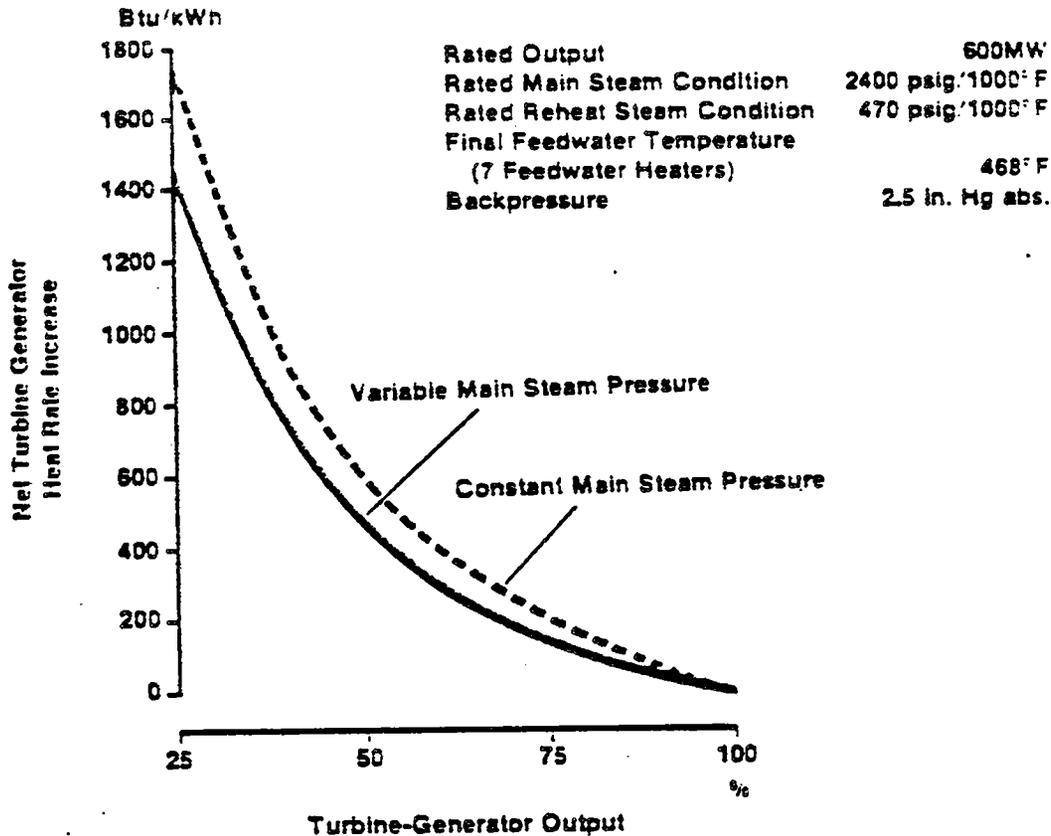
Figure IV.H.1. Net Heat Rate Differentials for Full-Arc Admission Turbines
