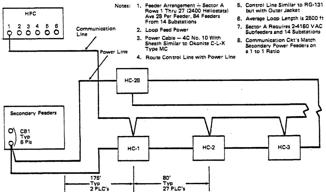
Figure IV.C.9. Electric Power Distribution Sector Layout
