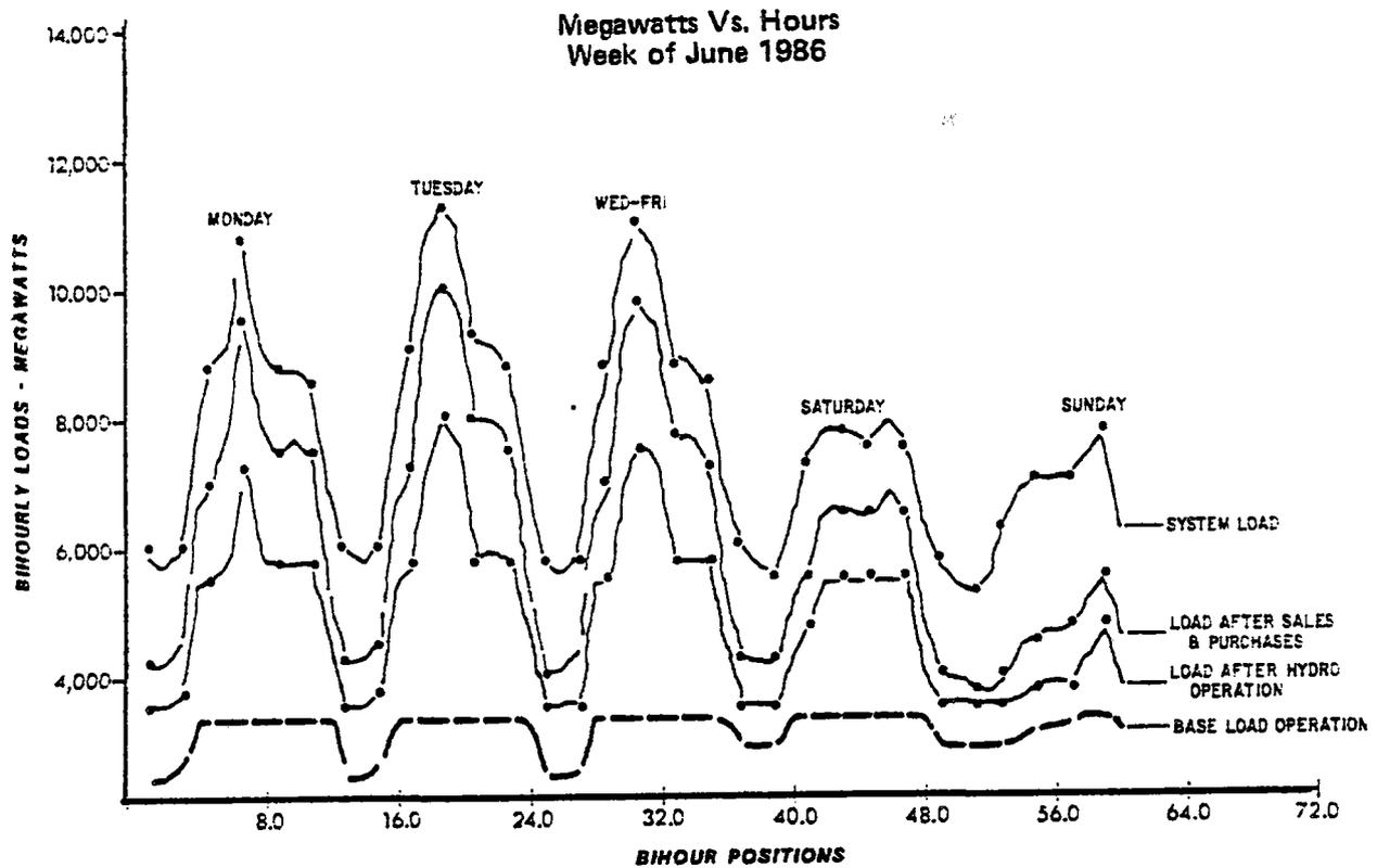
Figure III.E.1. System Simulation Results – Weekly Load Curve
