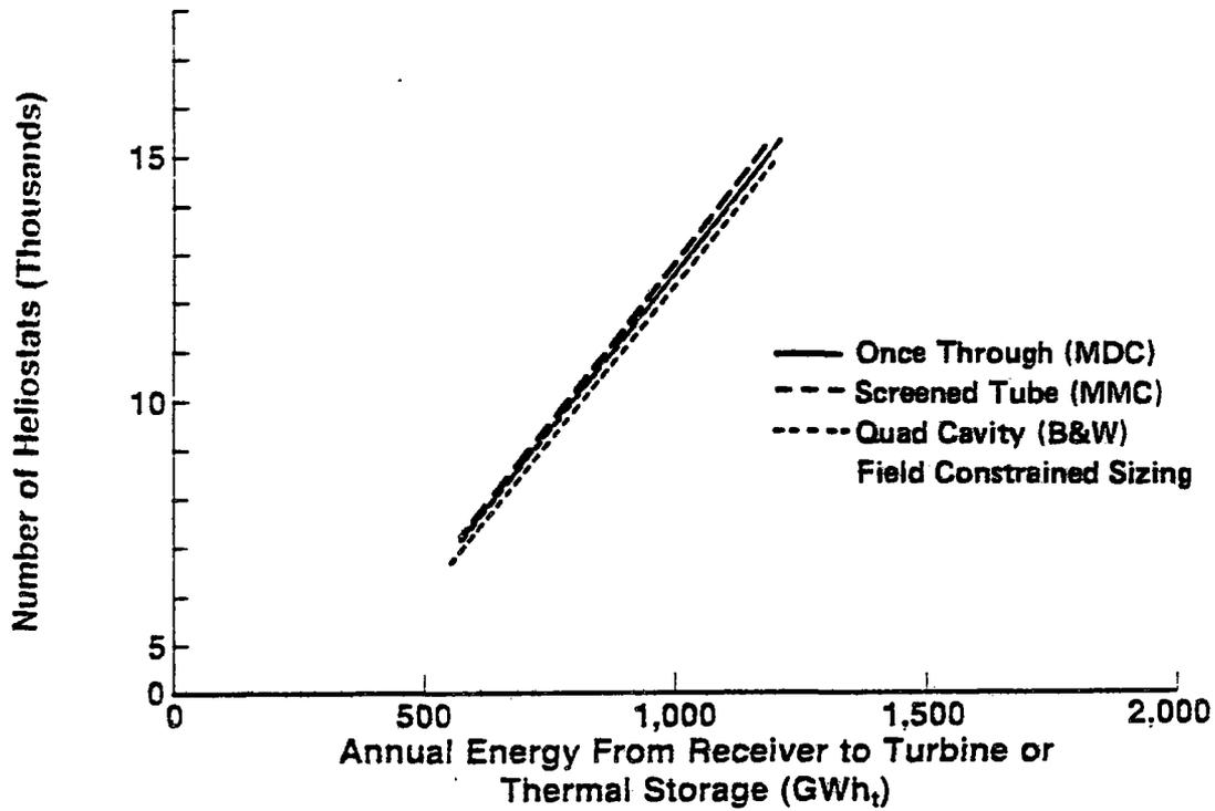
Figure III.B.5. Typical Delsol Results Comparison of Water/Steam Configurations
