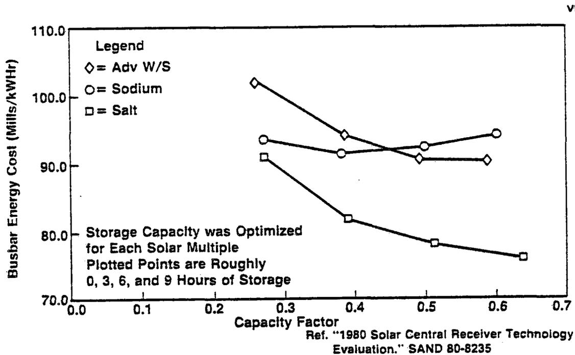
Figure III.A.2. Busbar Electricity Cost as a Function of Capacity Factor for Solar Central Receiver Technologies
