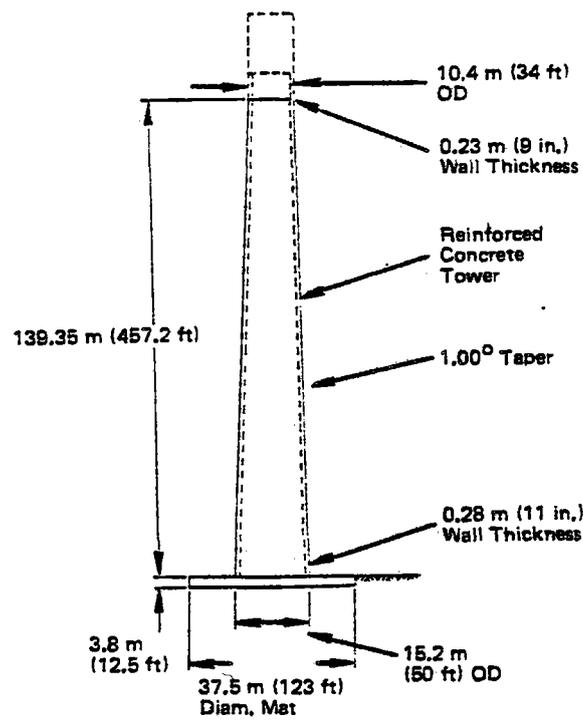
Figure III.D.5. Sodium Receiver Tower
