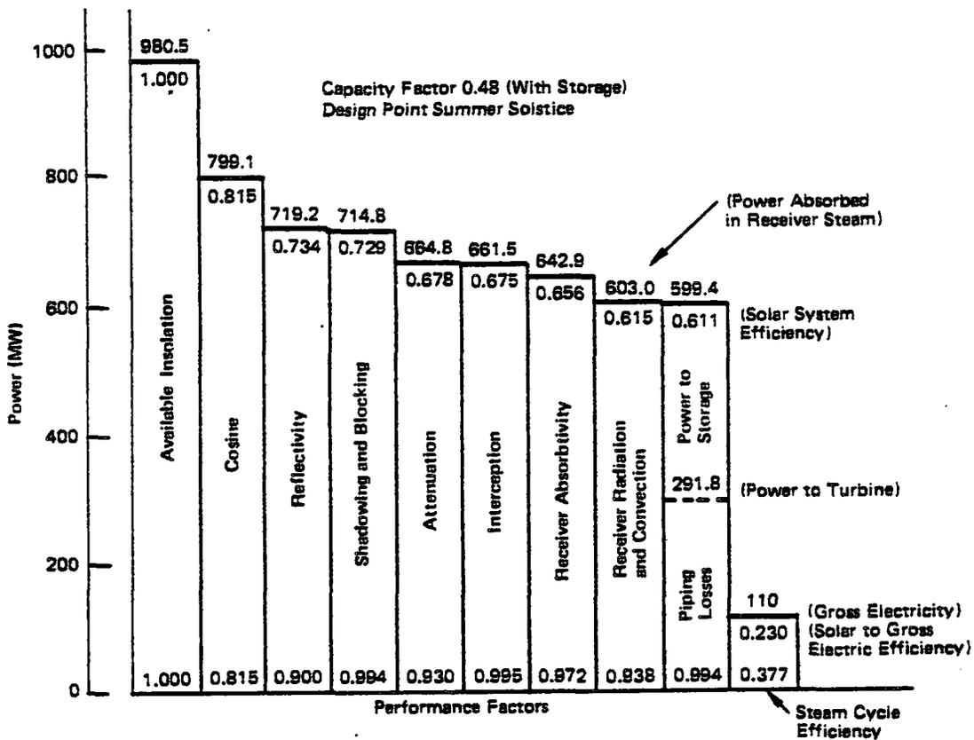
Figure III.B.16. Baseline Water/Steam System Performance
