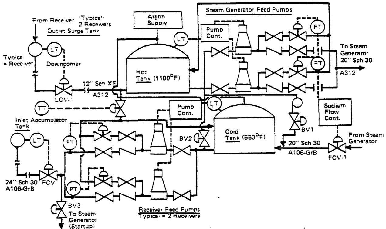
Figure III.D.7. Sodium Storage and Transport System Schematic
