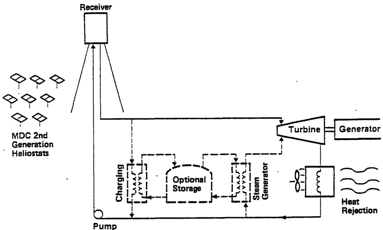
Figure III B-1 Solar Central Receiver System - Water Steam
