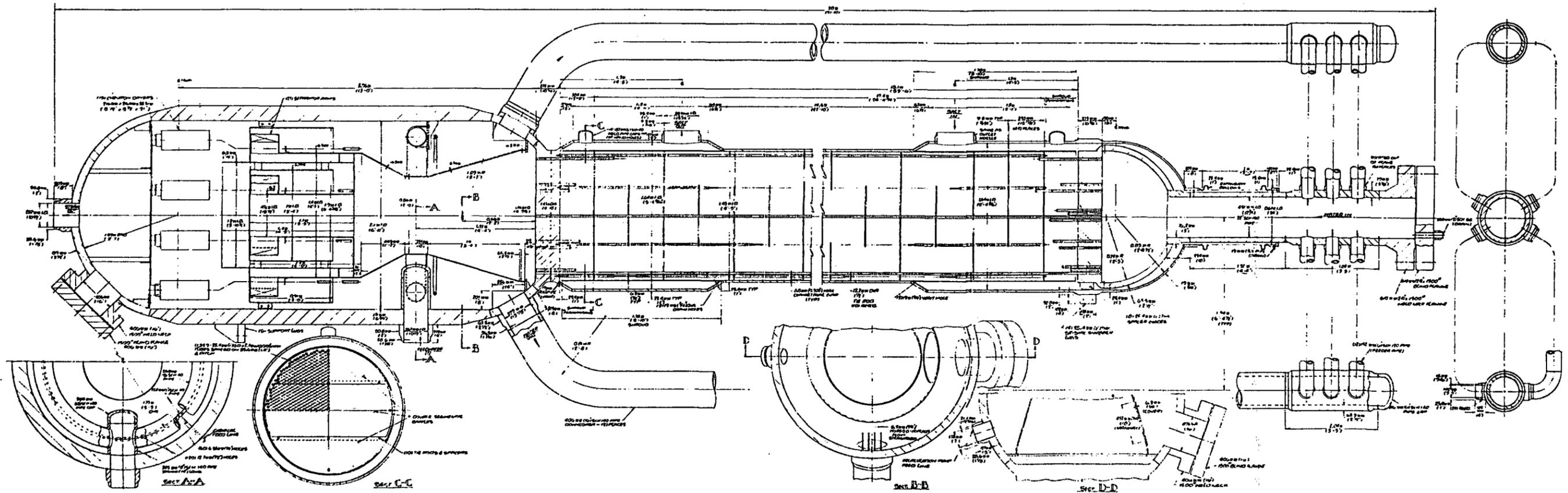
Figure IV. G. 2. Salt Evaporator Heat Exchanger
