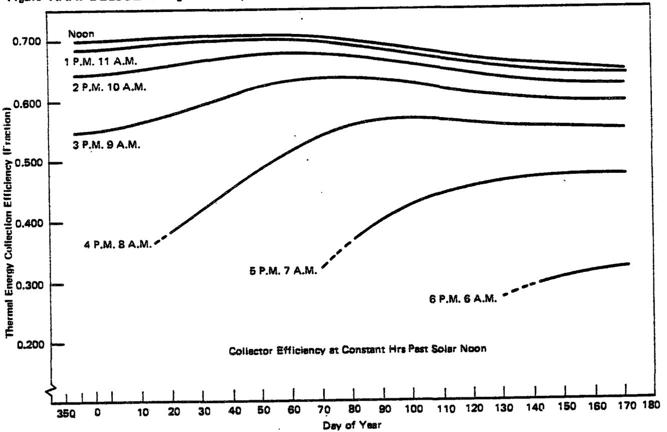
Figure V.A.5. Conversion Efficiency from Insolation to Thermal Energy
