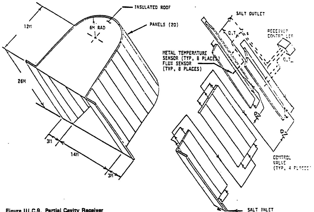
Figure III.C.9. Partial Cavity Receiver
