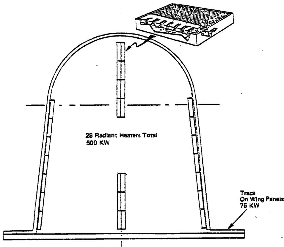
Figure IV.D.9. Heater Panel Layout - Plan View
