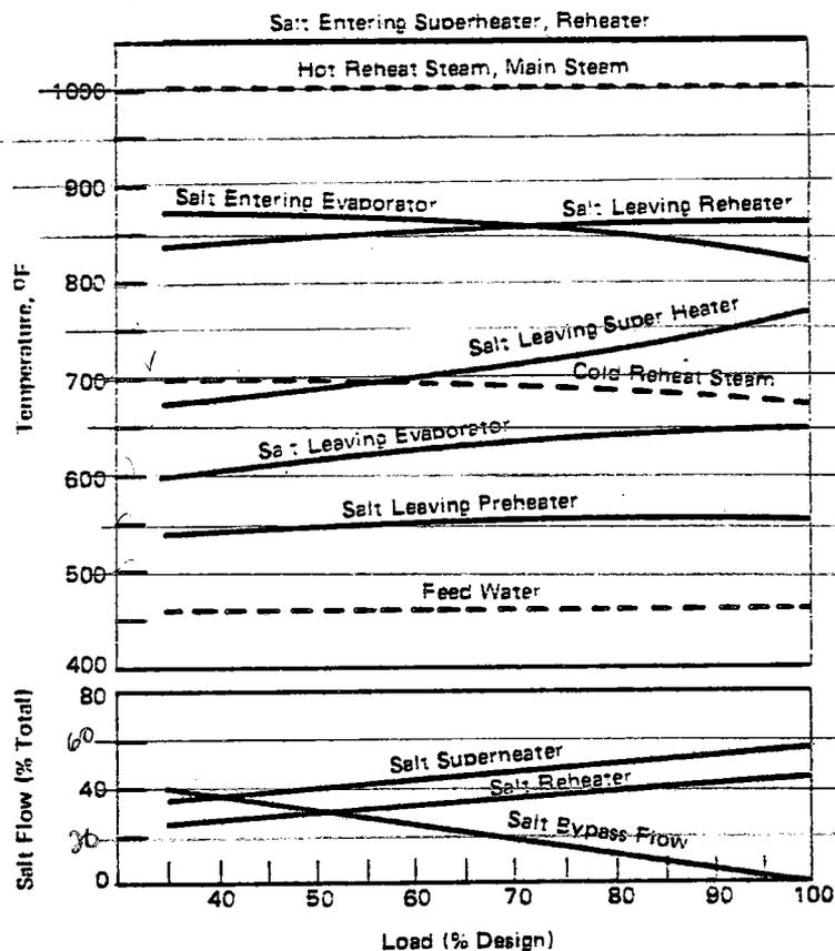
Figure IV.G.12. State Point Variation with Load at Sliding Pressure
