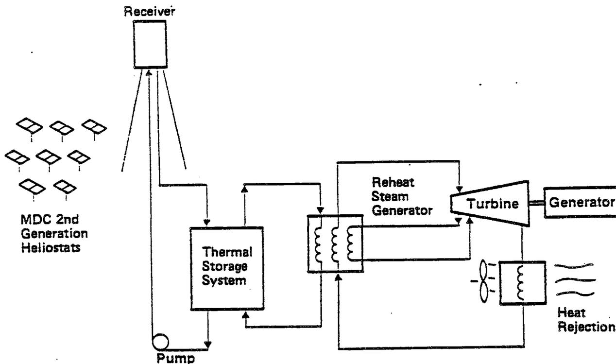
Figure III C-1. Solar Central Receiver System - Molten Salt
