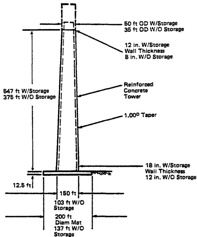
Figure III.B.9. Receiver Tower
