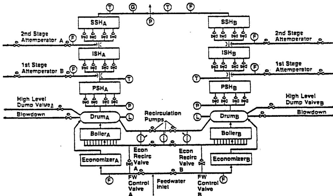
Figure III.B.11. Water/Steam Receiver Schematic
