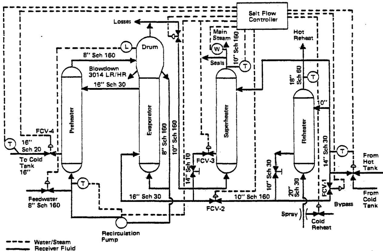
Figure III.C.12. Steam Generator System Schematic
