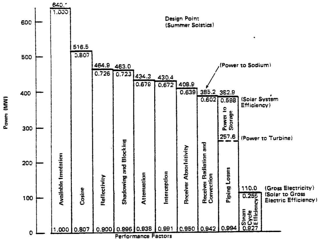
Figure III.D.8. Baseline Sodium System Performance
