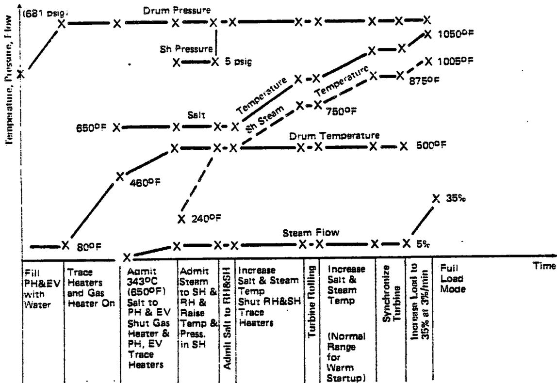
Figure IV.G.11. Cold Start-Up - 100-MWe Solar Stand-Alone SGS
