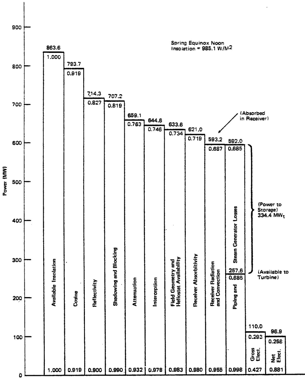
Figure V.D.3. Spring Equinox Noon Performance
