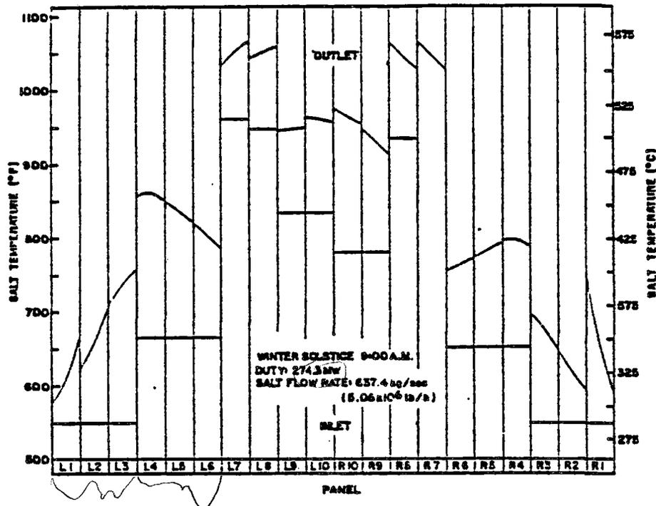
Figure IV.D.5. Winter Solstice Salt Temperature Profile
