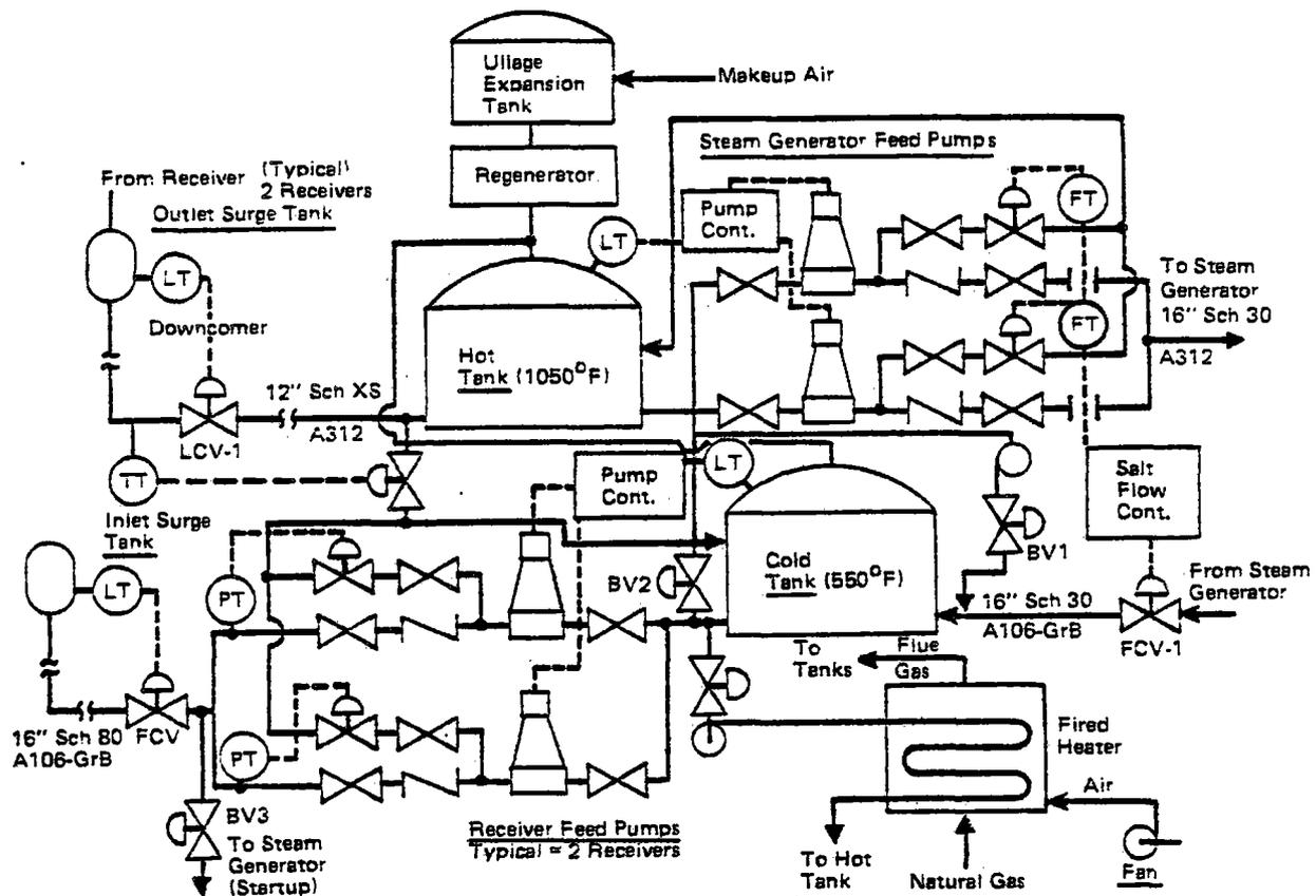
Figure III.C.10. Storage and Transport System Schematic
