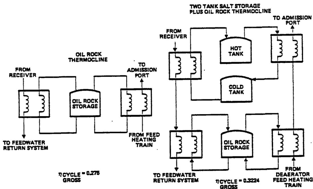
Figure III.B.3. Candidate Water/Steam Storage Systems
