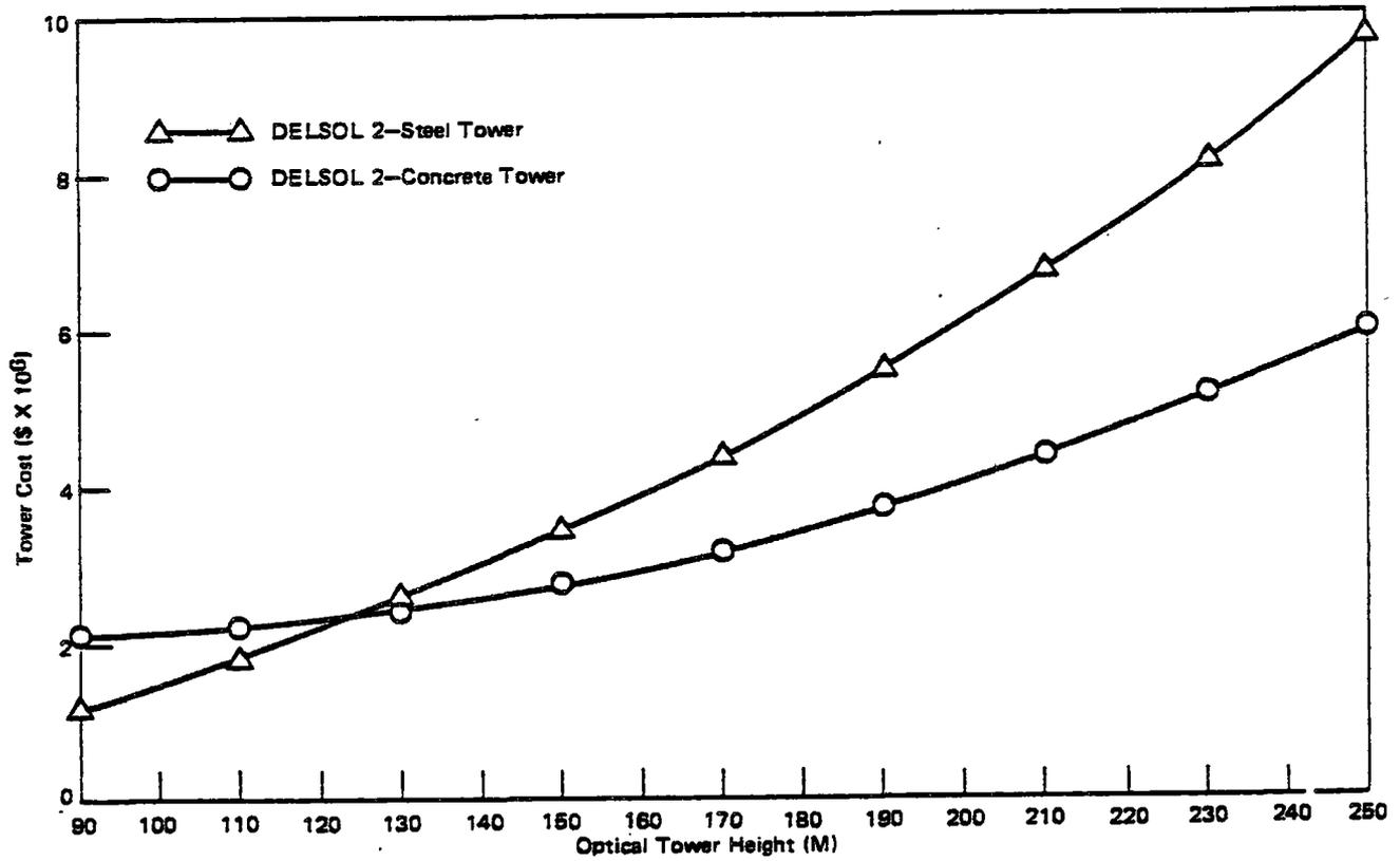
Figure III.C.6. Tower Cost Models
