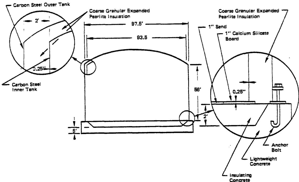
Figure III.B.13. Thermal Storage Tank
