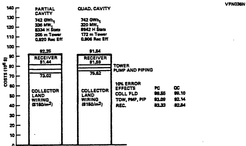
Figure III.C.4. Molten Salt Receiver Cost Breakdown Comparison
