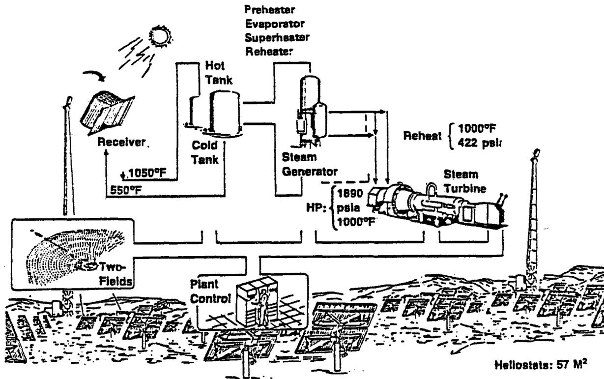
Figure II.G.1. 100 MWe Solar Central Receiver Plant
