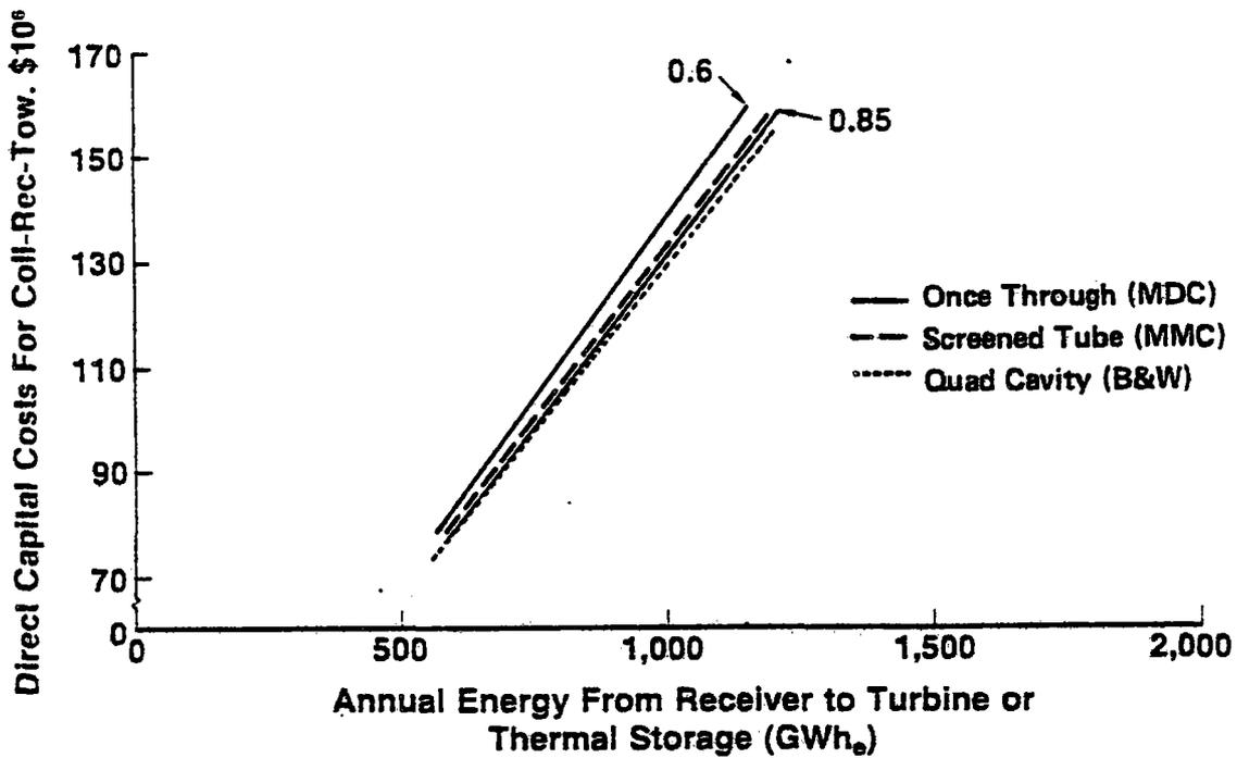
Figure III.B.6. Typical Delsol Results Comparison of Water/Steam Configurations
