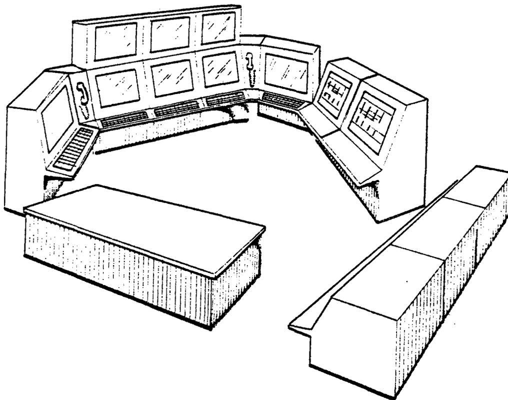
Figure IV.J.5. Integrated Control Console Layout
