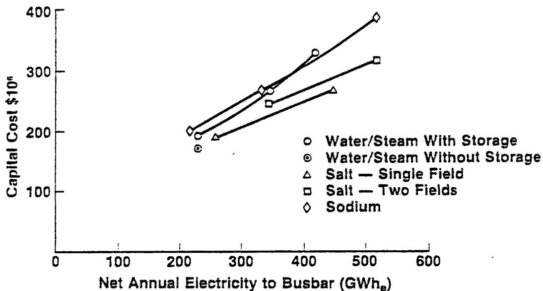
Figure III.F.1. System Costs Vs Net Annual Electricity Produced
