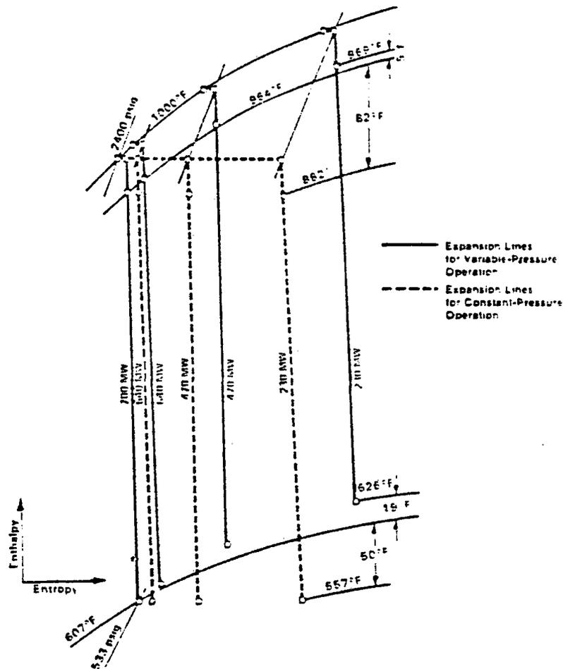
Figure IV.H.2. Comparison of Effect of Variable and Constant-Pressure Operation on the Steam Temperature Variations
