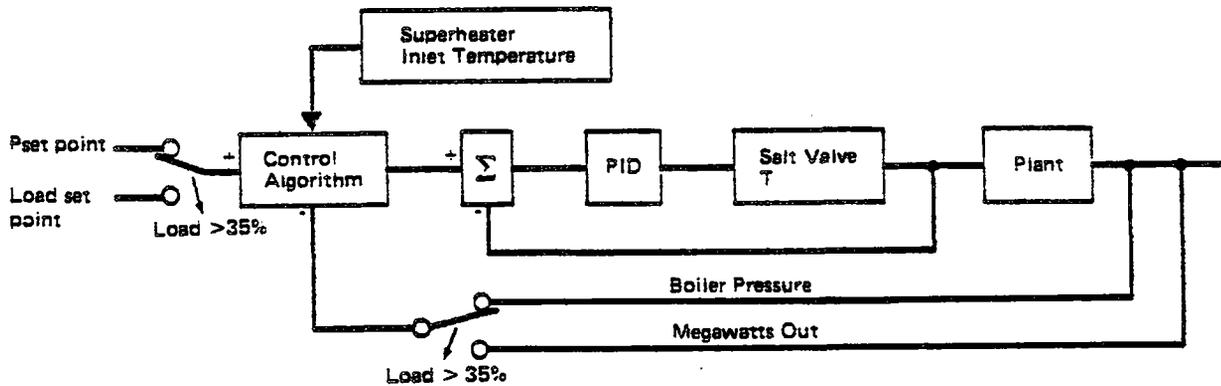
Figure IV.G.9. Boiler Control
