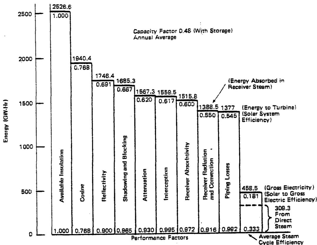
Figure III.B.17. Baseline Water/Steam System Performance
