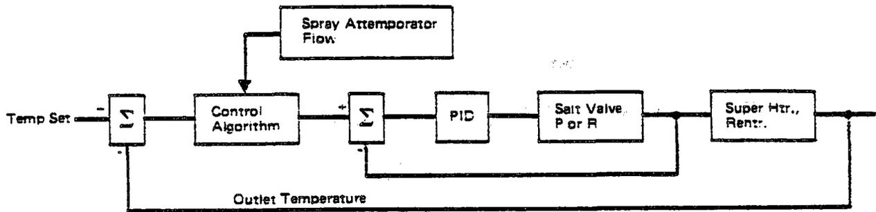
Figure IV.G.8. Superheater, Reheater Temperature Control
