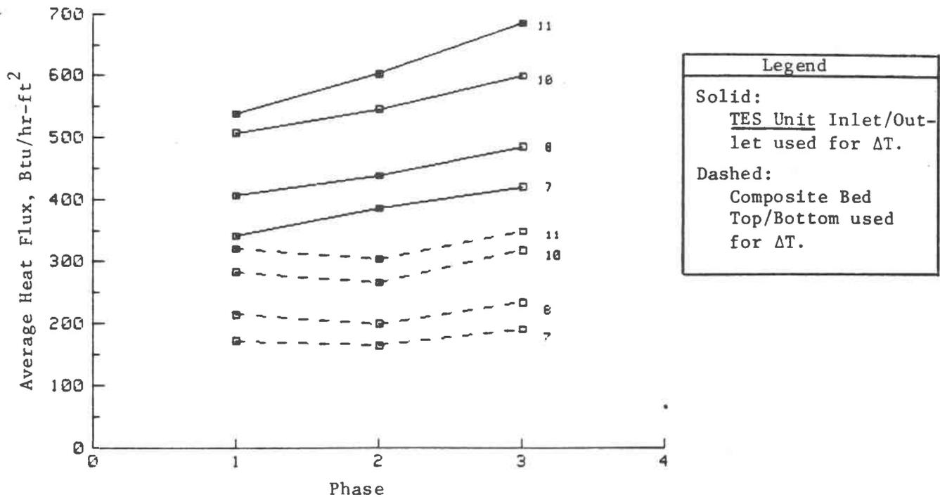
Figure 3. MEAN, EXPERIMENTAL DISCHARGE HEAT FLUXES FOR 51 WT % Na<sub>2</sub>CO<sub>3</sub>-BaCO<sub>3</sub>/ 49 WT % MgO FOR PHASE I, II and III
