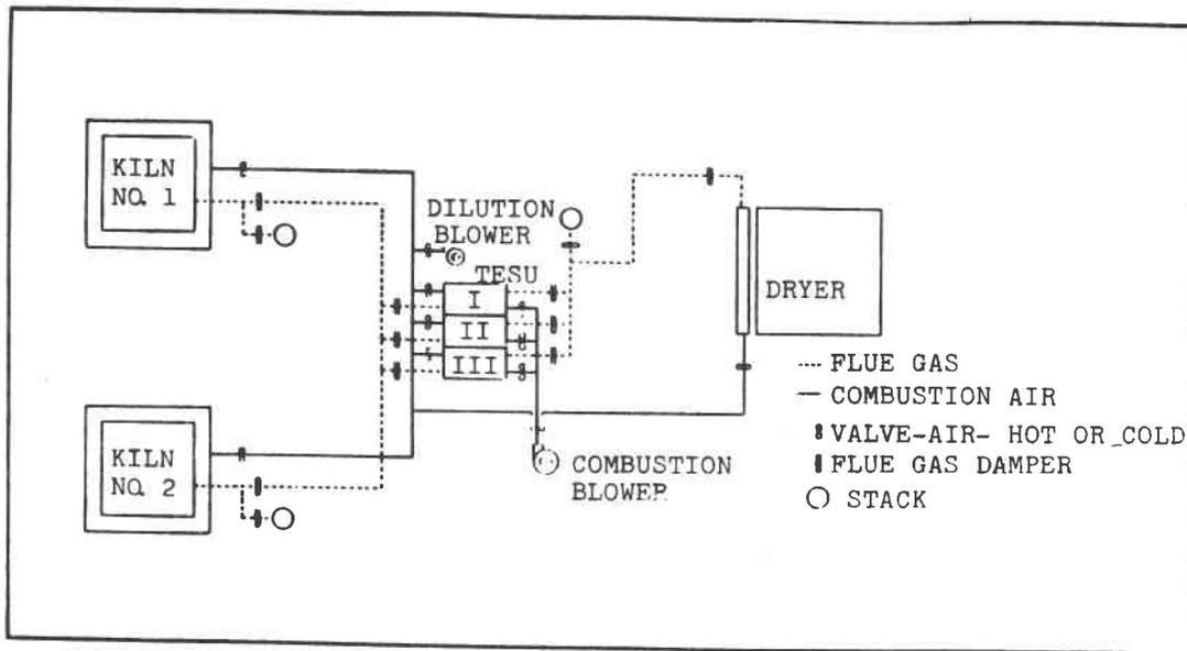
Figure 6. SCHEMATIC OF TES SYSTEM IN PERIODIC KILN APPLICATION
