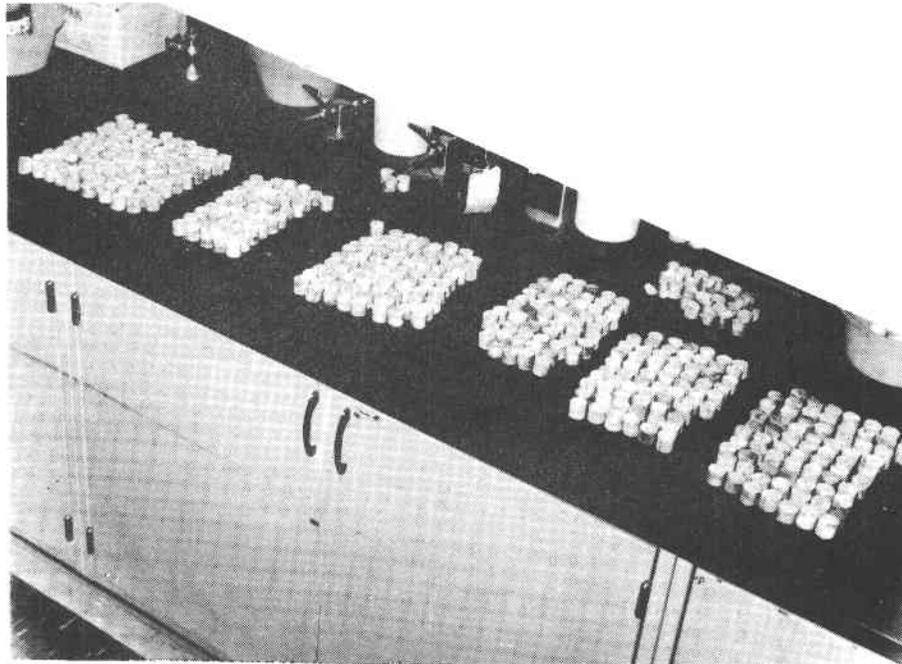
Figure 2. BENCH-SCALE POST-TEST CompPhase™ MEDIA AFTER 6060 HOURS AND 200 THERMAL CYCLES FROM 780° TO 400°C
