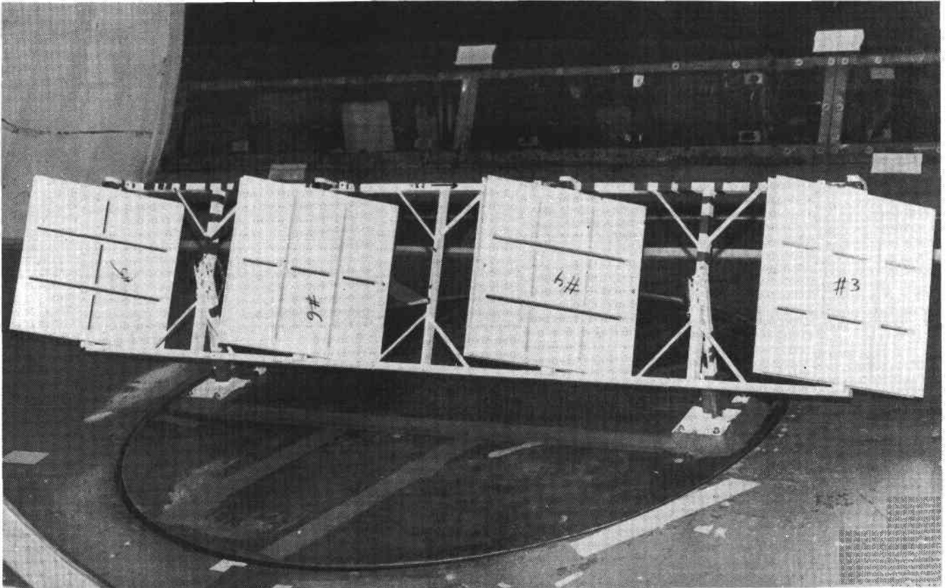
FIGURE 2-17. 1/10 SCALE MODEL WITH VENTED MIRROR MODULES IN WIND TUNNEL
