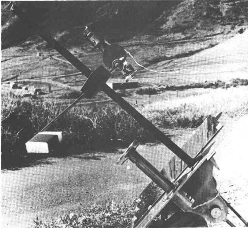
Figure B-15 Specular Reflectivity Test Rig Using Normal-Incidence Pyrheliometers, Profile View
