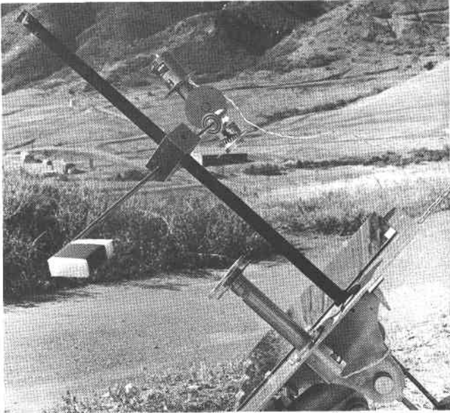
Figure II-I-1 Specular Reflectivity Test Rig Using Normal-Incidence Pyrheliometers, Profile View
