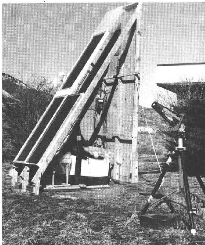
Figure II-10 Improved Collector Test Setup
