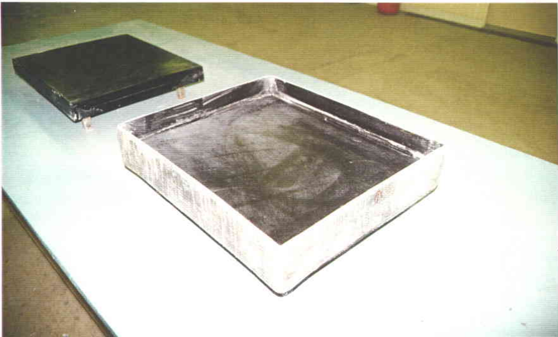
20" x 24" Segment: Female Mold Section with Flange Ring
