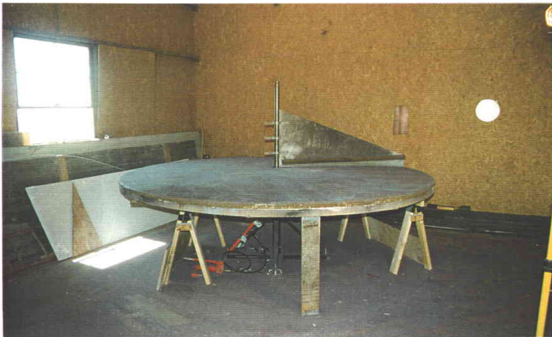
3-Meter Mold Showing Support Structure and Screed Apparatus
