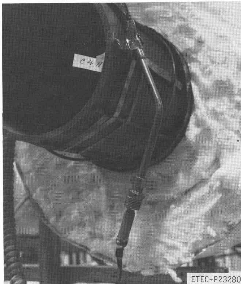
Figure 25. Typical Orientation of a Typical Heater Mounting on a Prototype Pipe
