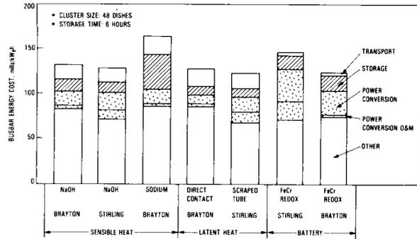
Figure 6. Comparison of Multi-Dish/Thermal Storage with Dish-Battery Systems
