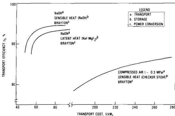
Figure 4. Transport System Performance and Cost Characteristics
