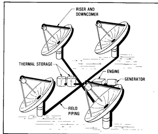
Figure 1. Multi-Dish Cluster/Thermal Storage Power Module
