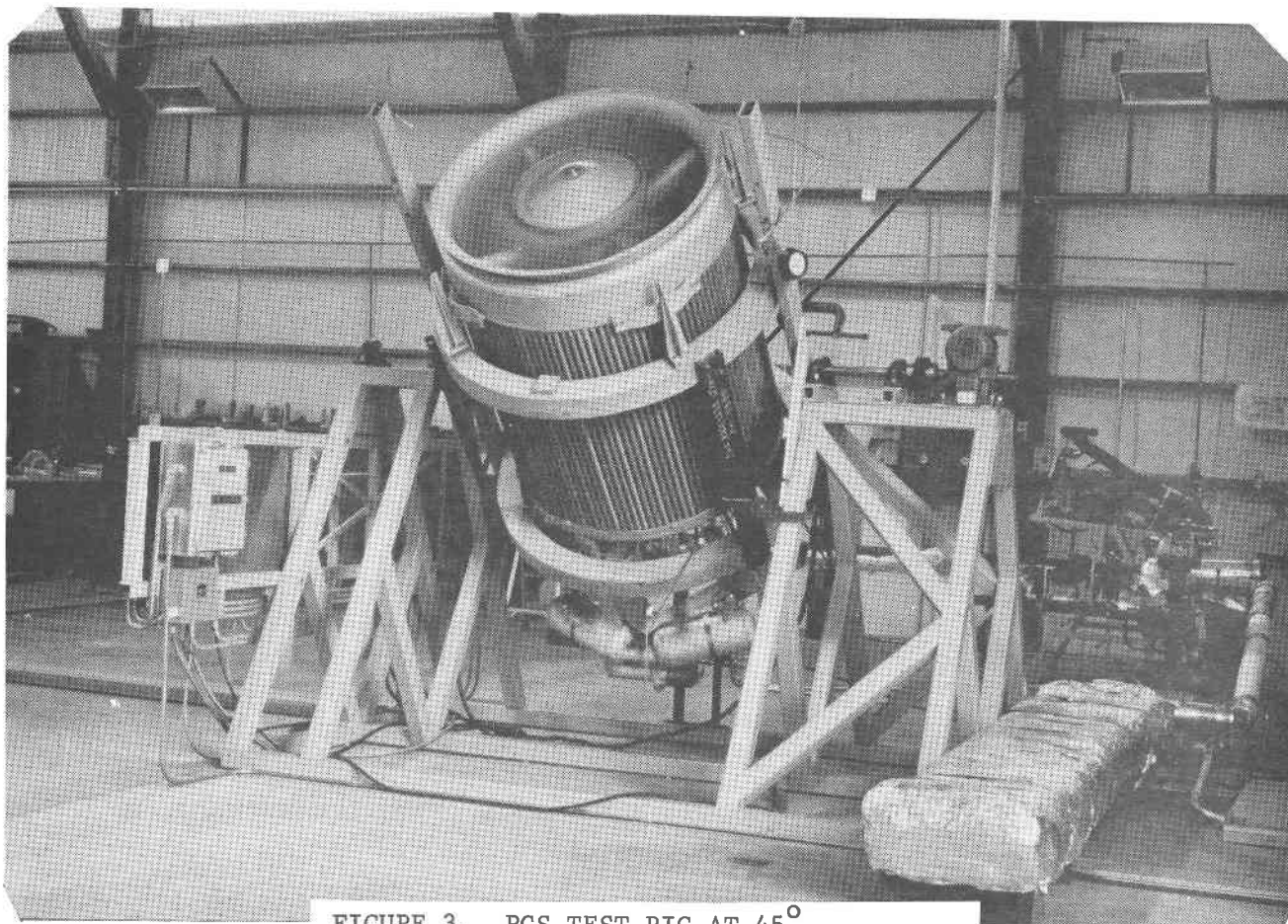
FIGURE 3. PCS TEST RIG AT 45° ELEVATION ANGLE
