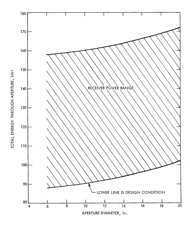
Figure 1. Concentrator Thermal Output Required for Various Receiver Apertures. (Explanation of figure as submitted: The lower limit was selected as the design point, as most of the engines are sized for an input of 80 kWt. The proposer could propose a higher performance level up to 150 kWt if he felt a larger concentrator would be more cost effective.)
