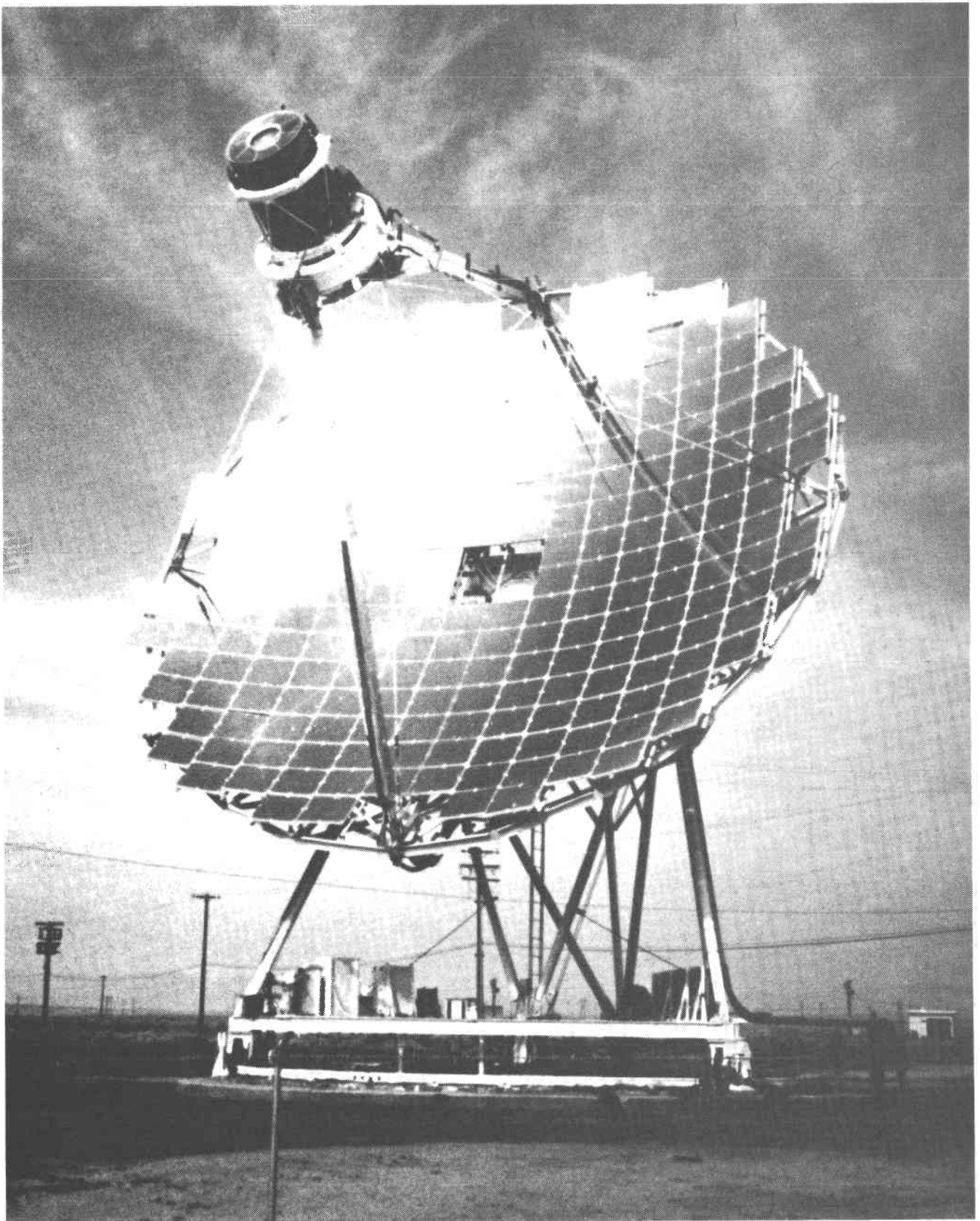
Figure 5-5. Power Conversion Assembly On-Sun Test at Edwards AFB, California
