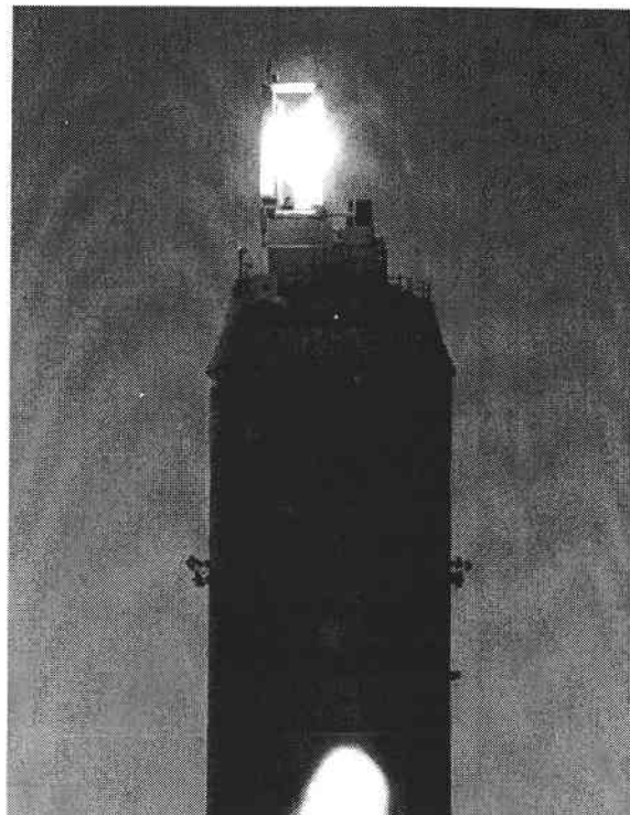
Figure 2. Boeing/Rocketdyne advanced panel undergoing high-flux testing at the NSTTF.
