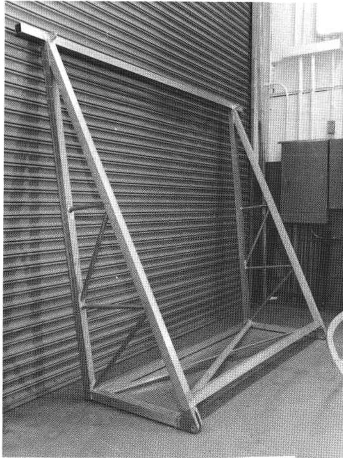
Figure 31. Wedge pivot structure of heliostat assembly.
