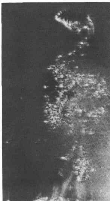
Fig. 3. Natural convection around a falling crystal revealed by examination in a Schlieren optical system.
