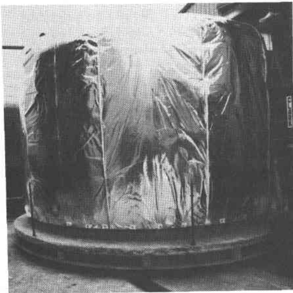
Fig. 2. Epoxy fiberglass inner dewar shell with 100 layers superinsulation.
