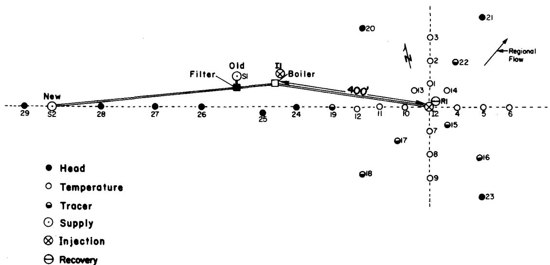
Fig. 2. Top view of the complete well field that has been constructed at the Mobile site. Water is obtained from the new supply well, heated by the boiler and injected into well I2. Water recovered from I2 after storage is injected back into S2 for later use.
