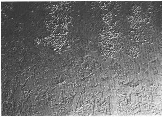
Figure 4.13 Top: Ni-Cr Powder Melt for Hard Facing Alloy on A2 Tool Steel; Bottom: Polished Cross Section Showing Alloy on Top and Steel on Bottom (1000X), Near Edge of Melt Zone
