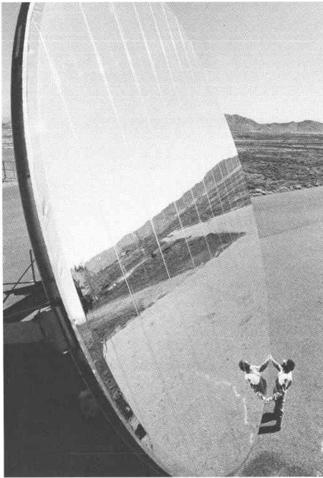
Figure 2.3 Prototype Stretched-Membrane Mirror Module Built by SKI
