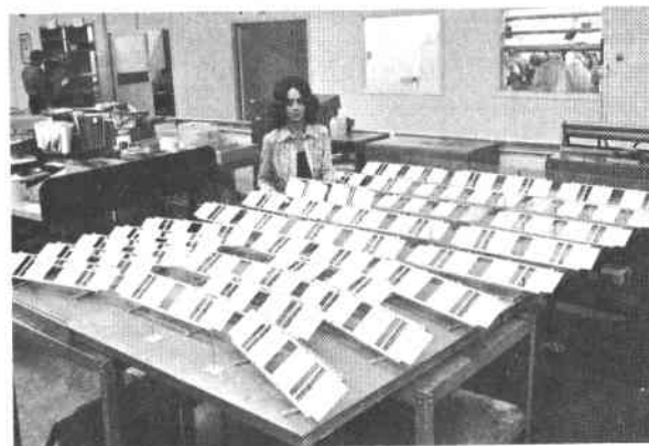
Figure 123. 1/30 Scale Model of Partial Heliostat Field Segments
