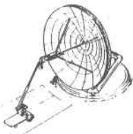
Figure 68. Proposed Engineering Experiment No. 1 — Phase I 1-MW e System Concept (Category C - Point-Focusing, Distributed Collector, Energy Conversion at the Collector)
