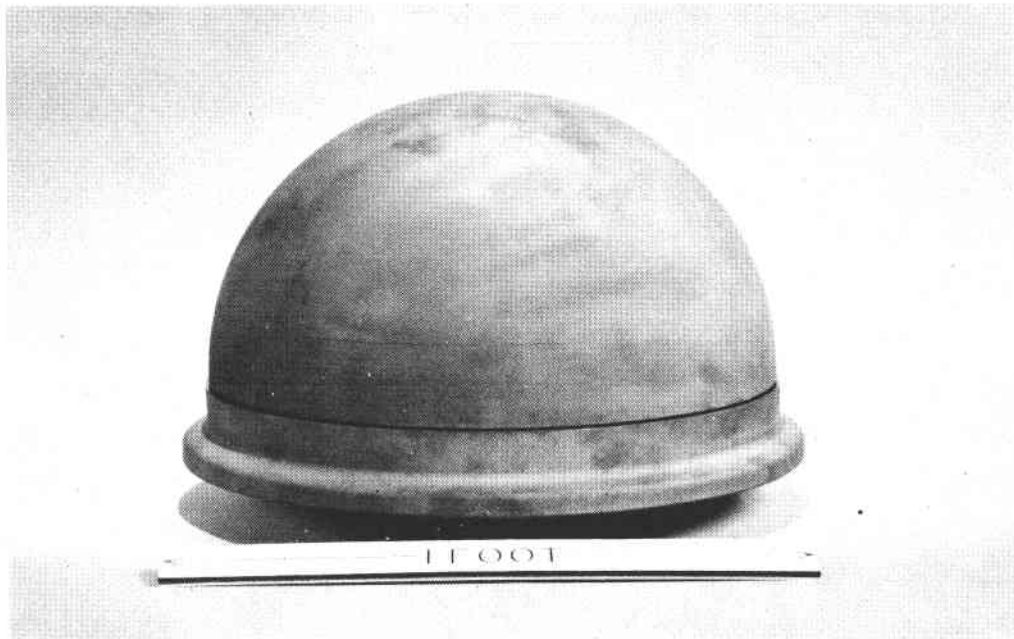
Figure 41. NC-430 silicon carbide hemispherical dome and insulating ring seal unit.
