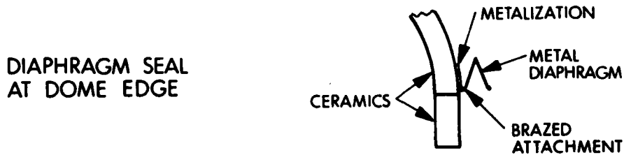
Figure 24. Brazed ceramic/metal seal concept.
