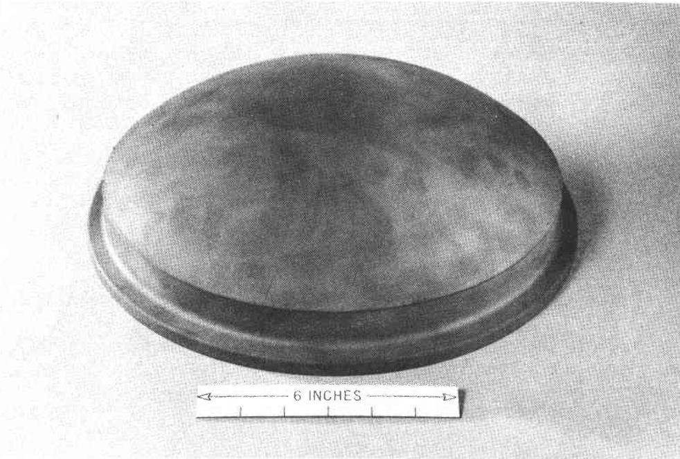
Figure 42. NC-430 silicon carbide shallow dome and insulating ring seal unit.
