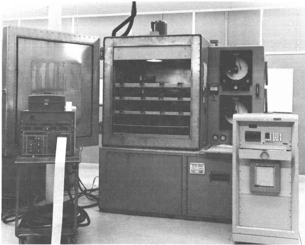
Figure 21. Environmental Control Chamber, Control Unit and Data Logger
