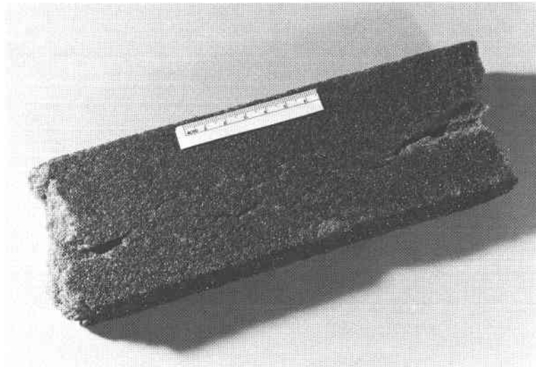
Figure 13. Degraded Cellular Glass
