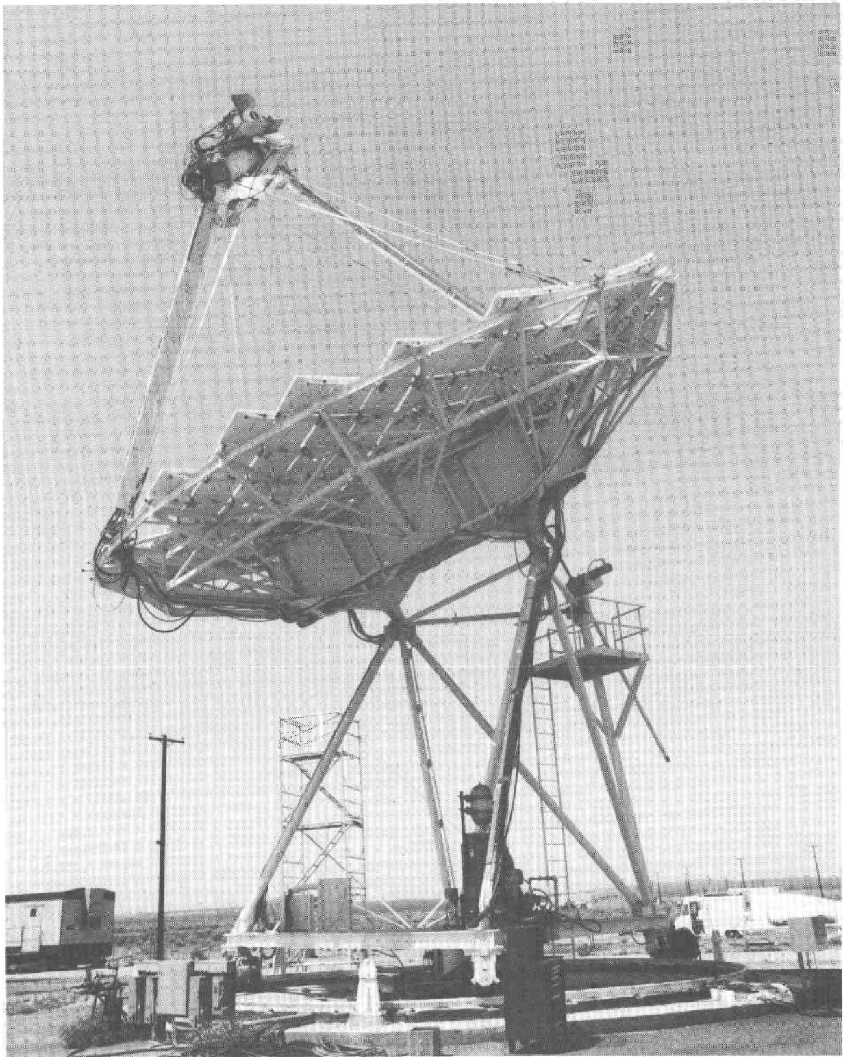
Figure 4. Stirling Engine Testing at the Parabolic Dish Test Site
