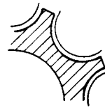
B) SALT CONTRACTION UPON FREEZING CAUSES A GAP TO FORM BETWEEN SALT AND CONTOUR SURFACE.
