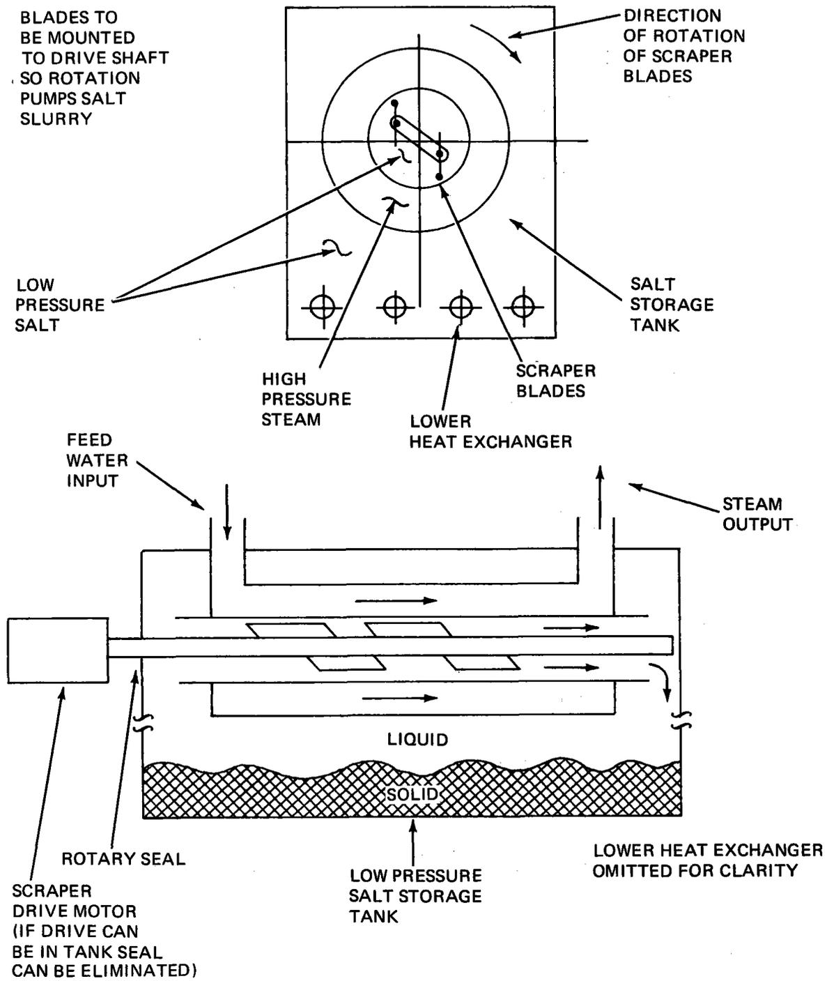
Figure 4-9 Proposed Heat Exchanger Internal Tube Scraper
