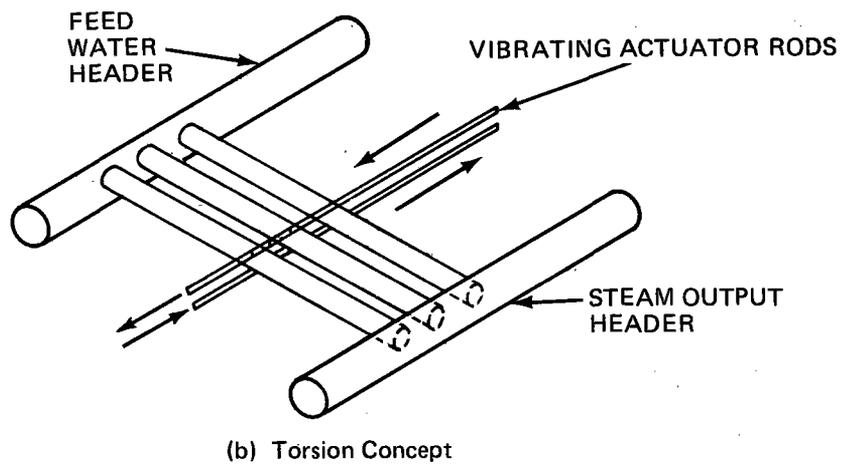
Figure 4-13 Proposed Vibrating Heat Exchanger Concepts
