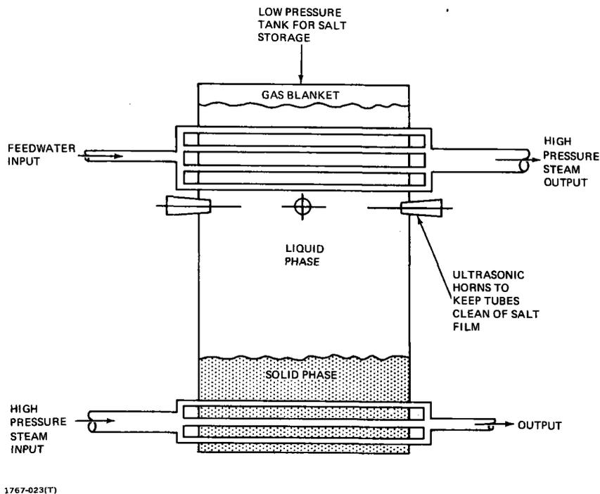
**Figure 4-14 Proposed Heat Exchanger Utilizing Ultrasonics to Keep Tubes from Getting Salt Buildup**
