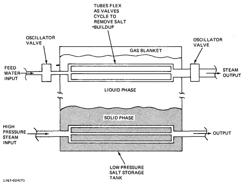
Figure 4-15 Proposed Heat Exchanger Tube Flexing thru Pressure Pulsing by Throttling Valving
