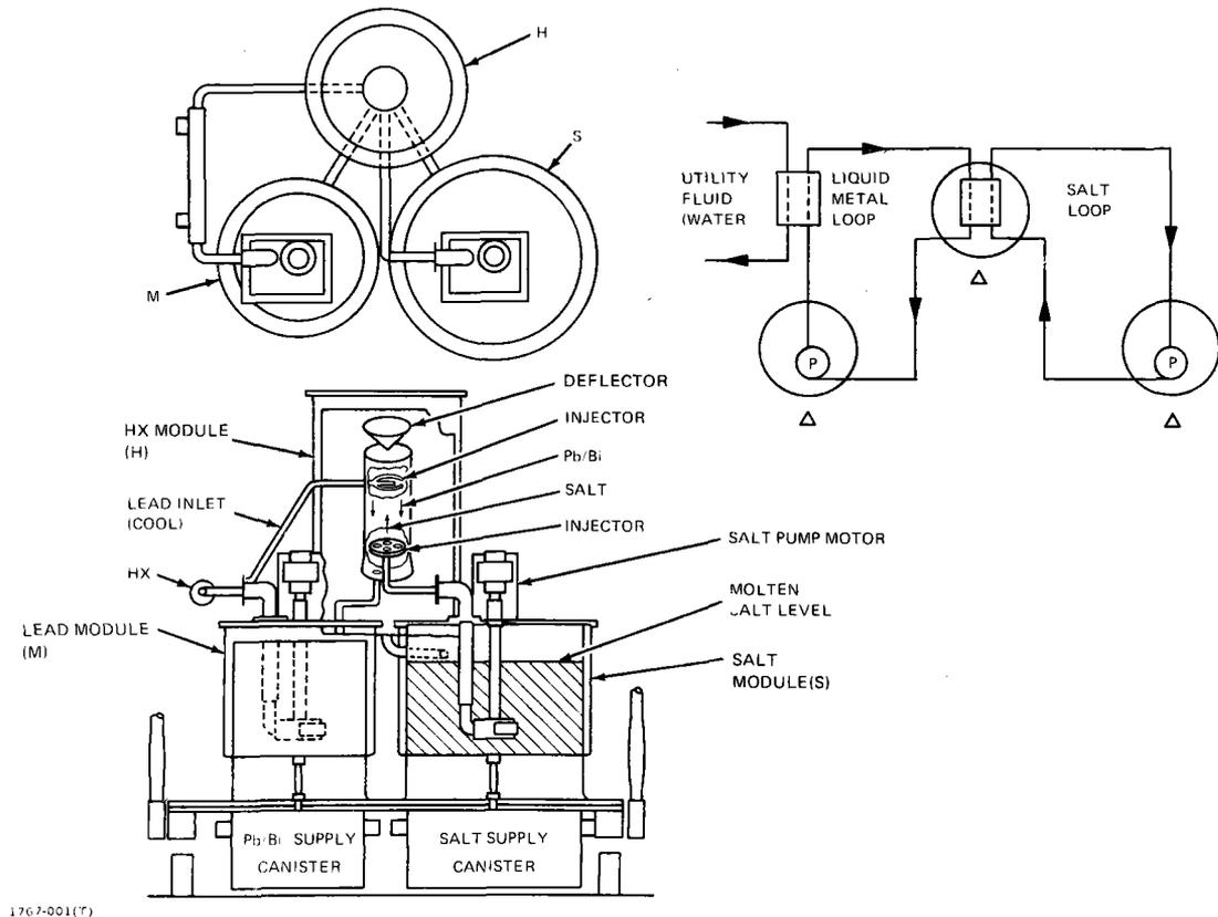
Figure 2-1 Direct Contact HX Concept
