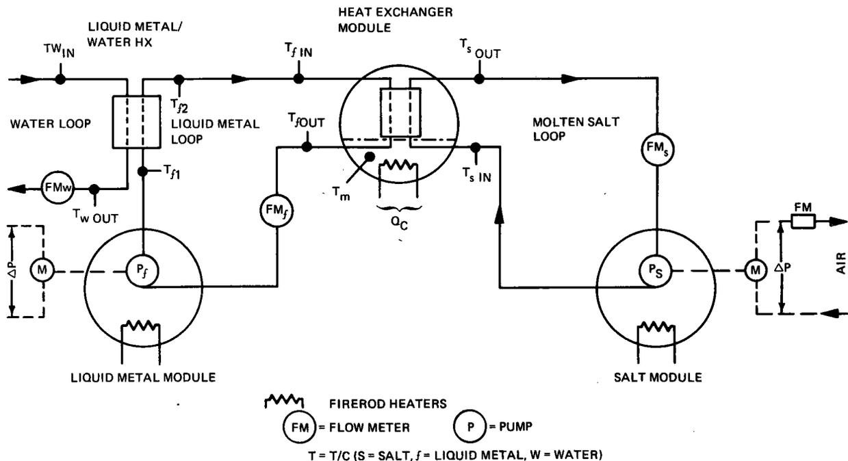
**Figure 6-1 Demonstration Active TES System Schematic**
