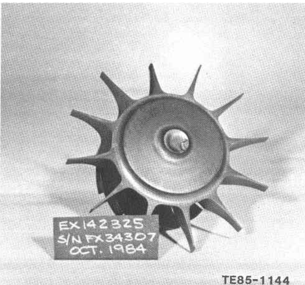
Figure 75. Fracture on rotor S/N FX34307 (first assembly, modified attachment design).
