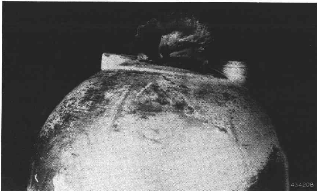
Figure 5. Carbon accumulation on S/N2, TD22 main combustor nozzle.
