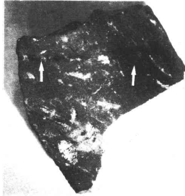
Figure 61. Gasifier scroll shroud pieces showing long curved rub marks left by the rotor airfoils.
