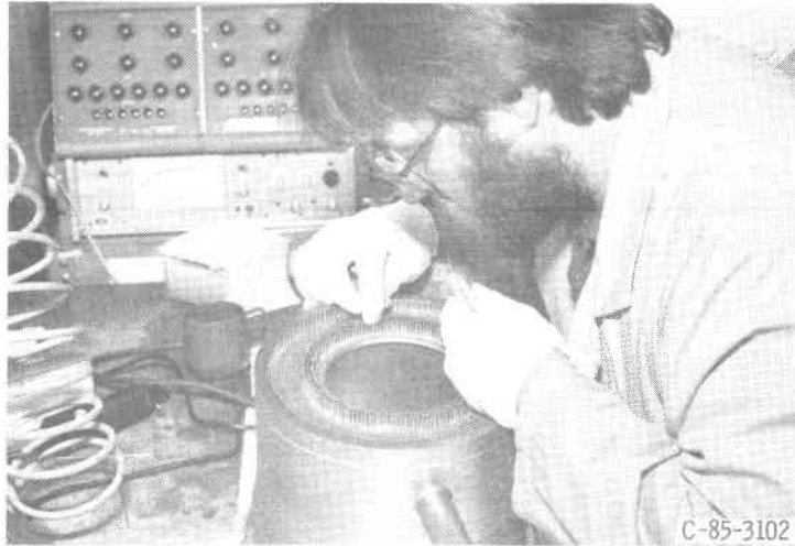
Figure 12. - Assembly of SPDE molten salt heat exchanger.
