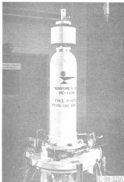
Figure 19. - 1 kW RE-1000 free-piston Stirling engine with dynamic absorber balancing unit.
