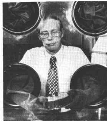
Dr. Paul Nelson, Argonne National Laboratory, holds the newly developed lithium/sulfur battery developed by Argonne engineers. An enclosure called a "glove box" filled with an inert atmosphere to prevent oxidation is used to assemble and test the cells.
