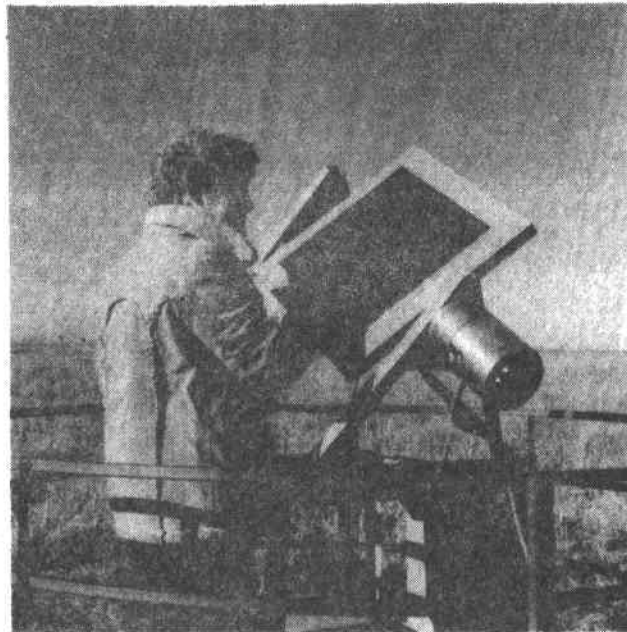
FIGURE 8-7. HELIOSTAT SIMULATOR IN PLACE AT THE PROPOSED SITE
