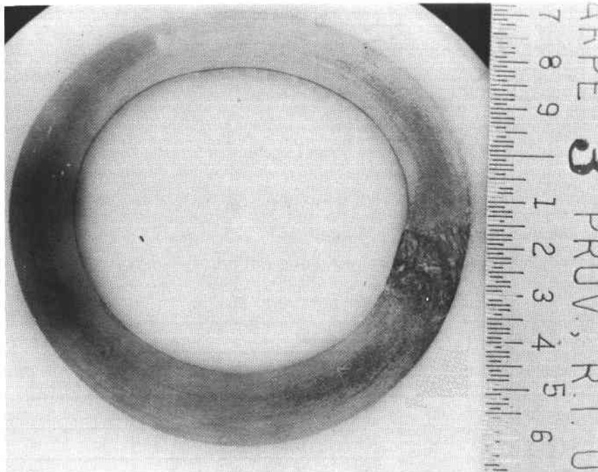
Figure 7-13. Wall Bending Effects
