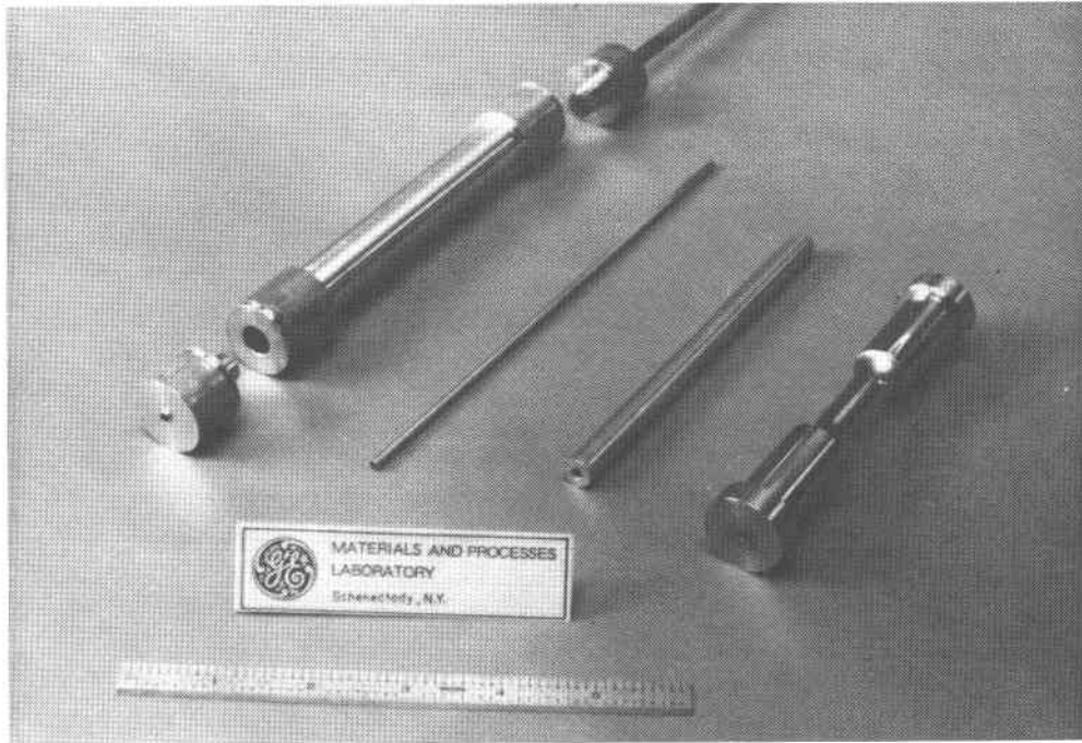
Figure 33. MZC Copper Composite LCF Specimen with IN-617 Outer Skin and IN-718 Inner Tube
