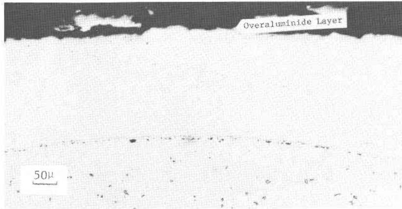
FIGURE 9. LEADING EDGE, S-57 CLADDING + OVERALUMINIDE AS POLISHED
